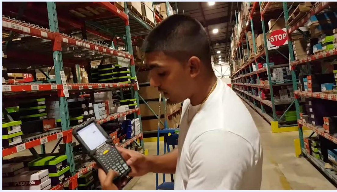
Close-up of the RF gun screen showing the assigned picking location and task details, with warehouse shelves in the background.
