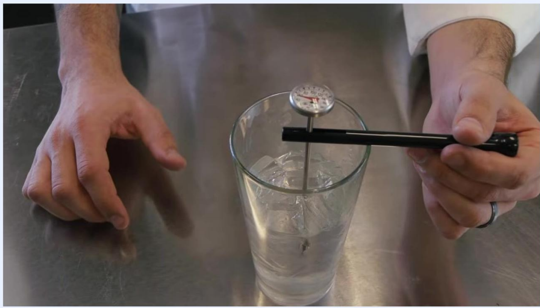
Close-up of a hand pointing to the calibration nut on the back of the thermometer dial, thermometer above a glass of ice water
