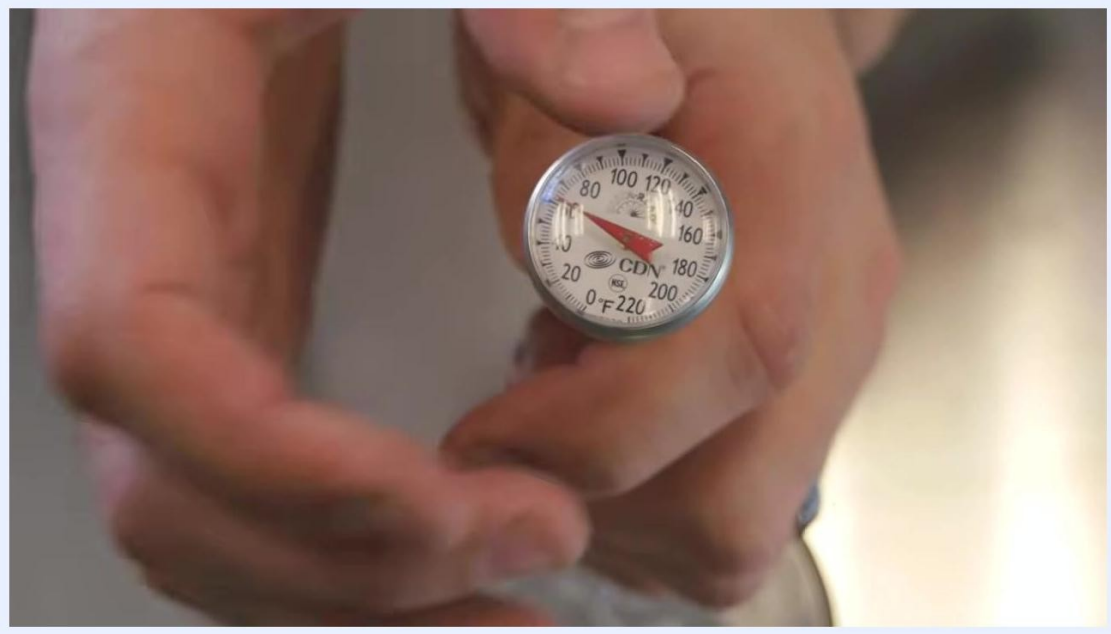
Hands holding the dial probe thermometer, showing the needle at the correct calibration point
