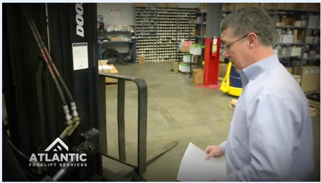
Inspector visually checking the overhead guard and lights above the operator's seat on the forklift.
