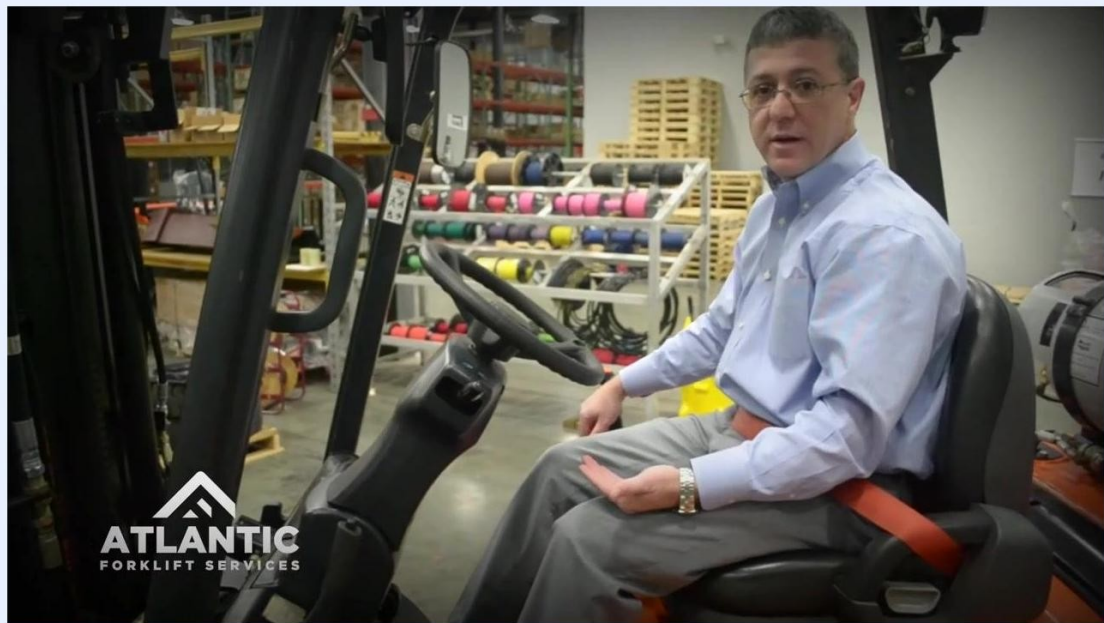
Operator seated in the forklift, demonstrating hydraulic control operation, with visible steering wheel, levers, and seat belt fastened.
