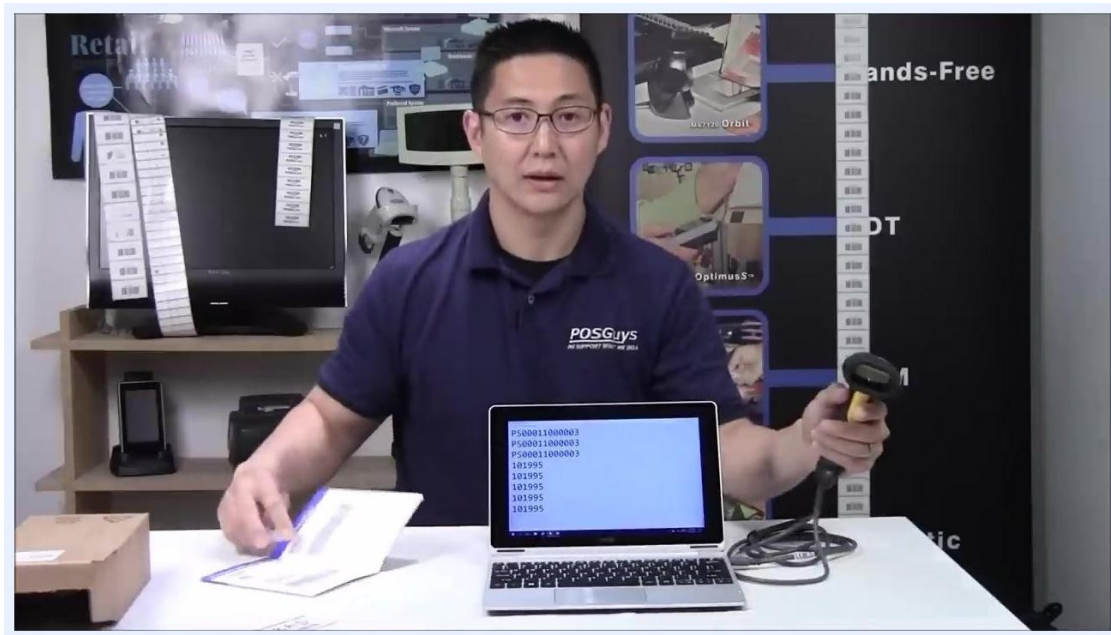
A person demonstrates scanning a barcode with the scanner, while the laptop screen shows barcode data in a text editor and the quick start guide is open on the table.
