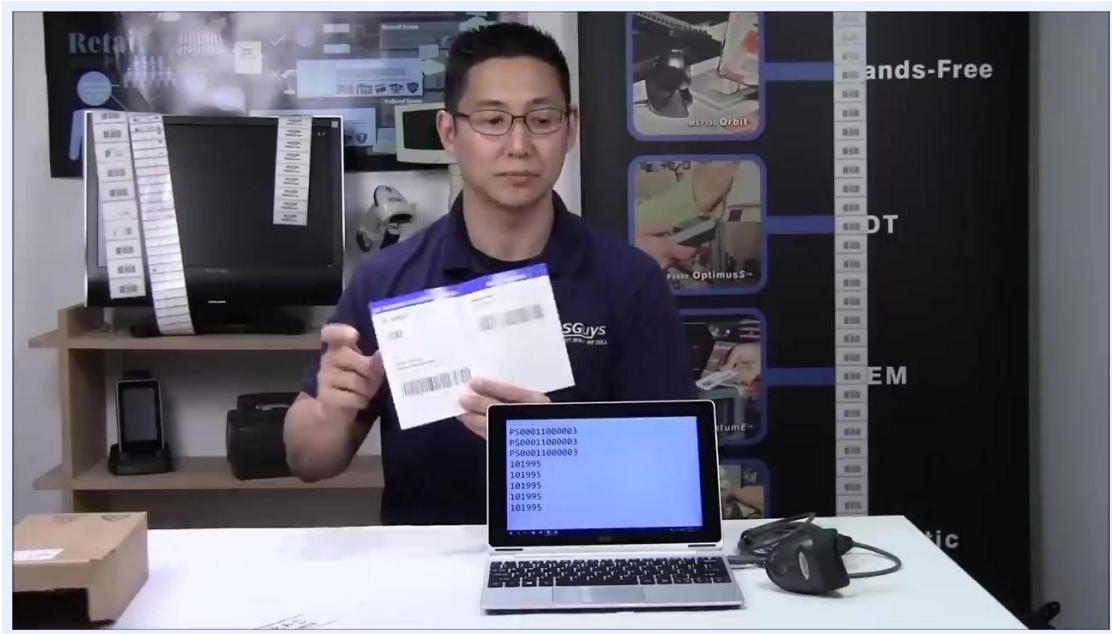
A person holding the quick start guide open to display configuration barcodes, with the laptop showing scanned data in Notepad.
