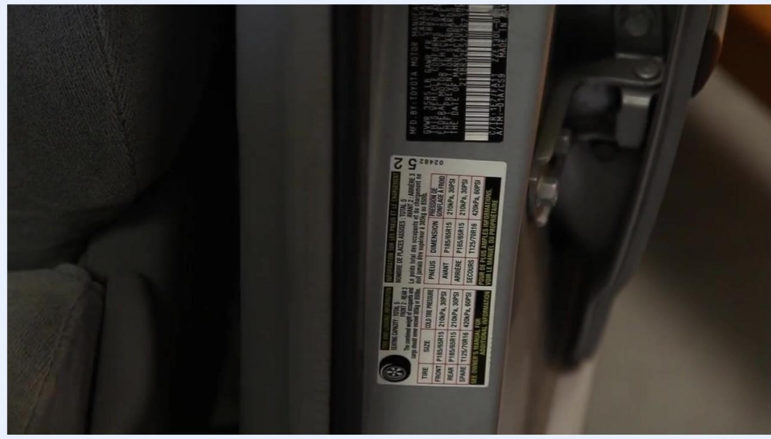
A close-up of the tire information sticker on the driver's side door jamb. A finger points to the sticker, which lists recommended tire pressures and tire sizes.
