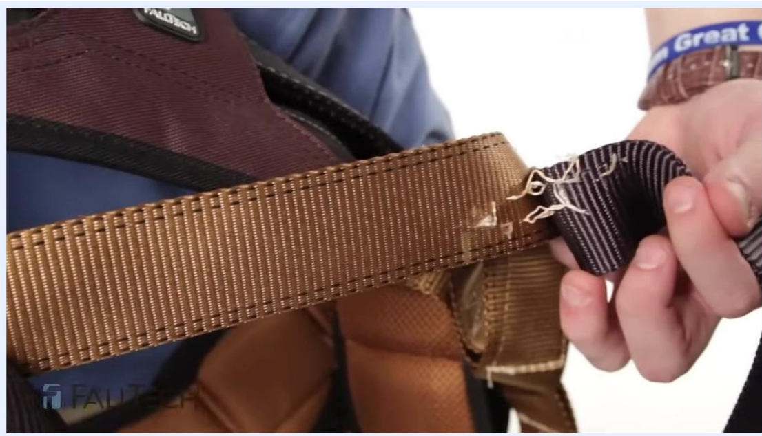
Close-up of a hand holding a brown sub-pelvic strap on a harness, showing visible fraying and damage to the webbing and stitching
