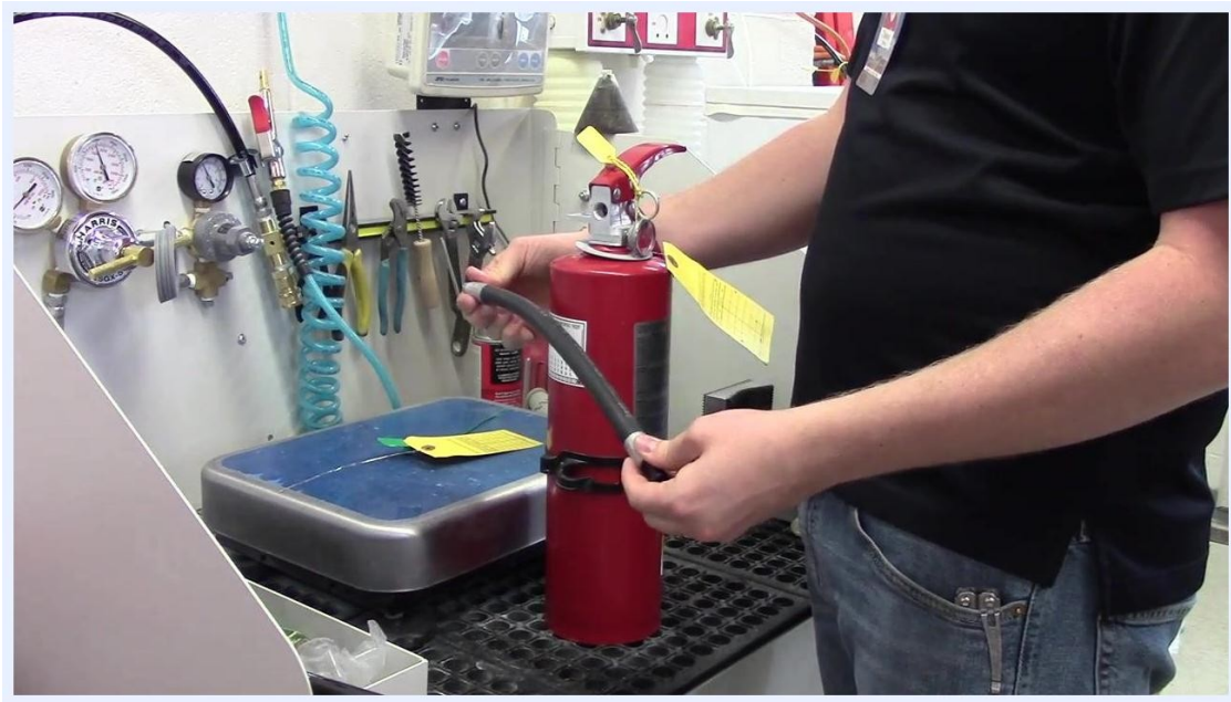
A person holding the detached hose, inspecting it for blockages and deformities.
