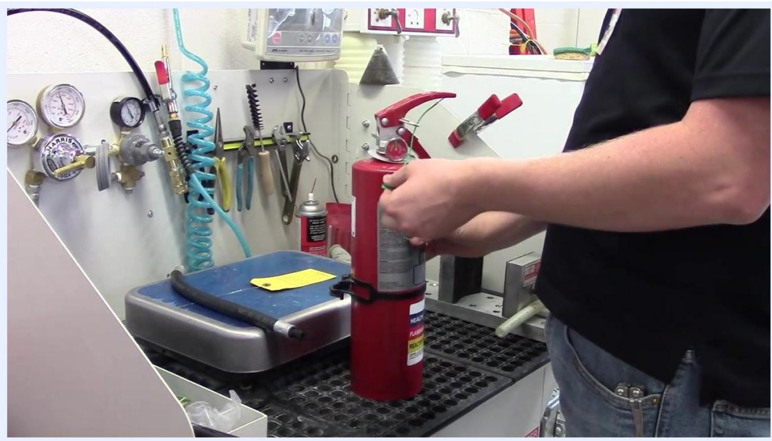
A person threading and securing a green zip tie through the pin and under the handle of the fire extinguisher.
