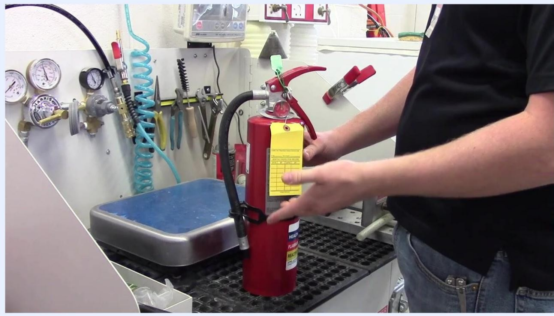
A person creasing and positioning the inspection tag so it sits flat and visible on the front of the fire extinguisher.
