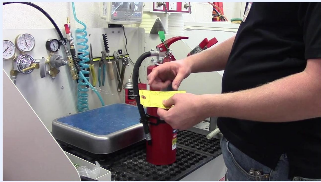
A person holding a yellow inspection tag next to a fire extinguisher, preparing to punch the tag. The workbench has various tools, gauges, and hoses visible.
