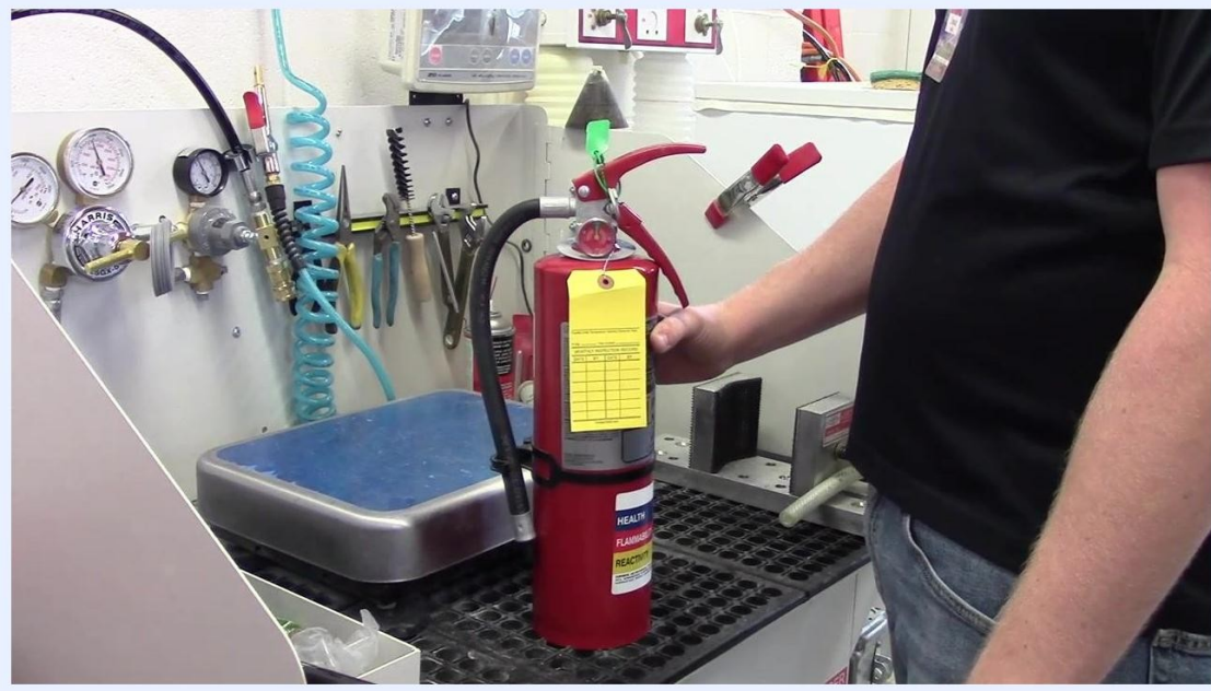
A completed fire extinguisher with a properly attached and positioned yellow inspection tag, ready for service. The workbench and tools are visible in the background.
