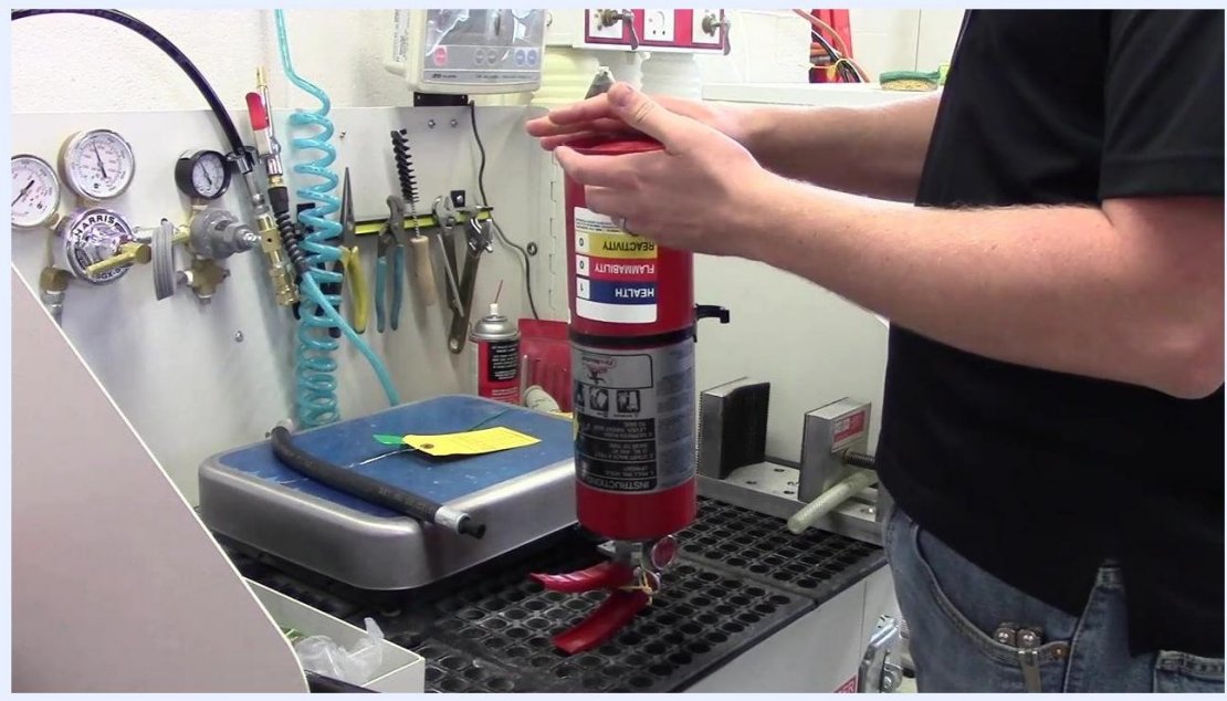
A person holding the fire extinguisher upside down, performing the fluffing procedure to loosen the internal agent.
