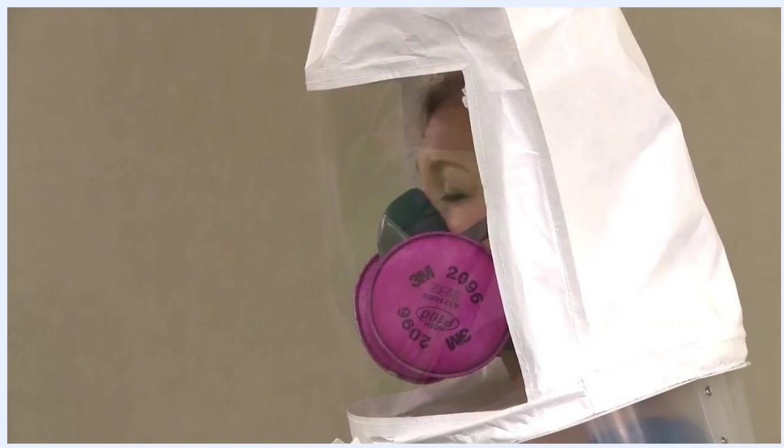
Close-up of a test subject wearing a respirator and fit test hood, indicating a successful fit.
