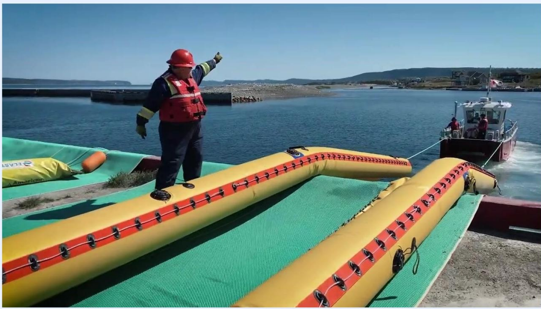
A Coast Guard worker in a red helmet and life vest standing on the containment boom, directing operations as a vessel tows the boom into the water.
