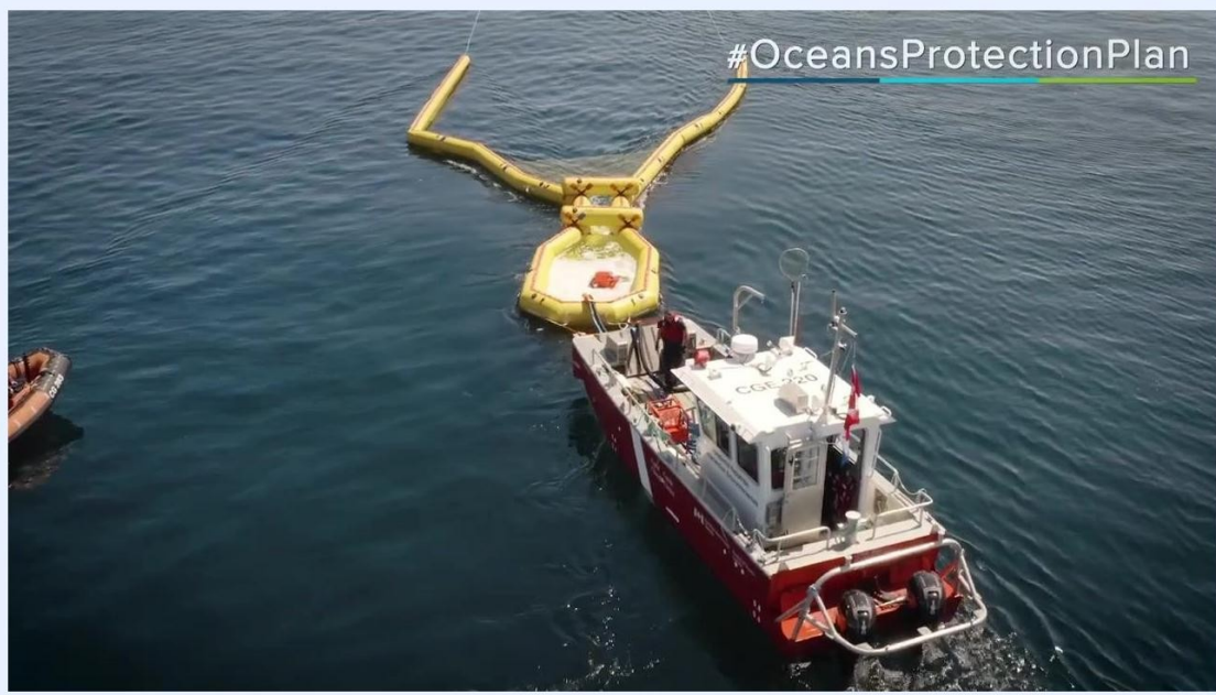
Aerial view of a Coast Guard vessel positioned at the apex of a yellow containment boom, with a skimmer device deployed inside the boom to recover oil.
