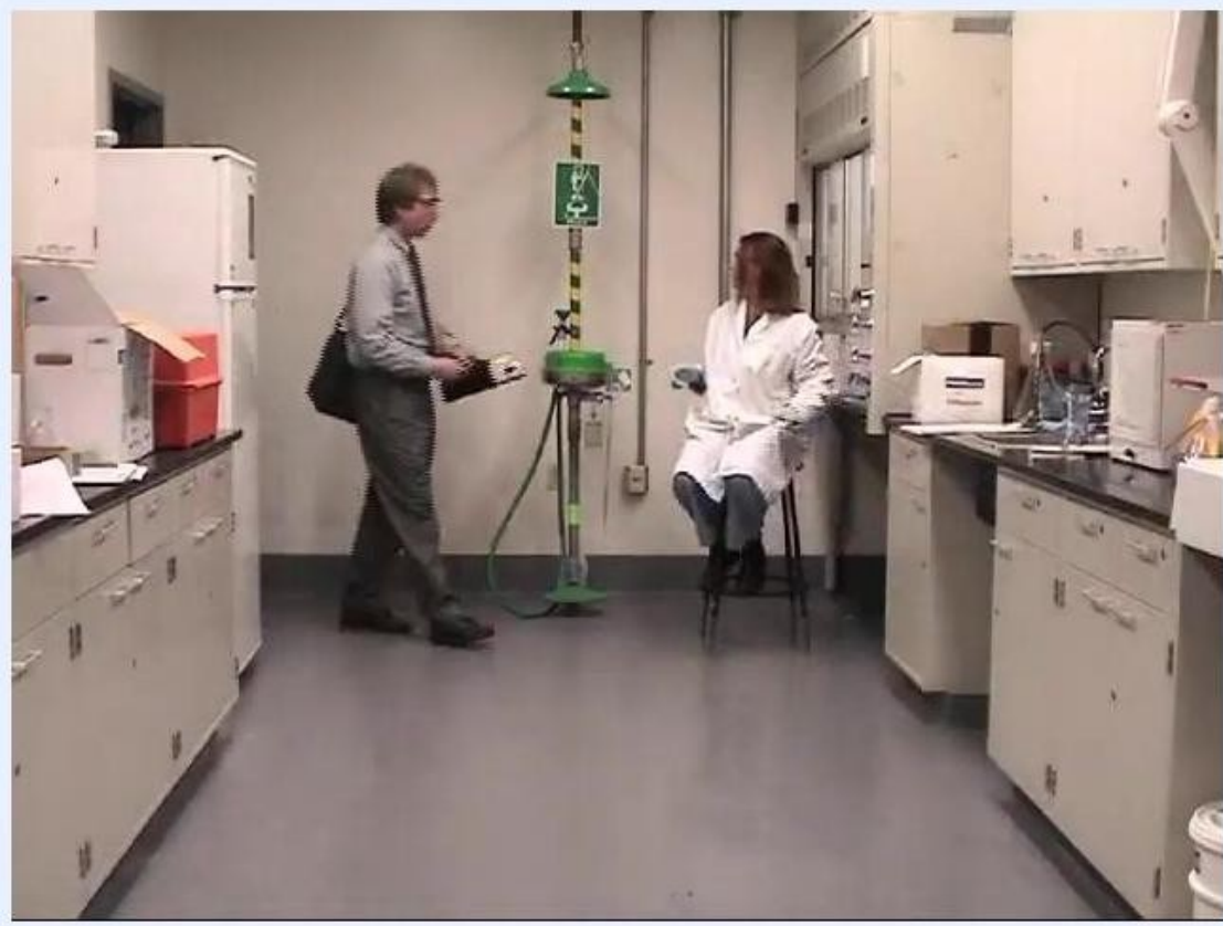
An EH&S staff member and a laboratory worker use a mercury vapor detector to check the floor and cabinet area for contamination.
