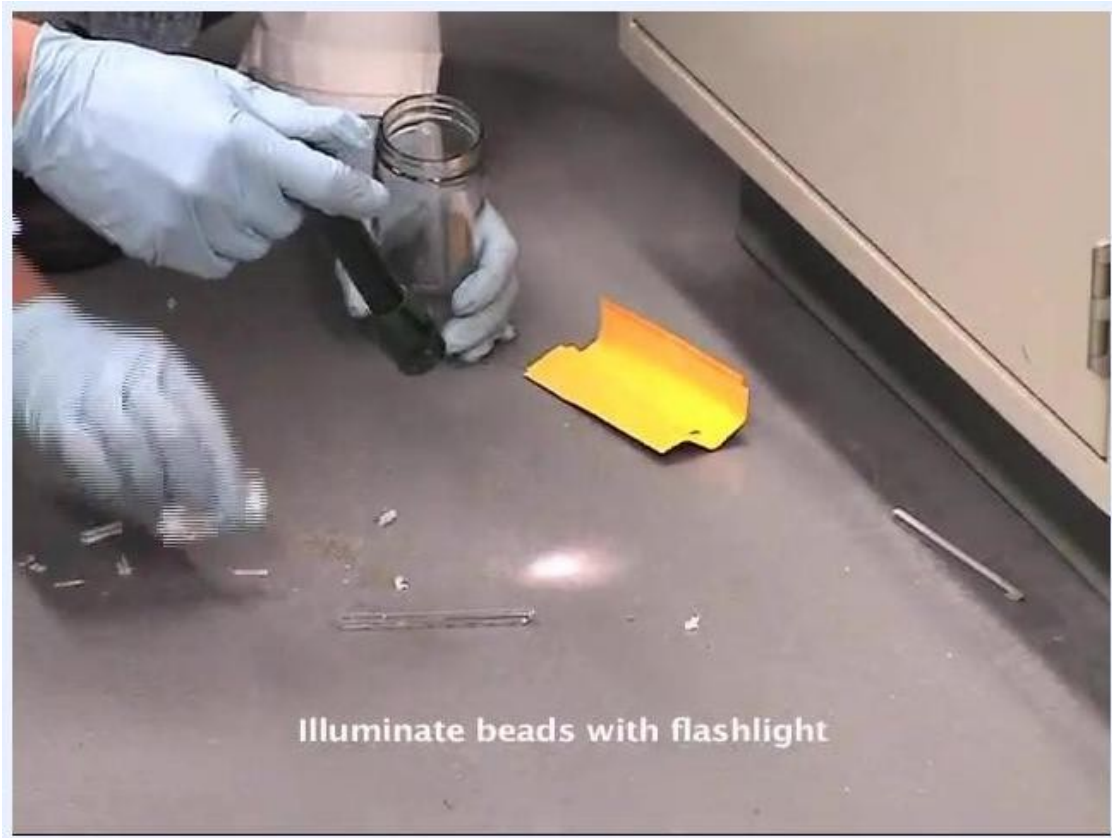
A gloved worker illuminates the floor with a flashlight to make small mercury beads visible.
