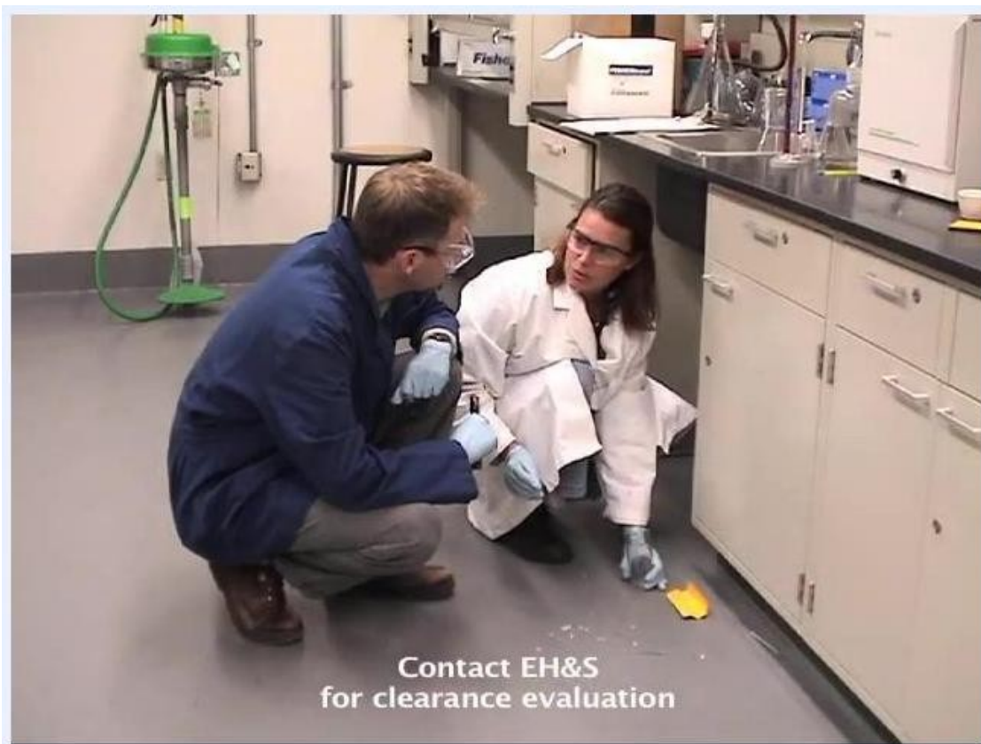
A gloved worker uses tape to dab the floor and collect small mercury beads.
