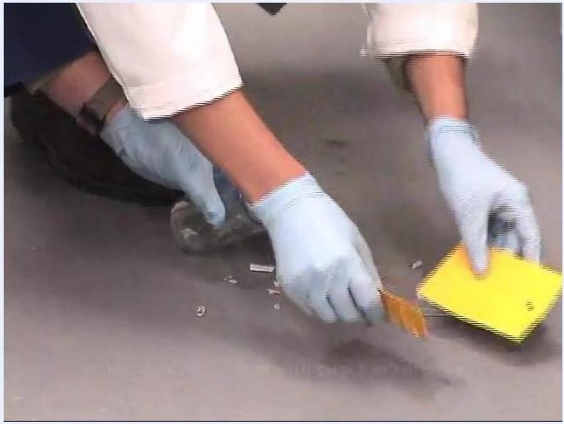
A gloved worker uses two pieces of paper to scoop up mercury beads and broken glass, placing them into a glass jar.
