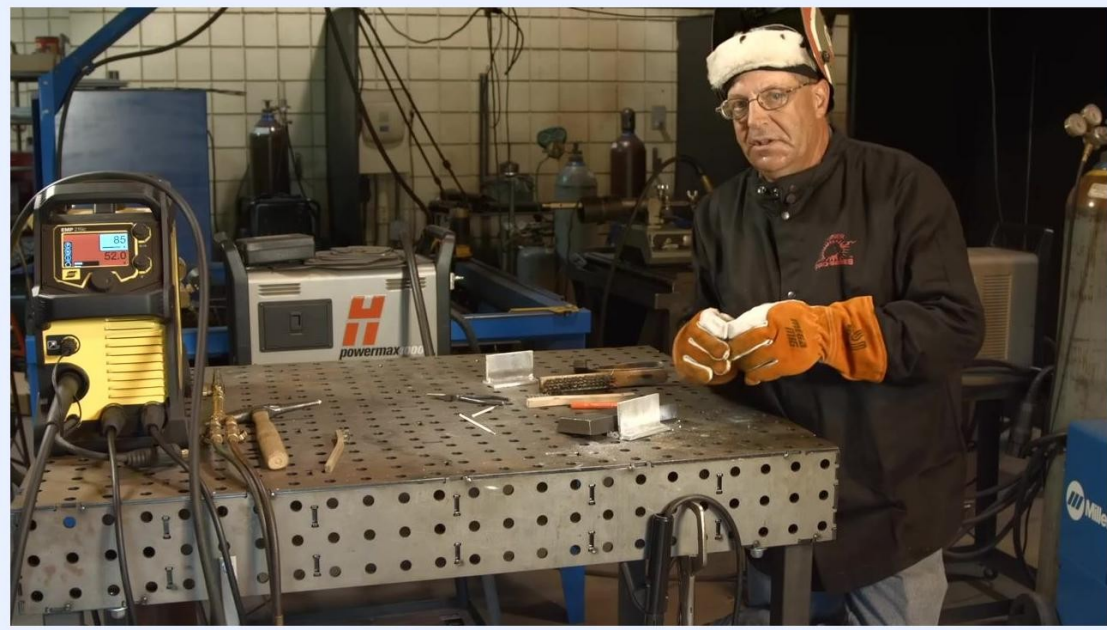
Using a wire brush or chipping hammer to clean the weld, gloves and helmet on, with the welding machine and tools visible.
