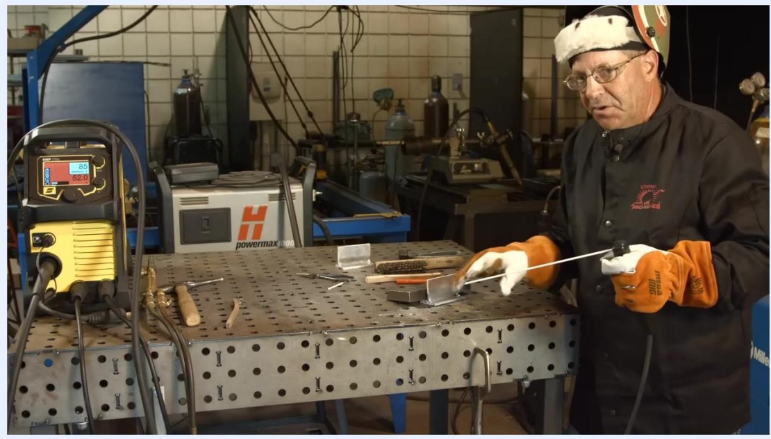
Gesturing toward the welded joint with the electrode while discussing grinding and multiple passes, with the welding machine and tools visible.
