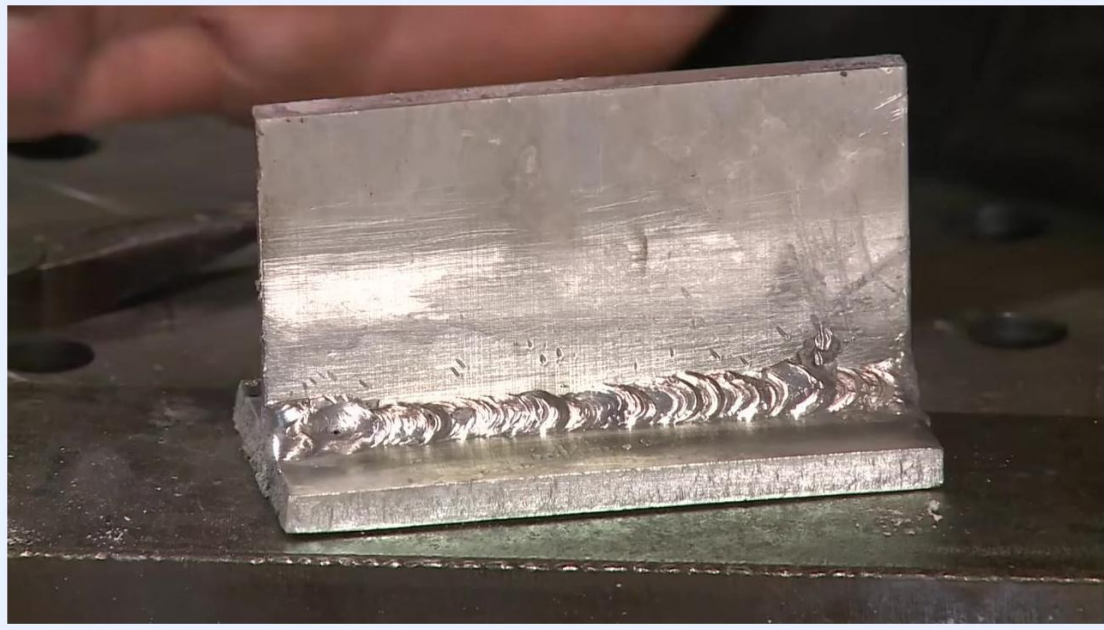
Aluminum weld joint on the workbench, rod pointing at the weld, ready for further cleaning or blending.
