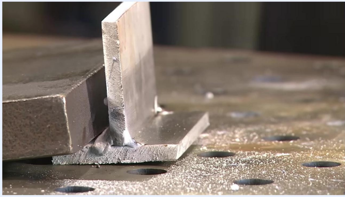
The welded joint on the perforated table, showing the results of the previous pass and some spatter, with no hands or tools in frame.
