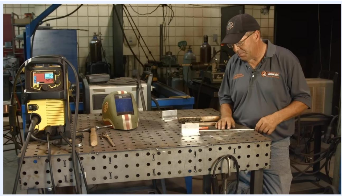
A welding table holds an ESAB EMP 210 welder displaying 85 amps and 52.0 volts, along with a welding helmet, wire brush, marker, and aluminum workpieces staged for the preheating process.
