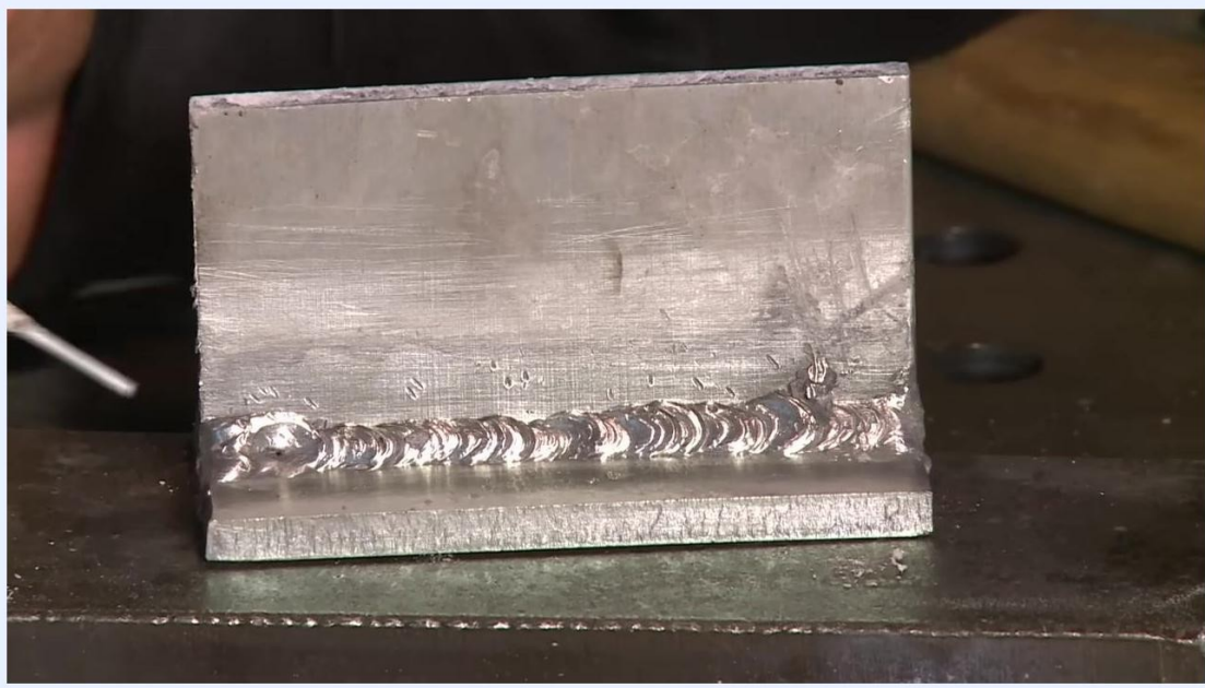
Aluminum weld bead with a hand and tool, illustrating finishing preferences.
