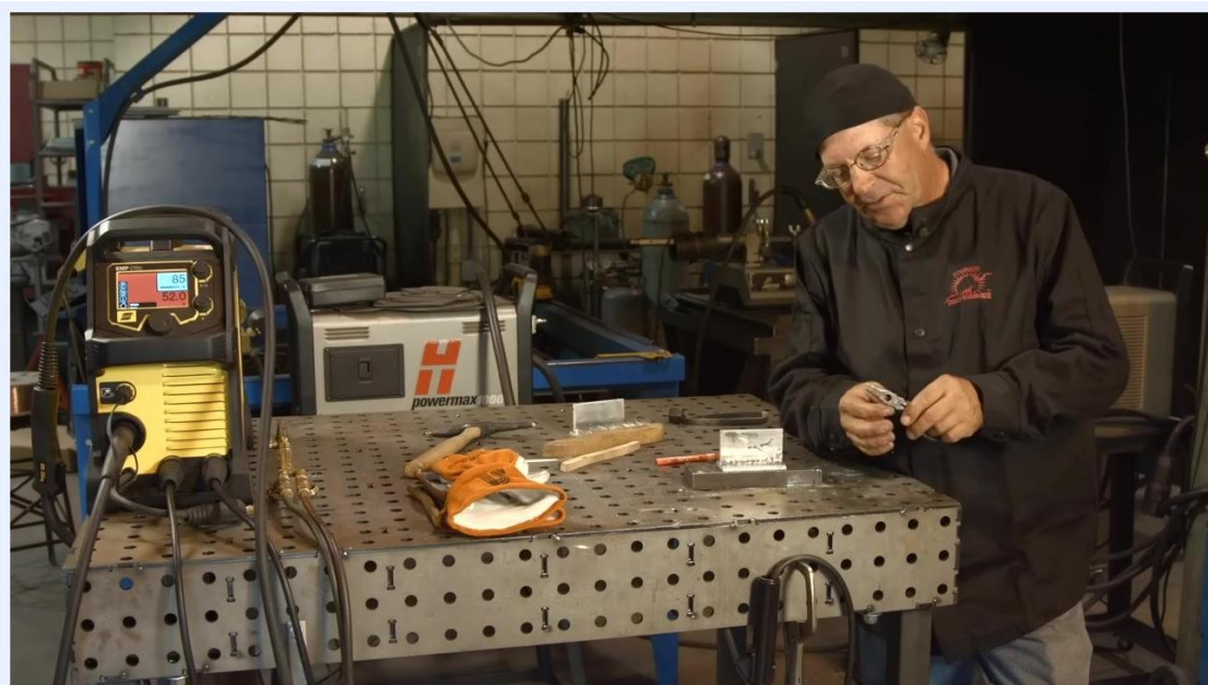
Using pliers to remove residue from the electrode or workpiece, with a close-up of hands and tools and the cleaned joint on the table.
