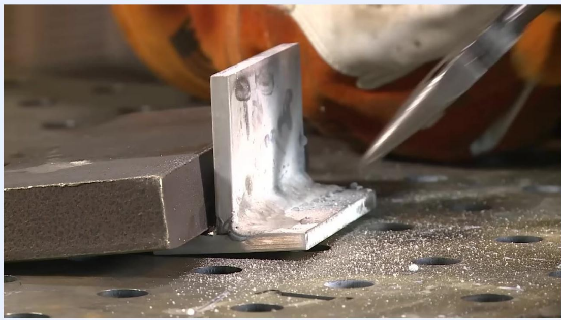
Close-up of the welded joint showing visible slag and spatter, with a gloved hand holding a tool near the weld and debris on the table surface.
