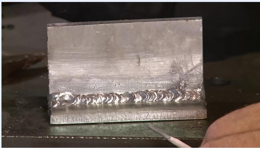
Extreme close-up of the weld crater and star hole, with a hand holding the workpiece for emphasis.
