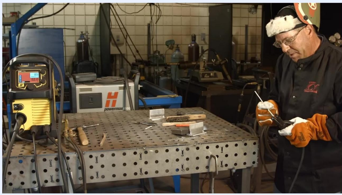
Preparing to weld with electrode and electrode holder in hand, the welding machine set to 85A/52.0V, and tools and metal pieces on the table.
