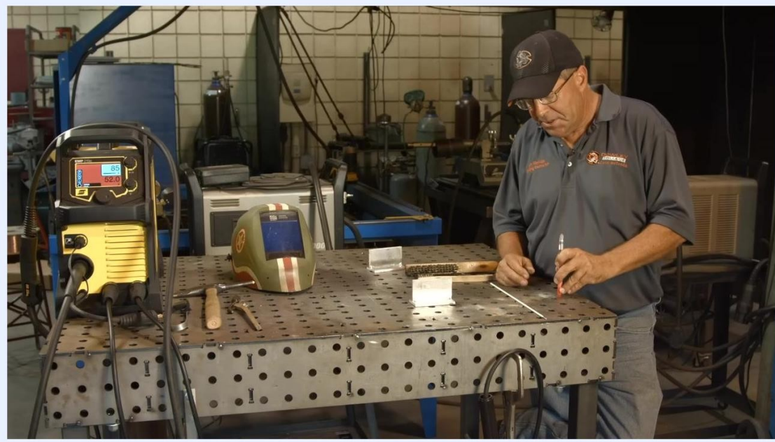
Marking the aluminum workpiece with a Tempilstik in preparation for preheating, with the full workbench setup visible.
