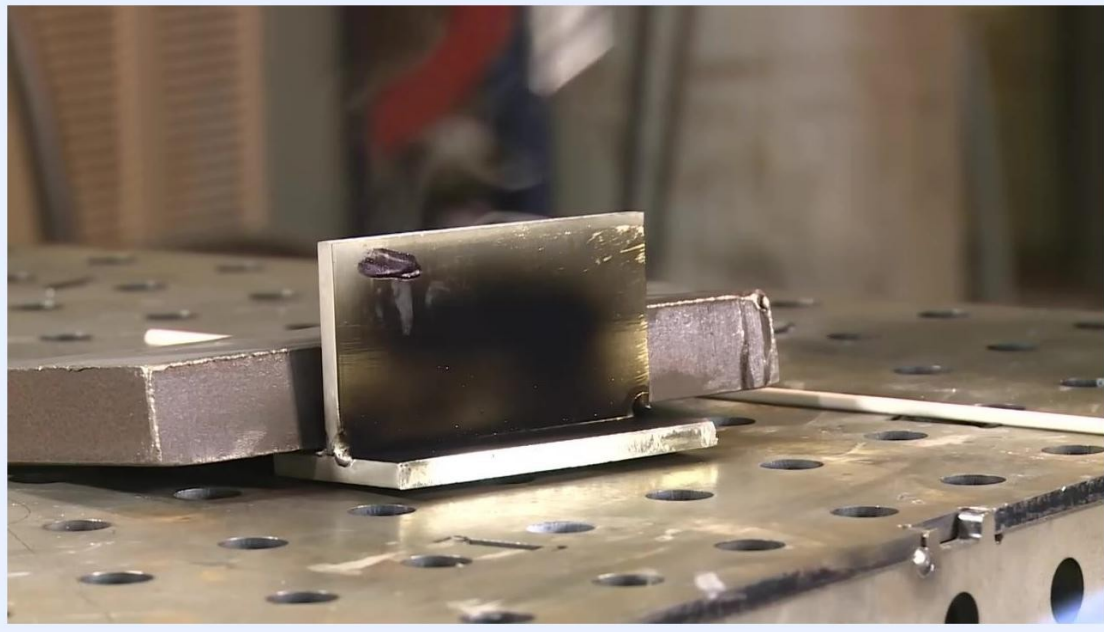
An oxy-acetylene torch flame applied to the aluminum workpiece, now cleaner with visible tack welds, sitting on a perforated welding table.
