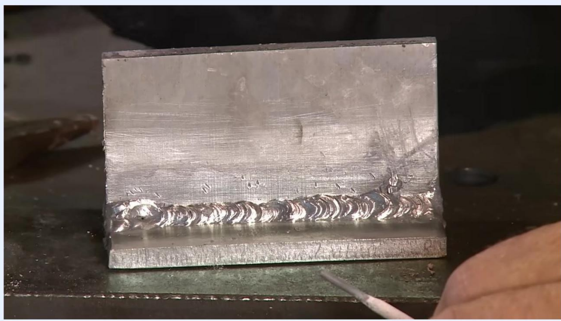
Aluminum weld joint with a crater at the termination point, a rod pointing to highlight the defect.
