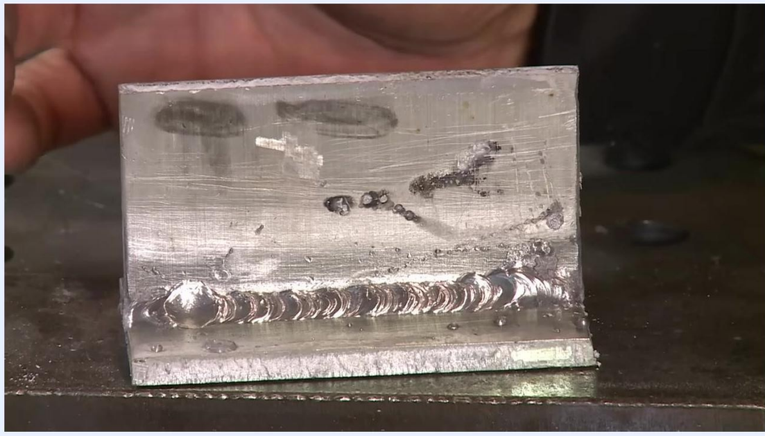
Opposite side of the aluminum weld showing an additional blob, with a hand pointing using a tool.
