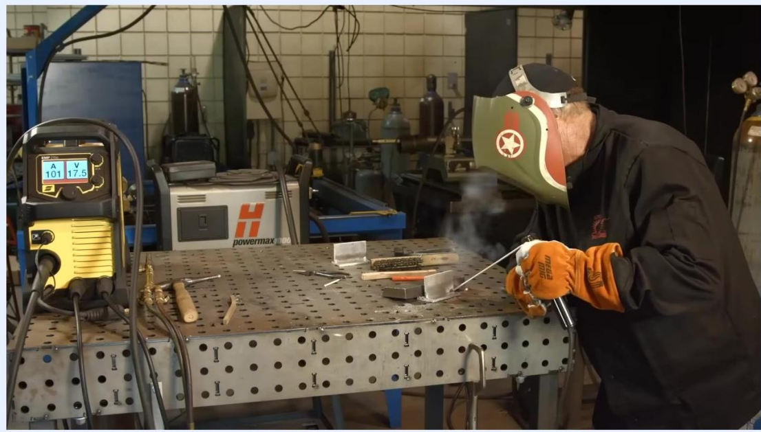
Actively welding with the helmet down and the arc visible; the welding machine display shows 101A/17.5V, with tools and materials on the table.
