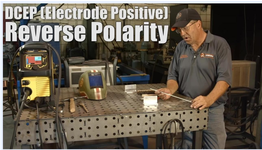
On-screen text reading "DCEP (Electrode Positive) Reverse Polarity" is displayed over the welding setup, with the ESAB EMP 210 machine, welding helmet, wire brush, and aluminum workpieces visible on the table.
