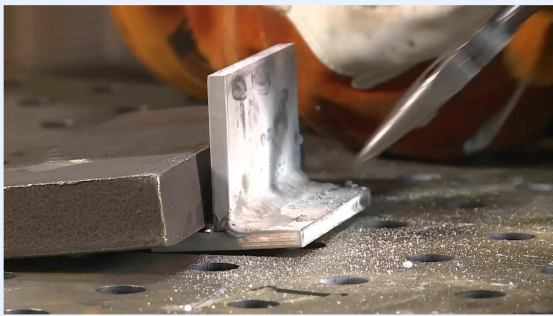
A gloved hand using pliers to remove spatter from the welded joint, with a close-up view of the weld and debris on the table.
