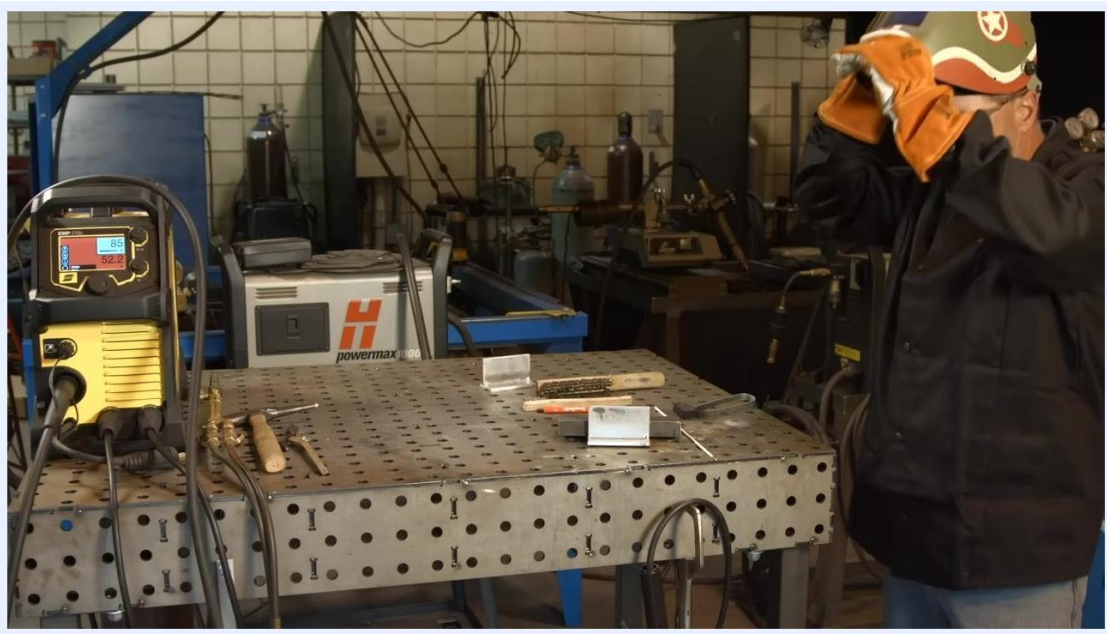
Putting on a welding helmet at the workbench, with the ESAB EMP 210 welder and various tools visible, ready for welding.
