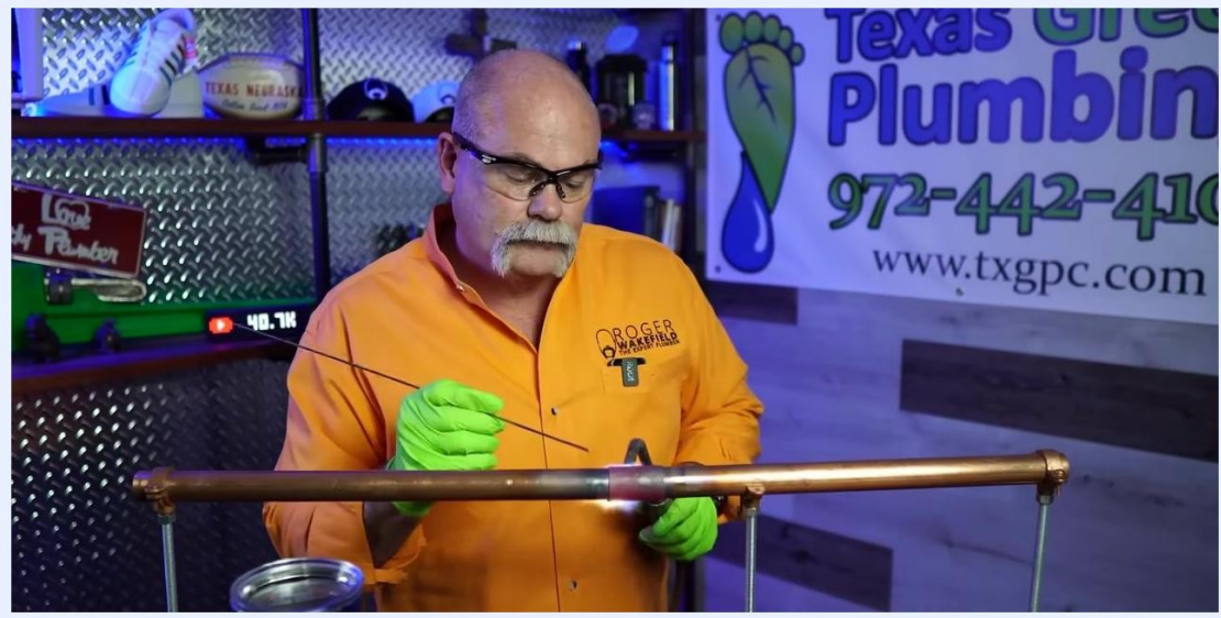
A person applies solder to a copper pipe joint while heating with a torch, ensuring a complete seal.
