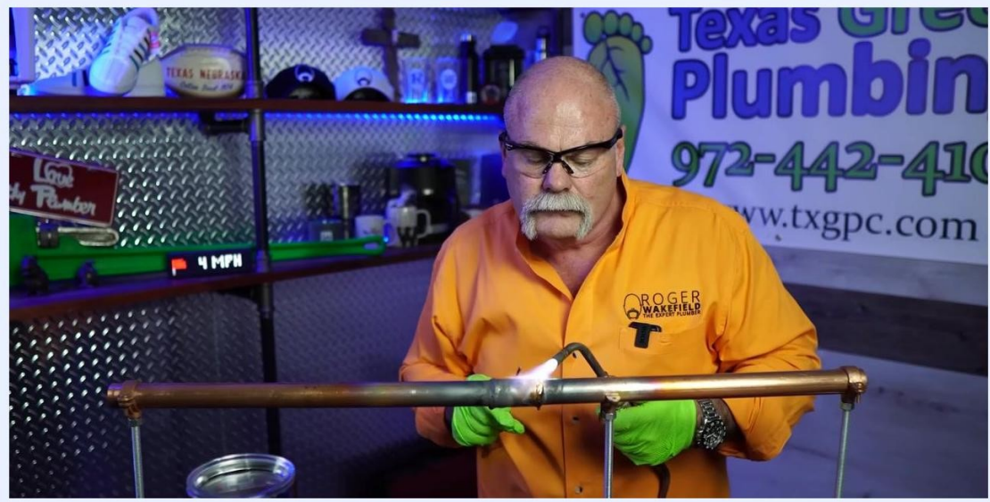
A person heats a copper pipe joint with a torch while holding solder wire above the joint, with a Texas Green Plumbing sign visible in the background.
