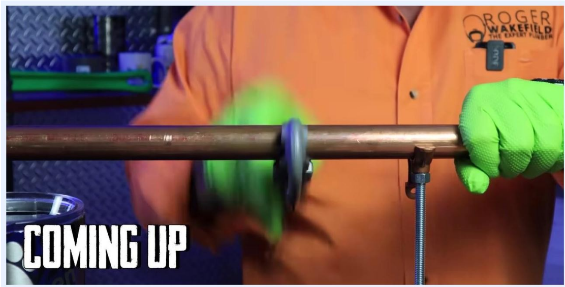
A person wearing an orange shirt and green gloves uses a pipe cleaning tool on a horizontally mounted copper pipe in a plumbing workshop with signage and tools in the background.
