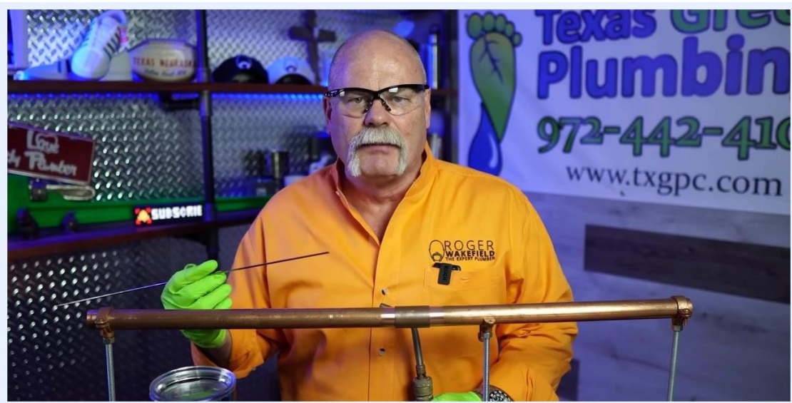
A person holds a thin solder wire near a copper pipe joint while the other hand remains near the torch.
