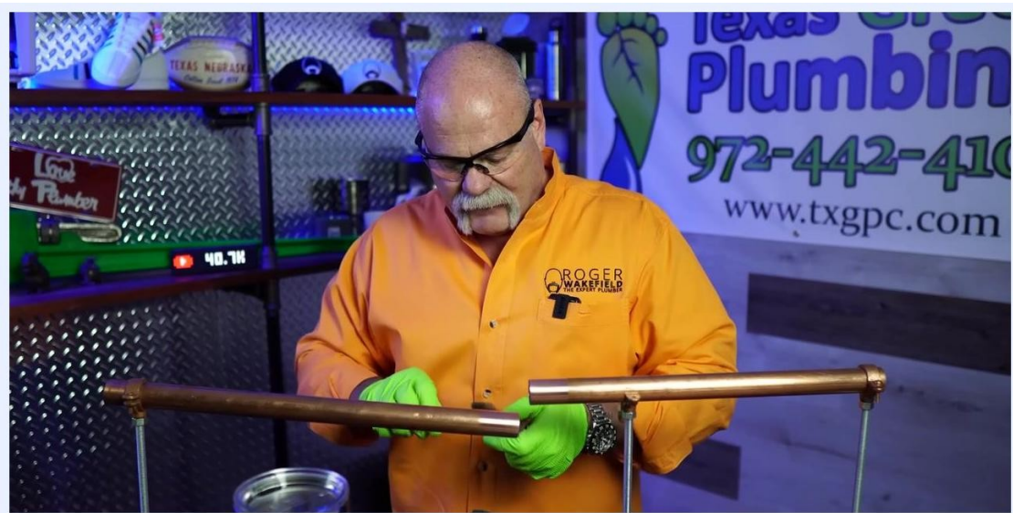
A person uses a green abrasive pad to clean a copper pipe in a plumbing workshop.
