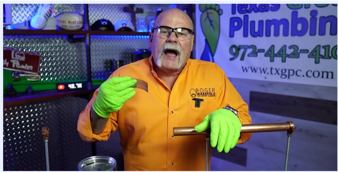
A person continues cleaning a copper pipe with an abrasive cloth in a plumbing workshop.
