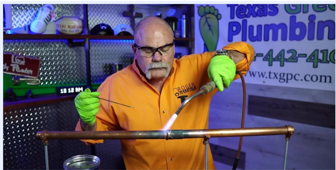
A person applies torch flame to a copper pipe joint while holding solder wire ready in a workshop with branded signage.
