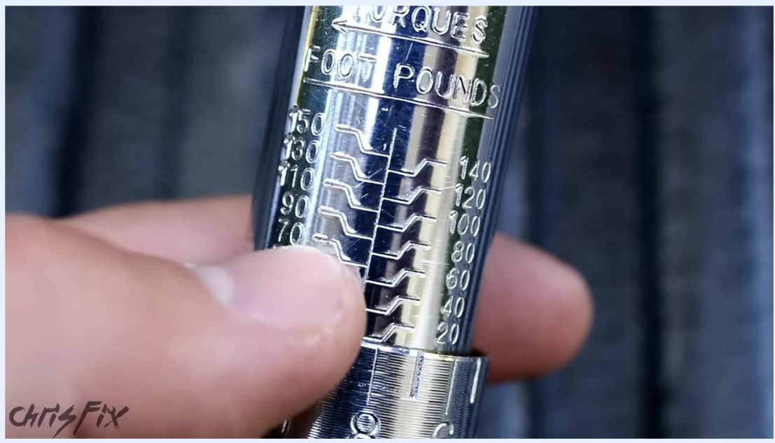
Close-up of a torque wrench scale with a finger pointing at the 100 foot-pounds mark
