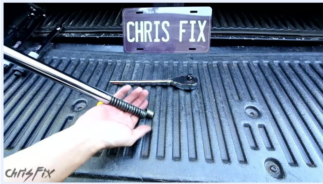
A disassembled torque wrench showing the internal spring and ratchet mechanism, with a "CHRIS FIX" plate in the background
