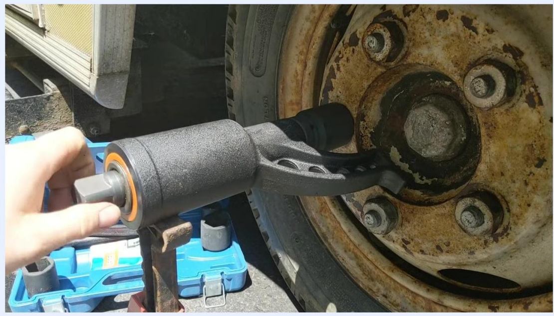
Torque multiplier socket attached to a rusty lug nut on a large vehicle wheel, blue tool case open on the ground, jack stand supporting the tool, and additional sockets visible
