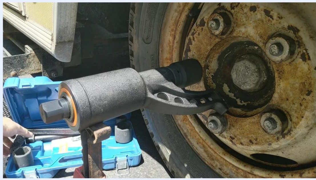
Hand reaching for the short handle in the blue case, with the torque multiplier in place on the lug nut and the jack stand supporting the tool
