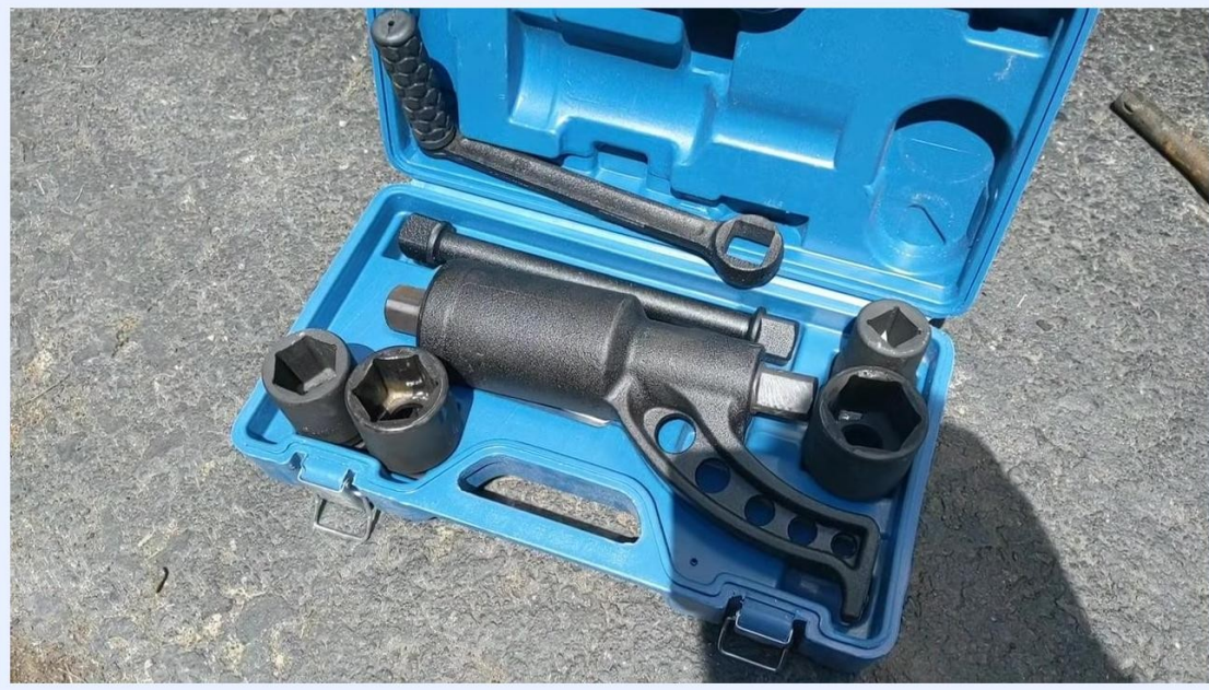
Open blue torque multiplier kit on the pavement, showing the torque multiplier, sockets, handle, and extension bar neatly arranged in molded slots
