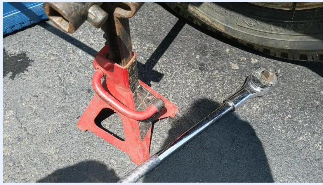
Red jack stand supporting a lug wrench, with a large chrome ratchet and extension pipe lying on the ground nearby
