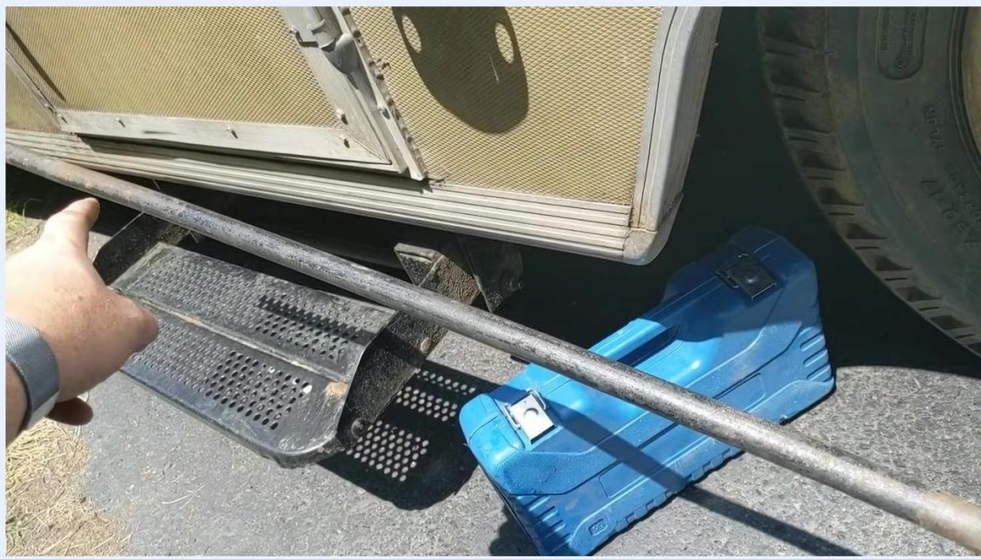
Long metal bar attached to a lug wrench, bent from excessive force, with a hand pointing at the bend and an RV step visible
