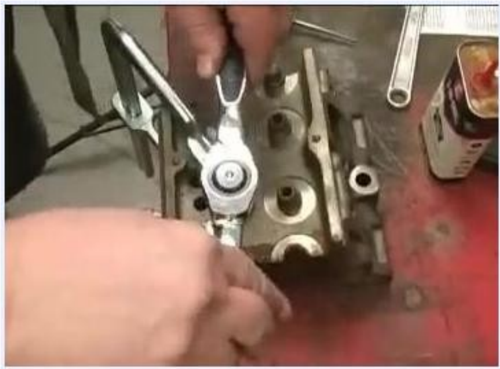
A ratcheting tap handle being used to turn a tap into a metal workpiece, with tools and oil visible on the workbench
