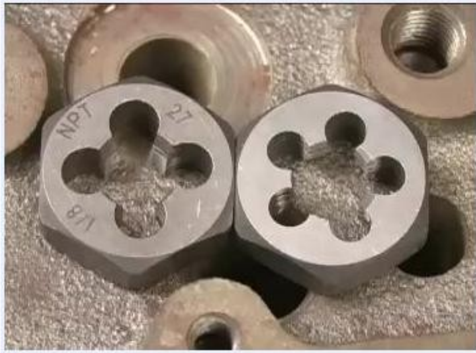
Close-up of two dies, one with the bottom side showing the marking "NPT 1/8 27" facing up
