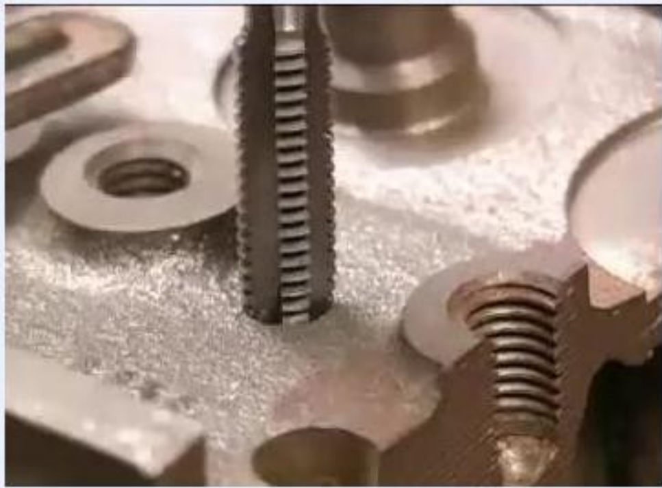
A tap being carefully aligned and started into a drilled hole in a metal workpiece, with several threaded and unthreaded holes visible on the workpiece
