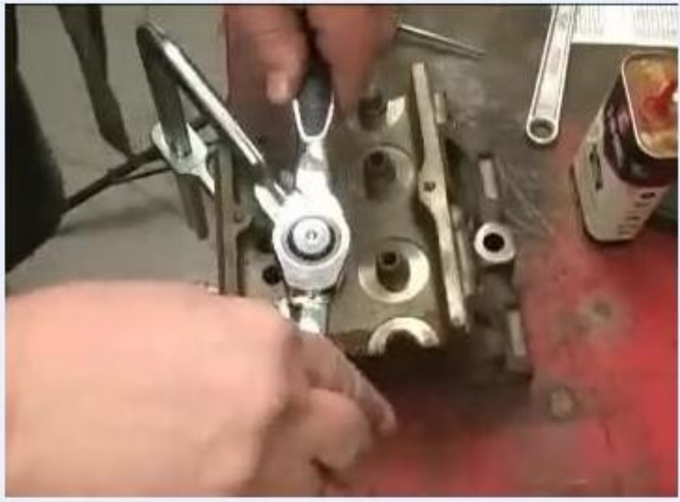
A tap partially inserted into a metal hole, with visible oil and metal chips around the entry point
