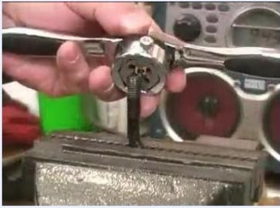
A die being started onto a rod held in a vise, using a die handle to turn it
