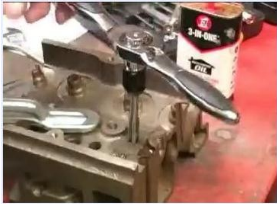
A ratcheting tap handle positioned above a threaded hole, with a can of 3-IN-ONE oil on the workbench nearby
