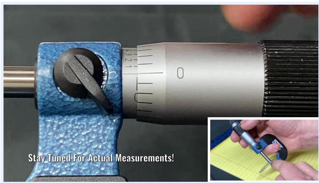
Micrometer close-up showing the thimble and sleeve perfectly aligned at zero.
