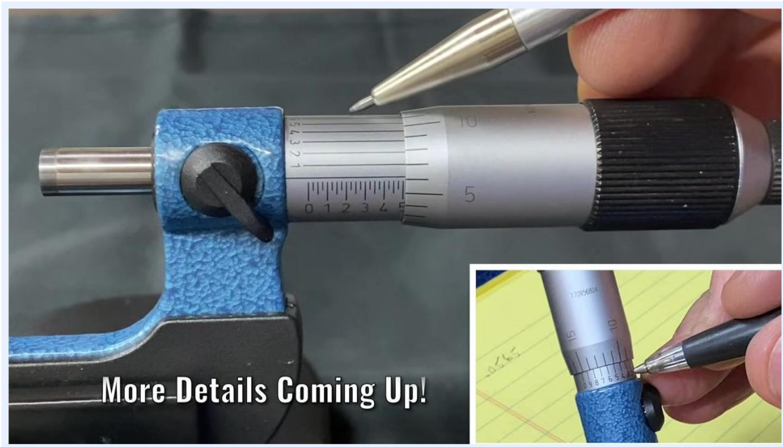
Micrometer with a pen pointing to the auxiliary lines on the sleeve, with an inset close-up of the auxiliary scale.
