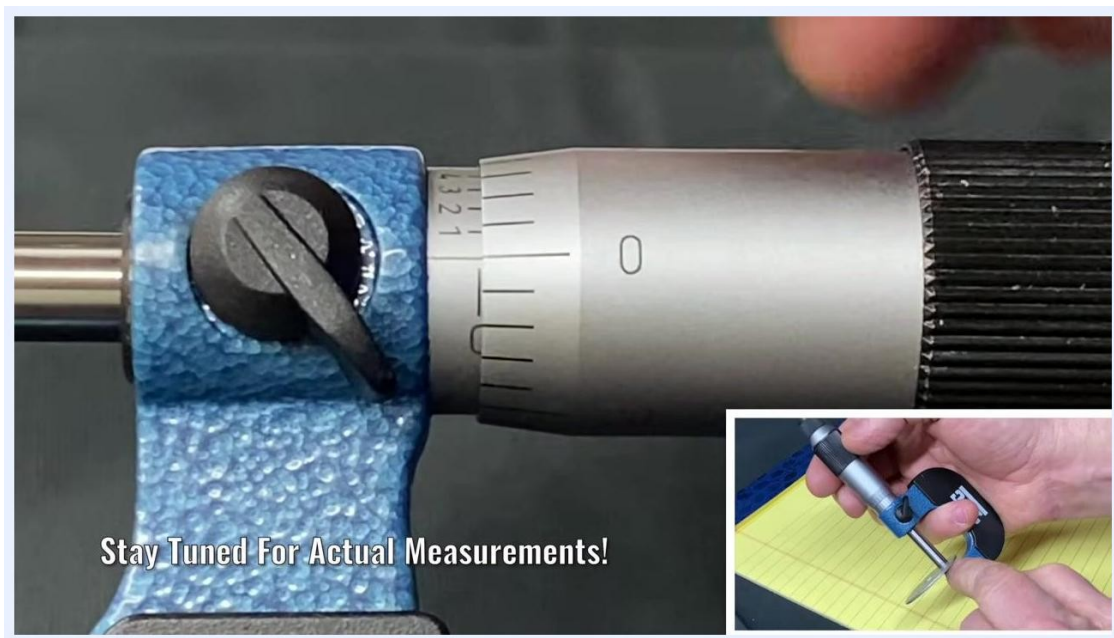
Micrometer close-up with the thimble at zero and a small line on the sleeve visible, indicating the 25-thousandths position.
