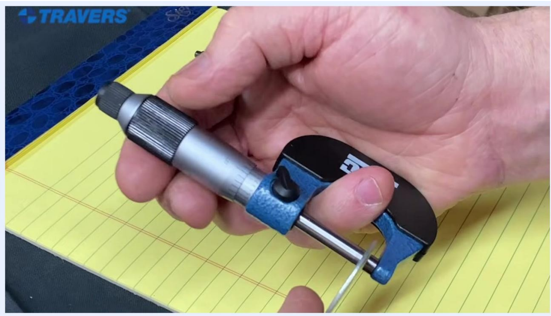
A hand holding the micrometer with the frame in the palm and the ring finger resting on the thimble.
