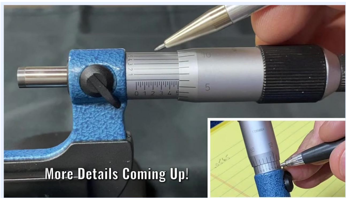
Micrometer with a pen pointing to the "5" mark on the sleeve, preparing to use the auxiliary scale.
