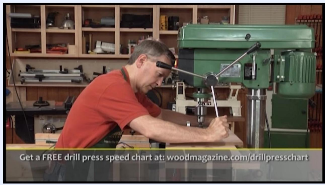
Backer board and clamps positioned under a large board on the drill press table
