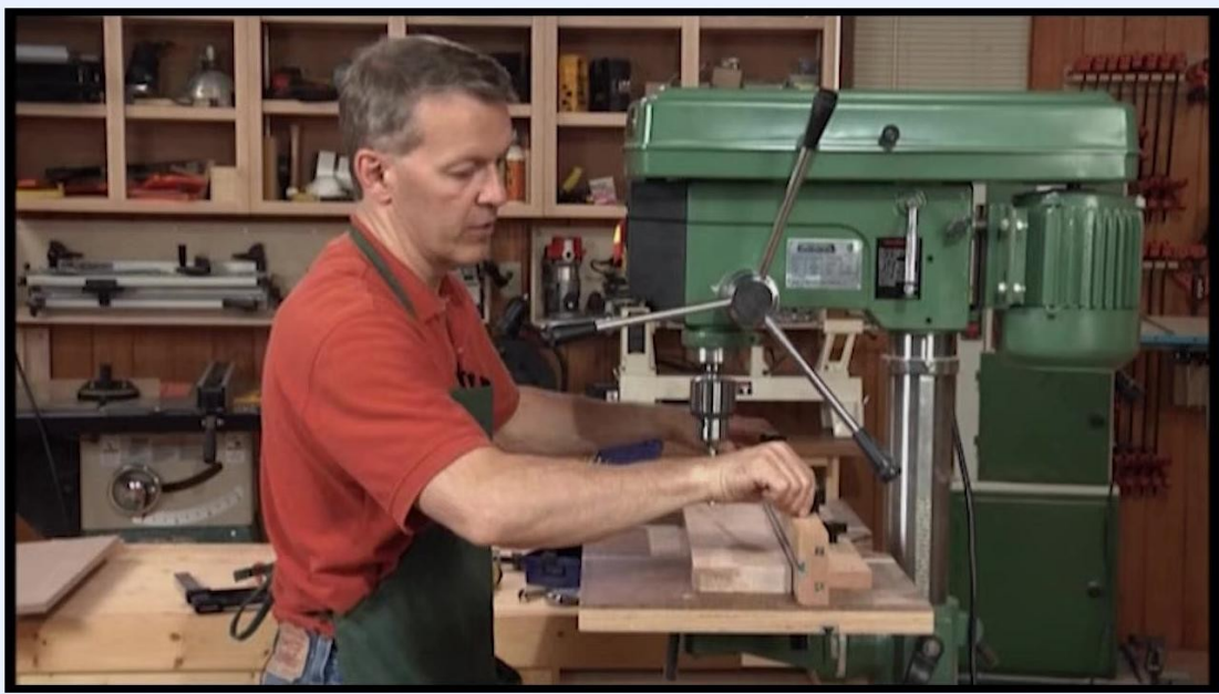
Operator extending the table wings and adjusting stop blocks for repetitive drilling tasks
