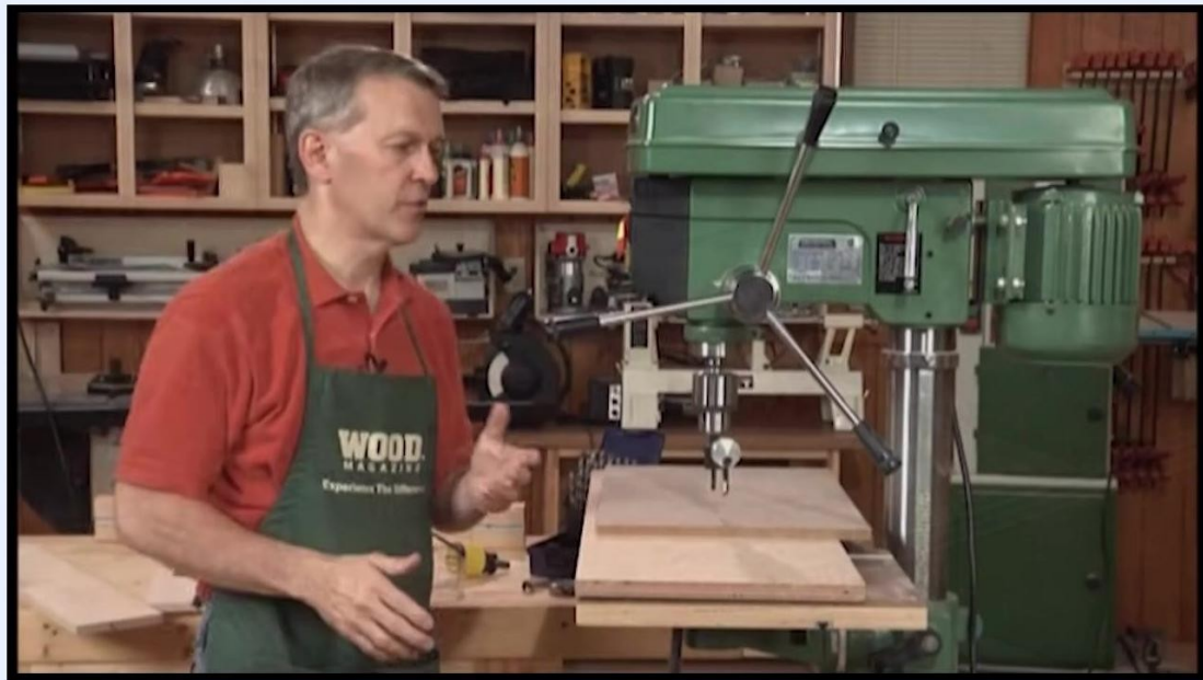
Operator adjusting the drill press table height with the workpiece positioned under the drum sander
