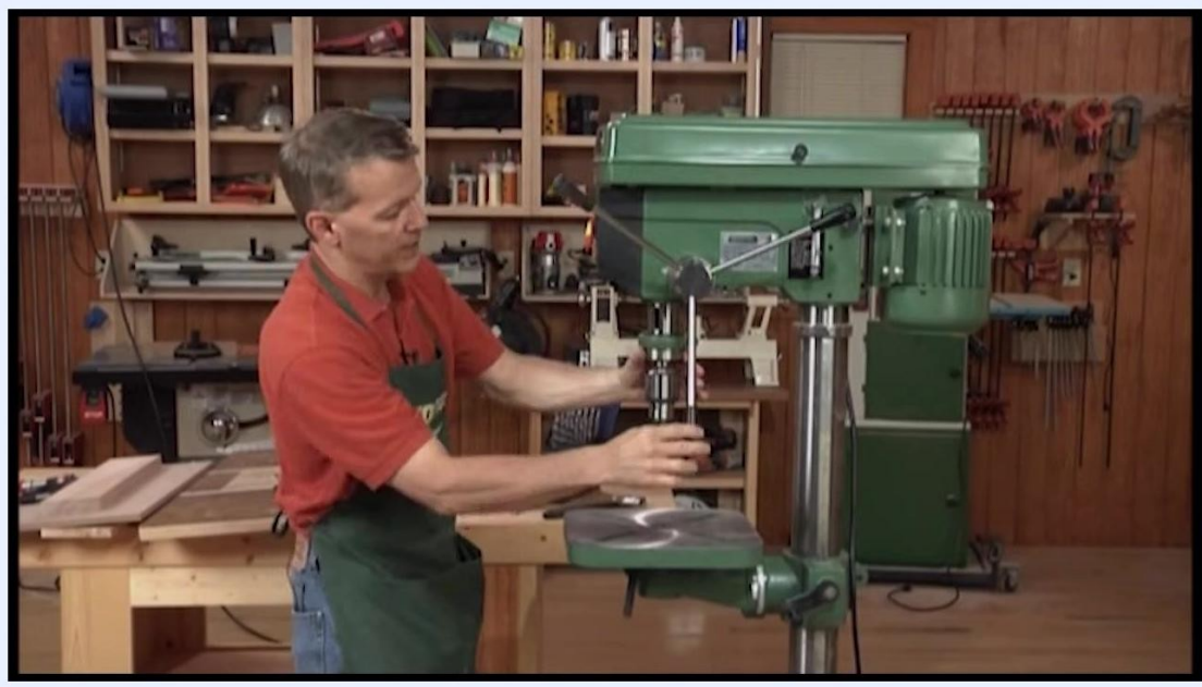
Operator adjusting the screw-type depth stop on the drill press column
