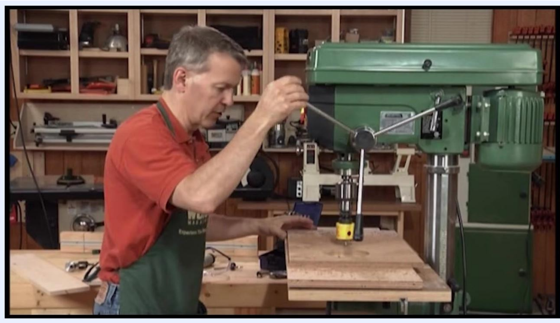
Wooden workpiece clamped to the drill press table with a yellow hole saw attached
