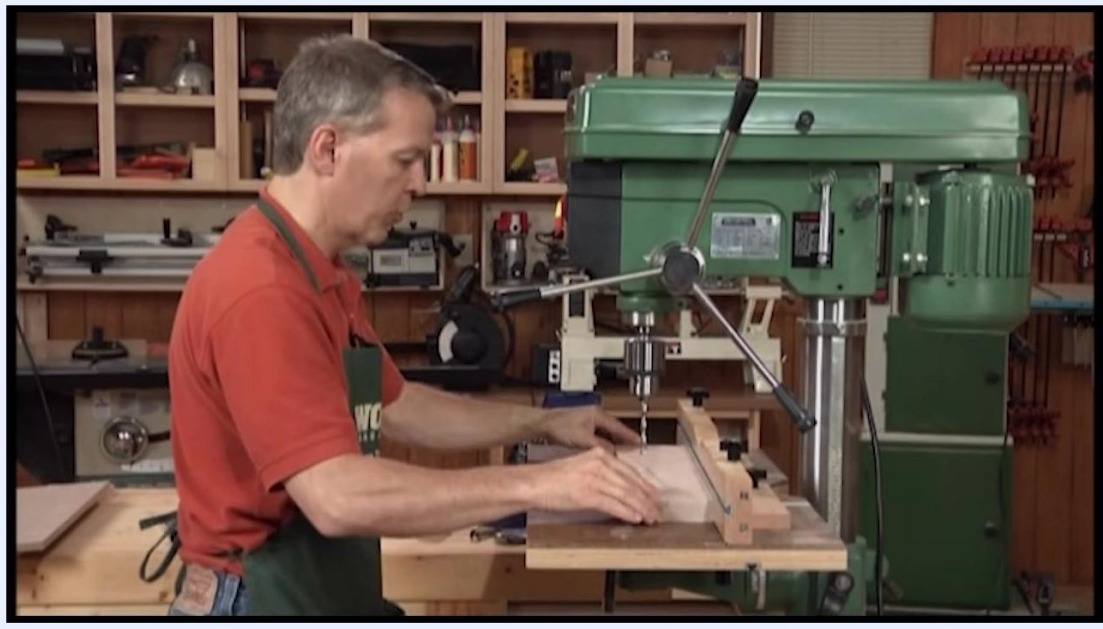
Operator positioning a workpiece against the adjustable fence for consistent hole spacing
