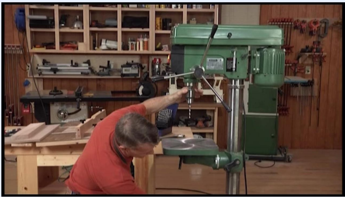
Operator adjusting the drill press table height using the geared handle on the column
