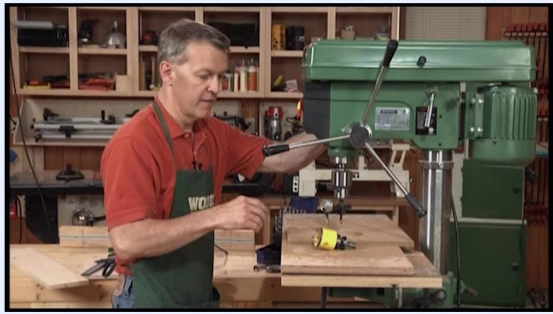
Preparing to clamp a wooden workpiece with a yellow hole saw attached to the drill press
