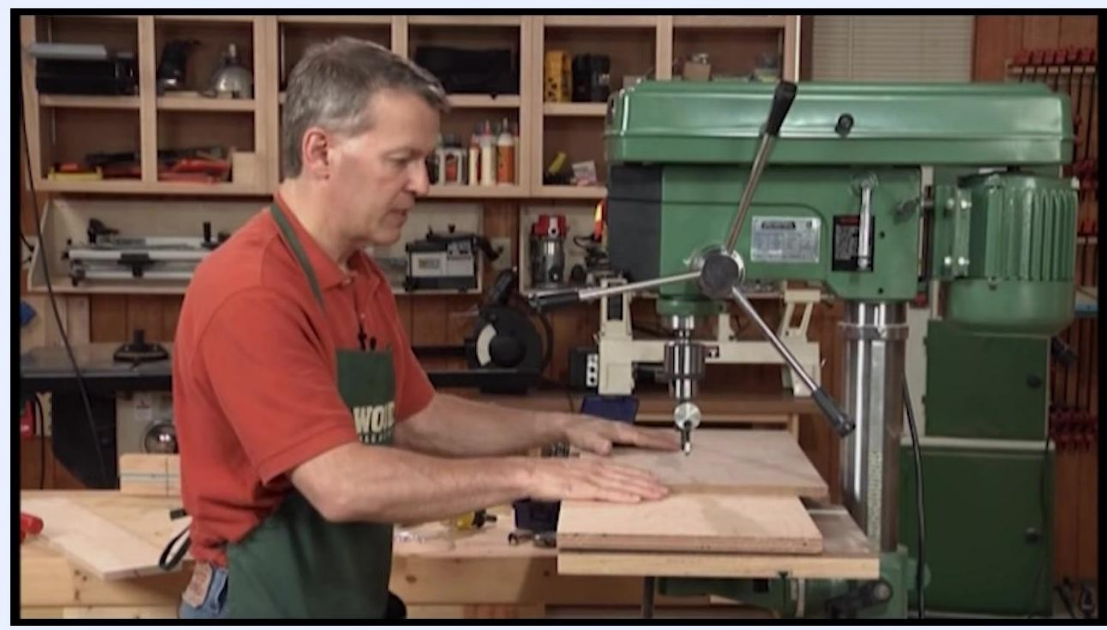
Large wooden board positioned on the drill press table, extending beyond the fence
