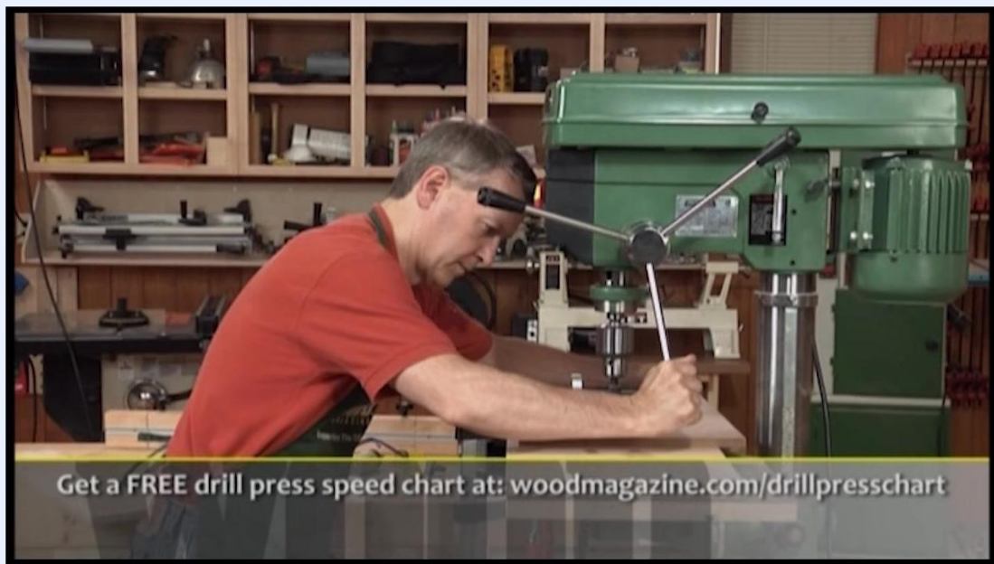
Demonstration of safe hand placement on a large board at the drill press, keeping hands away from the spinning bit
