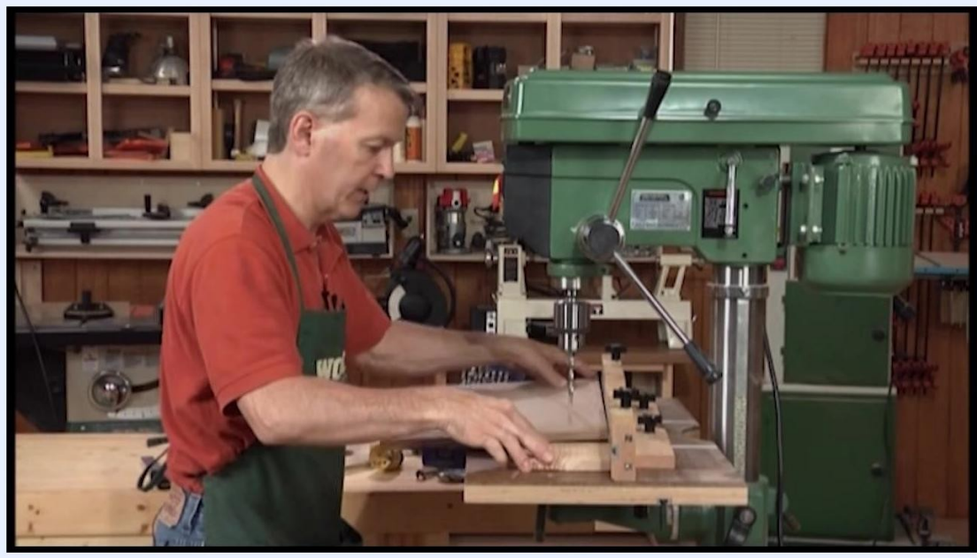
Close-up of a hand holding the workpiece steady as the drill bit approaches, with a backer board visible underneath
