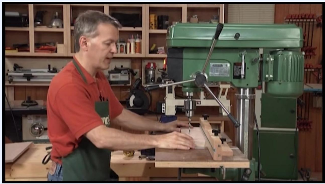
Operator holding a workpiece against the fence to demonstrate improved drilling safety
