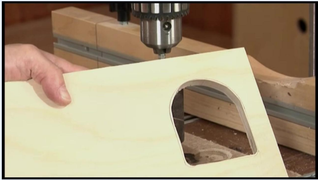
Close-up of a hand holding a wooden workpiece with a curved cutout near the drum sander, with the pencil line visible
