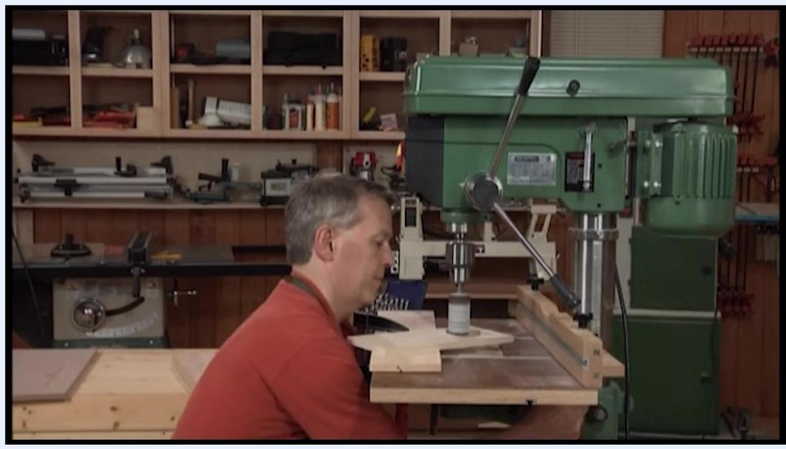
Hands positioning a wooden workpiece on the drill press table, with the sanding drum and wood dust visible
