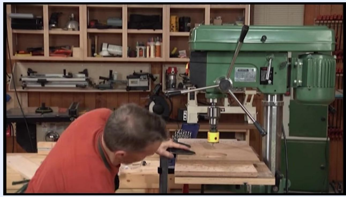
Close inspection of the clamped workpiece and hole saw setup on the drill press
