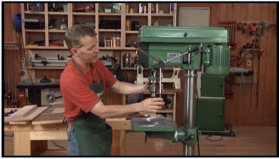
Operator raising and lowering the quill assembly using the side handle of the drill press
