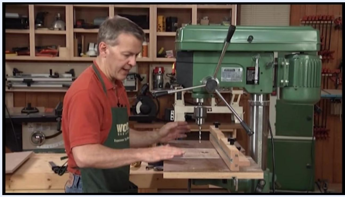
Large woodworking drill press table with fence and accessories installed on the drill press
