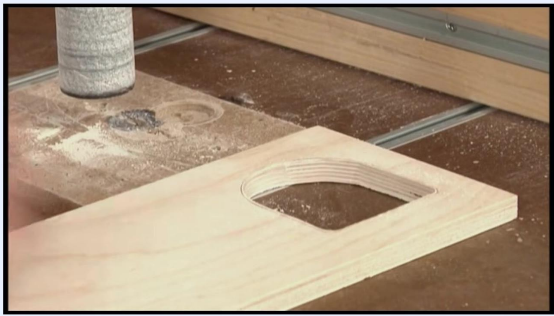
Wooden workpiece positioned near the drum sander with a scrap block clamped in front of the drum as a stop
