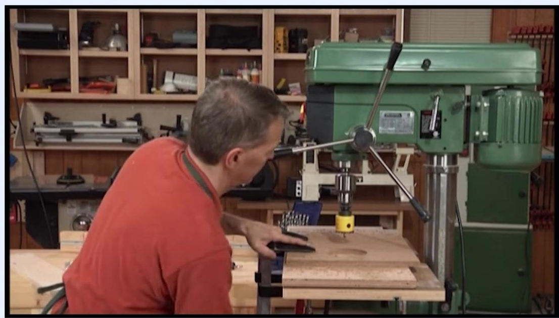
Drill press operating with a yellow hole saw, with the workpiece clamped and the machine set to slow speed
