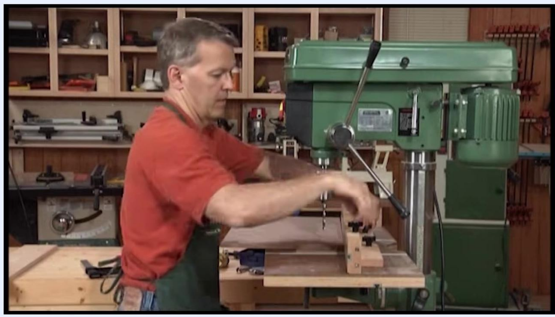
Operator adjusting and locking down a wooden fence on the drill press table
