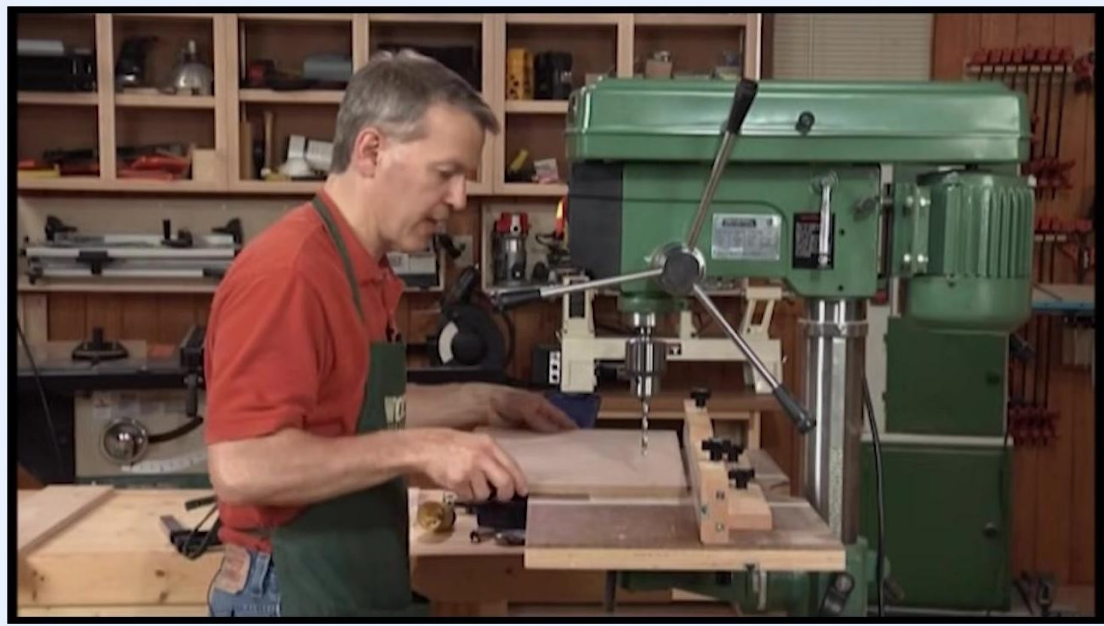
Operator positioning a marked workpiece under the drill bit using the fence for alignment
