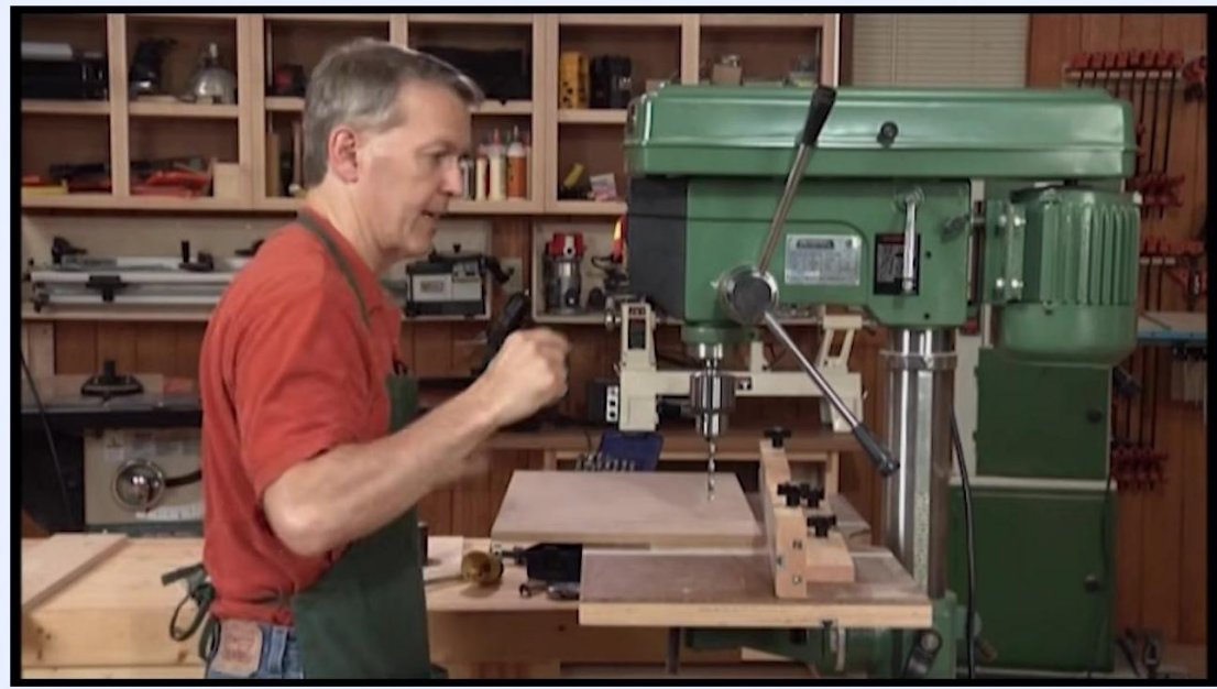
Operator positioning the workpiece under the drill bit with the handle removed, aligned with the fence and stop blocks
