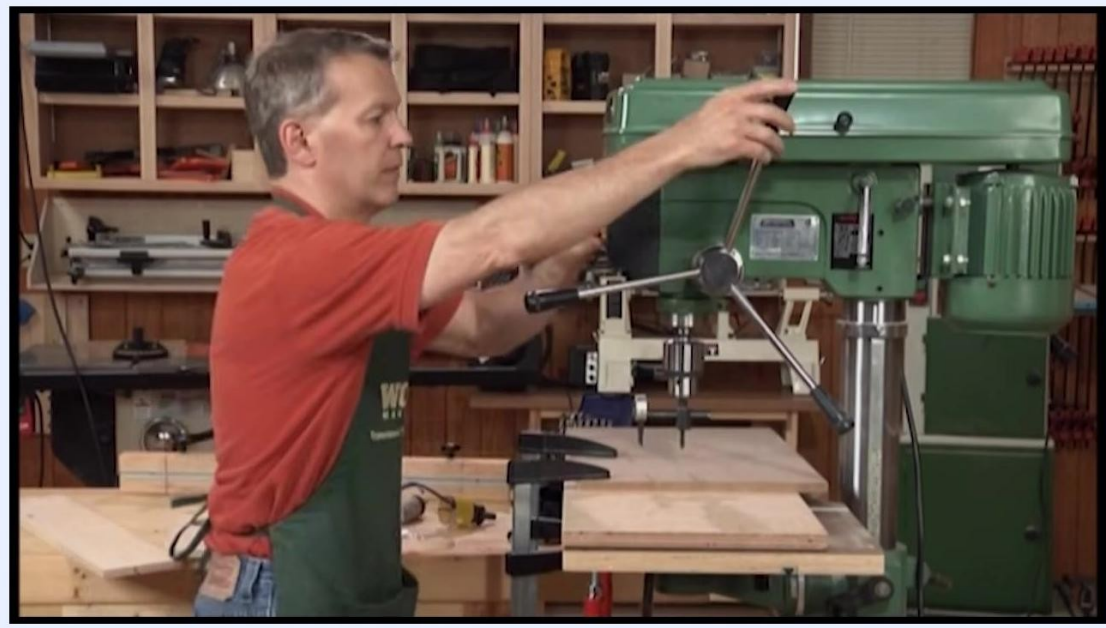
Operator adjusting and locking the fence on the drill press table with the workpiece clamped in place
