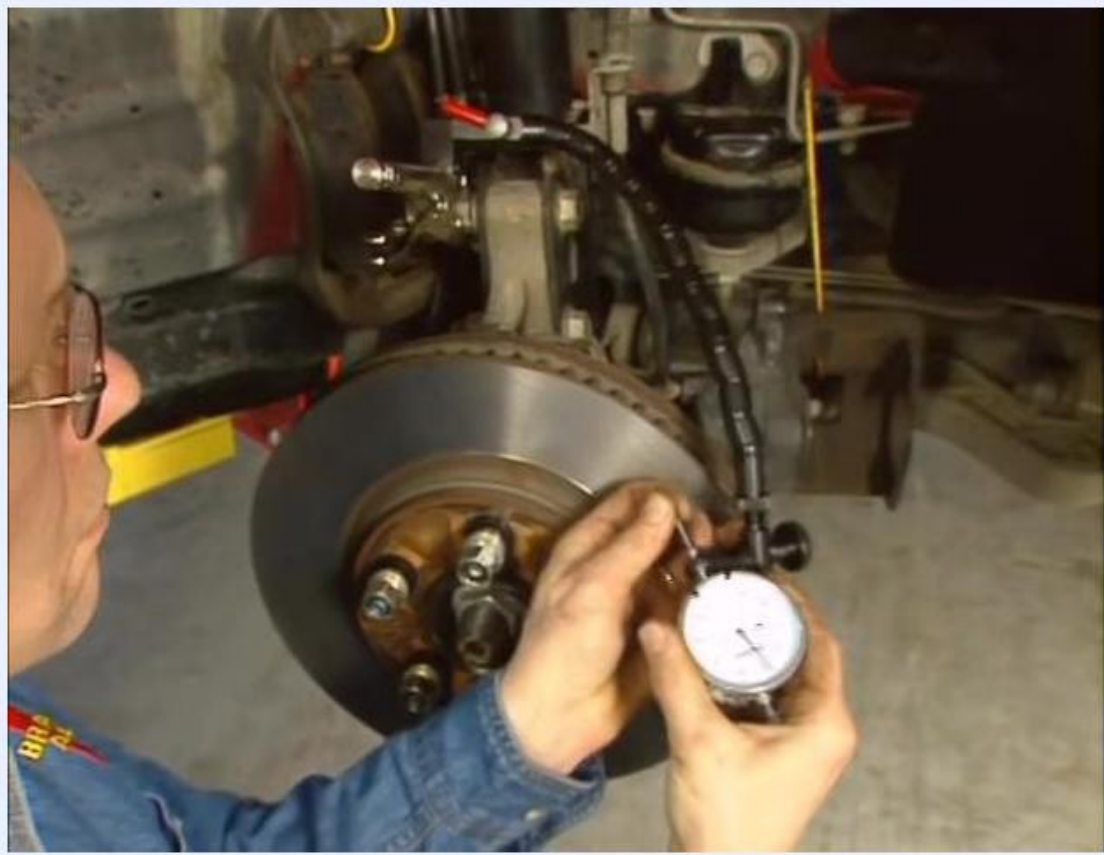
Person checking and tightening the contact tip of the dial indicator, with the flex arm and rotor visible.
