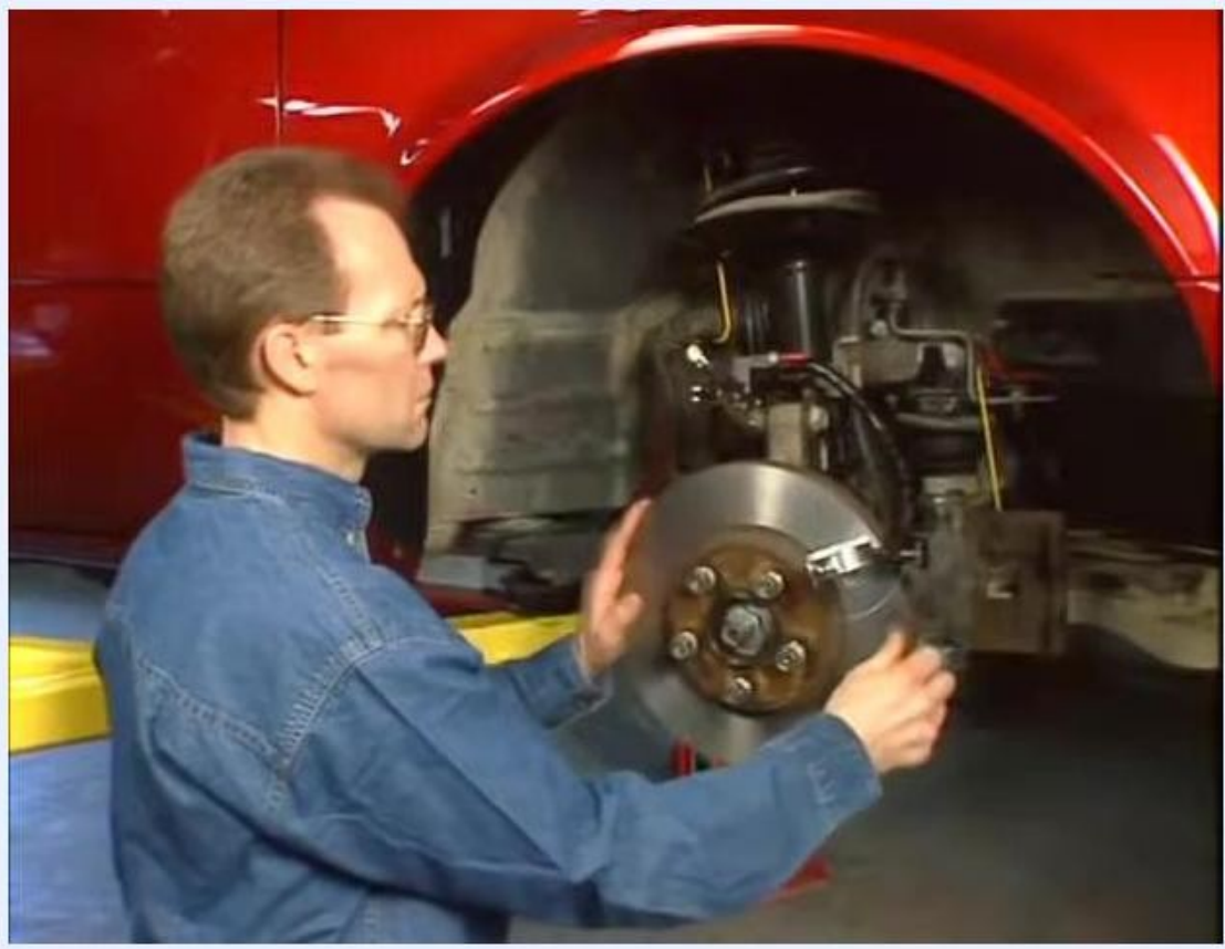
Technician rotating the brake rotor by hand while observing the dial indicator to find the high spot.
