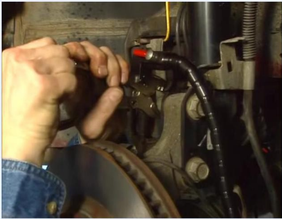
Hands adjusting the knurled knob on a vise grip clamped to a vehicle suspension component, with a brake rotor visible in the foreground.
