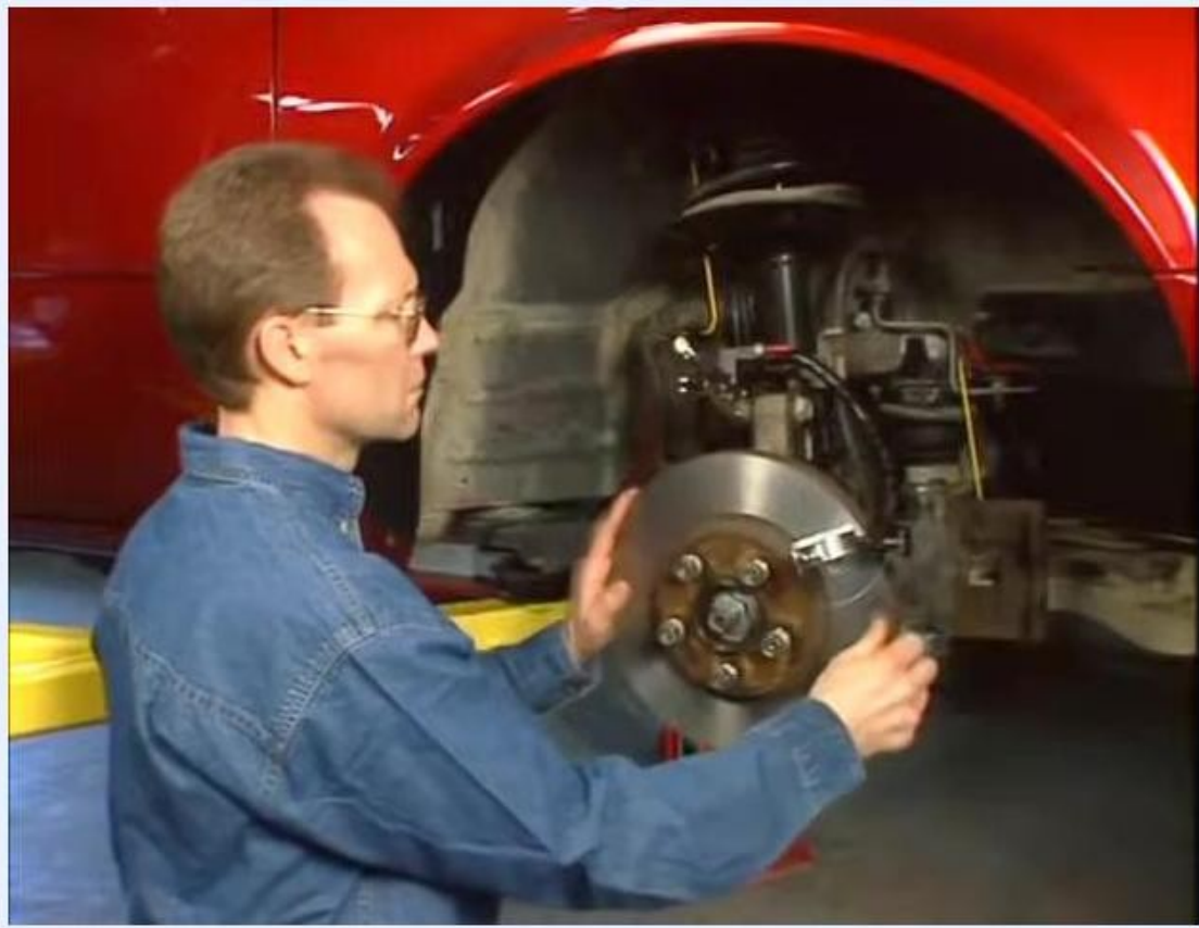
Technician closely monitoring the dial indicator as the rotor is rotated to the high spot.
