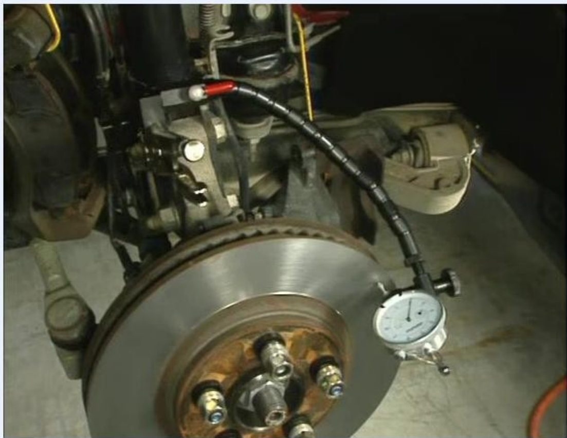
Dial indicator gauge being zeroed at the low spot, with the needle pointing to zero.
