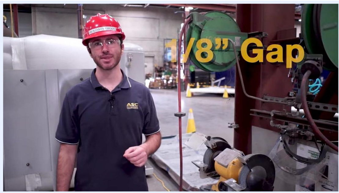
A bench grinder in an industrial setting with on-screen text reading "1/8" Gap," reinforcing the correct work rest and guard adjustment.
