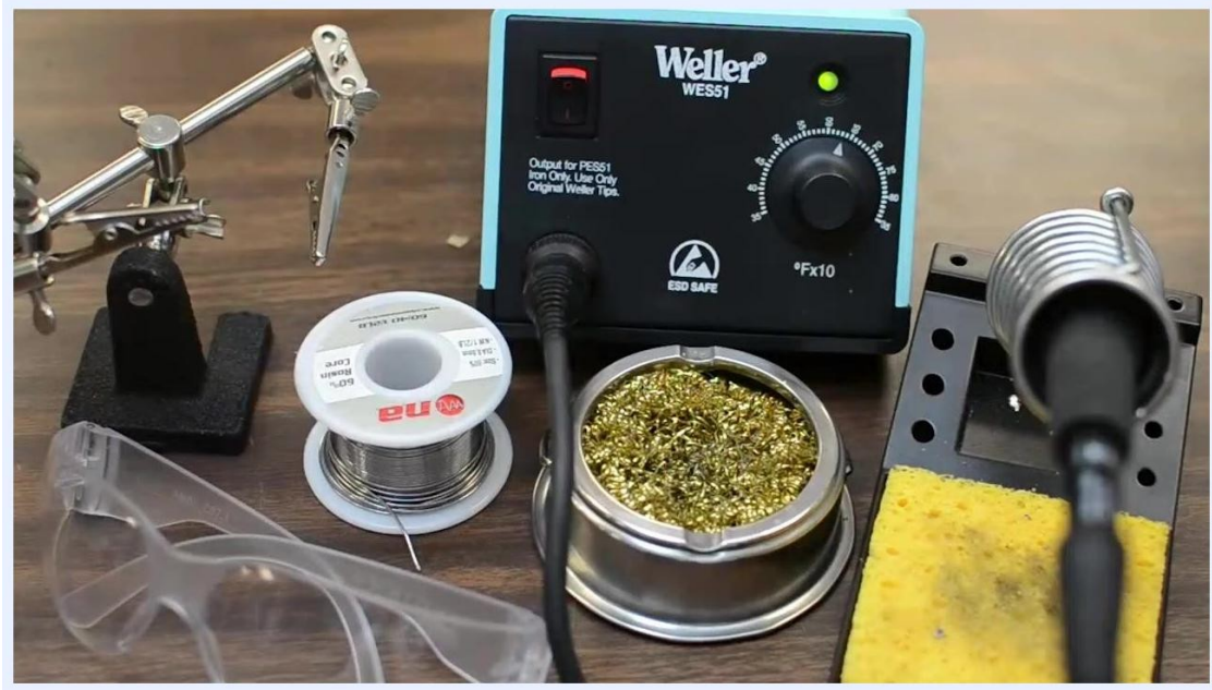
A complete soldering setup on a workbench: Weller WES51 soldering station, spool of solder, brass sponge, yellow cleaning sponge, helping hands tool, and clear safety goggles
