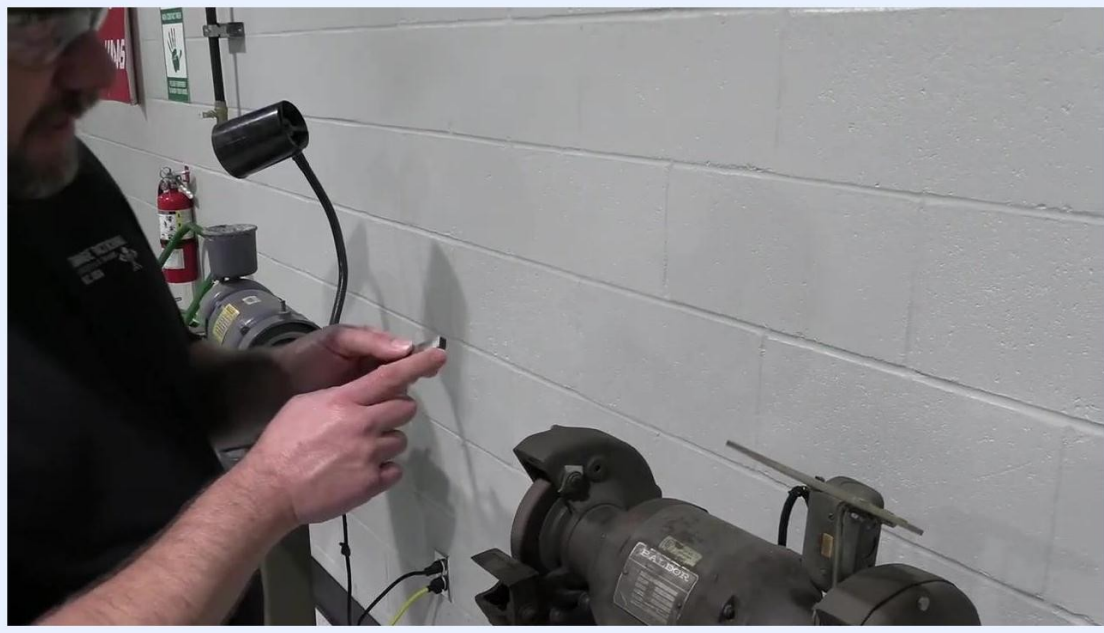
A hand points to the slanted side of the tool bit near the bench grinder, with safety signage visible in the background.
