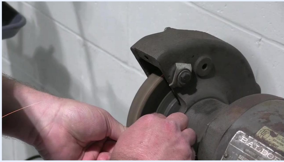
Hands hold the tool bit against the grinding wheel with a small spark visible, indicating active grinding.
