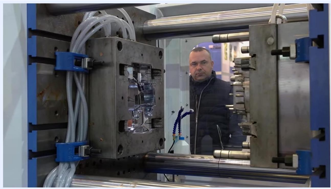
Close-up of an injection mold with hoses and a person observing, illustrating the importance of proper mold clamping
