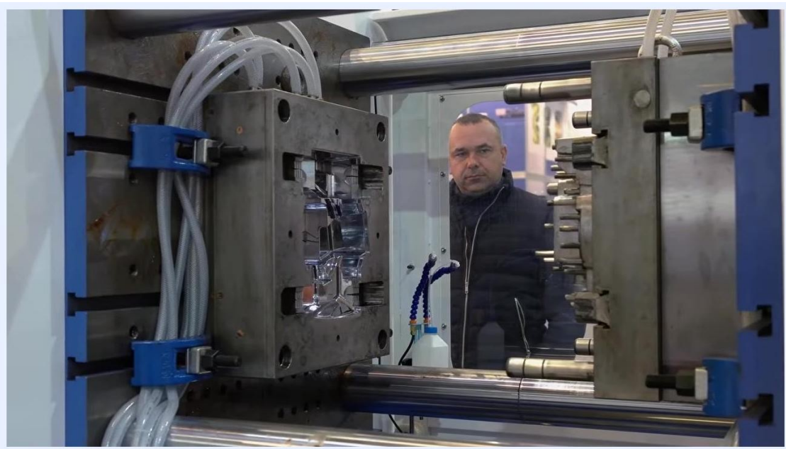
Step 5: Opening and repeating, diagram of the injection molding machine with the mold open
