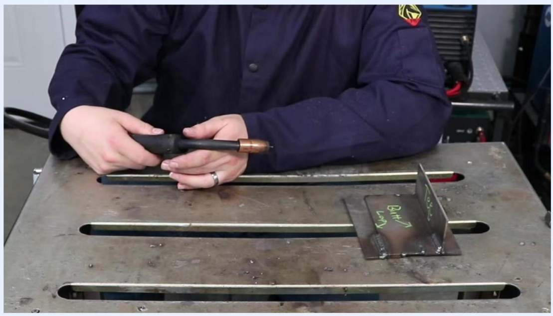
Person holding the MIG gun with both hands, workpiece set up for welding, emphasizing travel speed and movement
