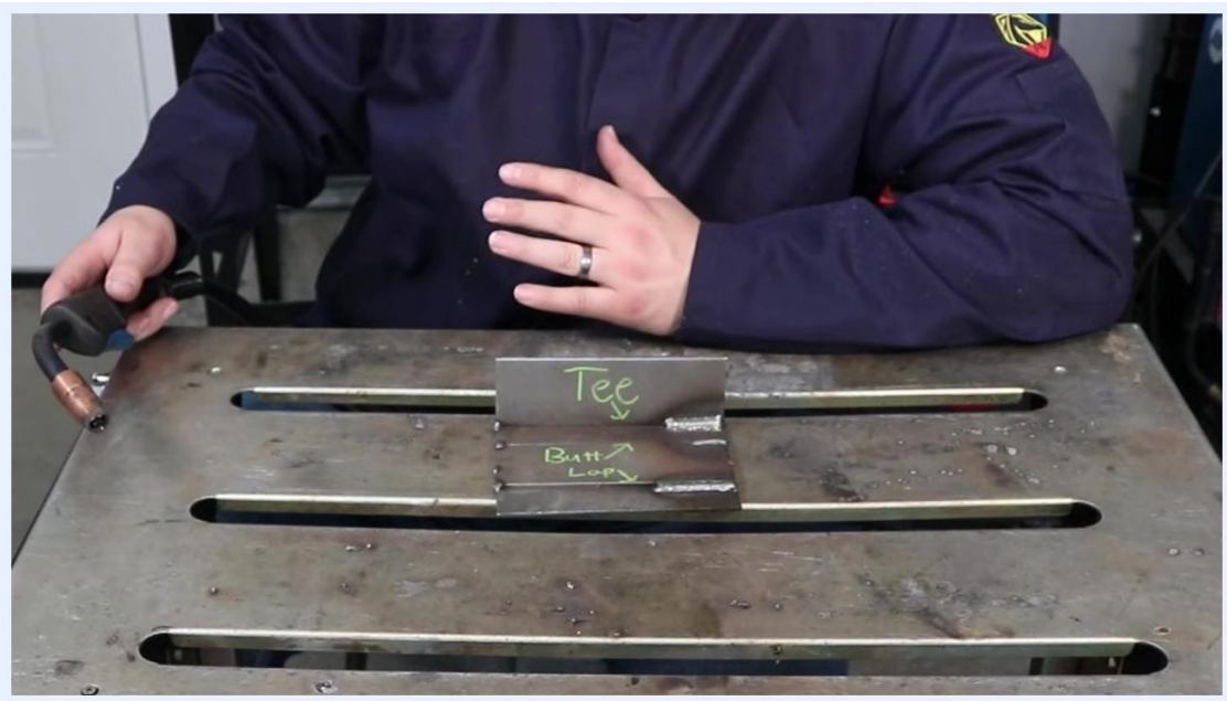
Person in a welding jacket holding a MIG gun above two labeled metal plates, "Tee" and "Butt/Loop," on a metal workbench, demonstrating dry run practice
