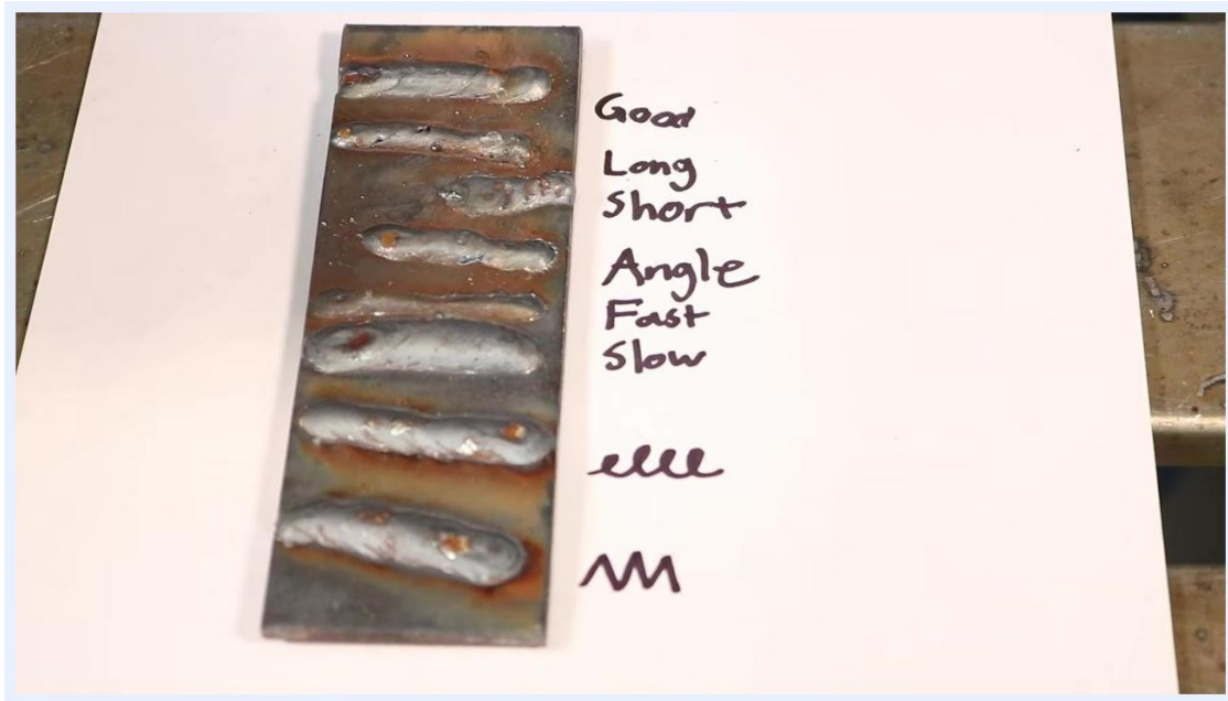
Close-up of a weld bead plate, illustrating burn-through and other issues caused by incorrect technique
