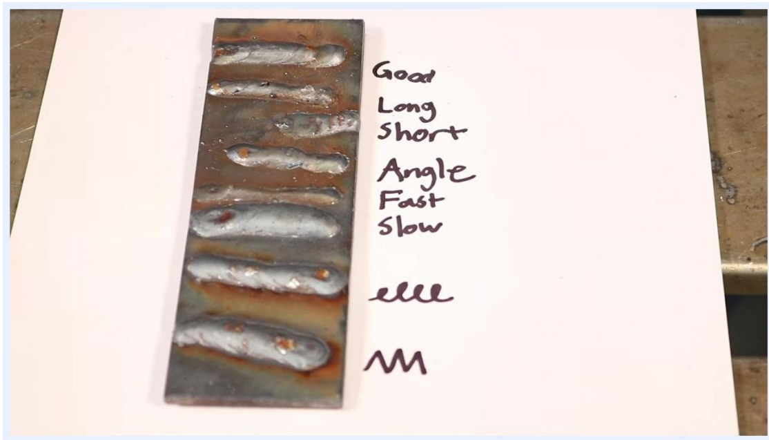
Close-up of a weld bead plate showing porosity and other defects, with handwritten labels for each weld type
