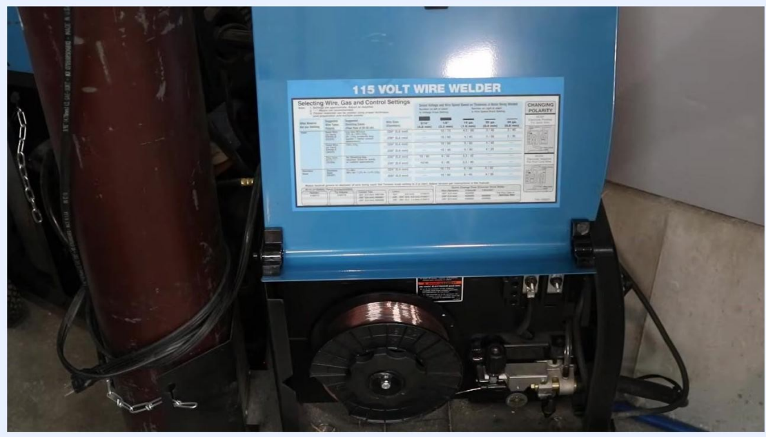
Close-up of a 115 Volt wire welder with the settings chart visible inside the open panel, showing wire, gas, and control settings for different material thicknesses and wire diameters
