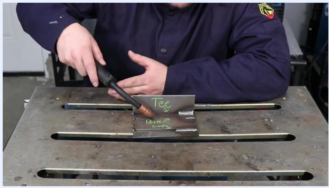
Person holding the MIG gun at an angle over the "Tee" and "Butt/Loop" plates, discussing angle importance in out-of-position welding
