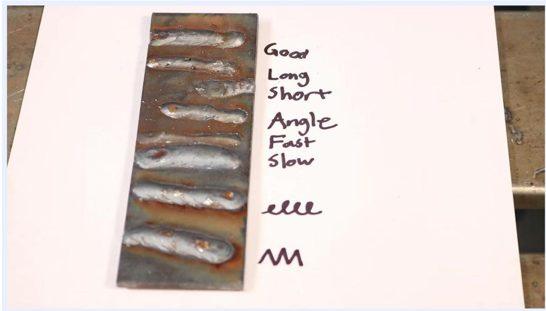
Close-up of a metal plate with multiple weld beads, each labeled: Good, Long, Short, Angle, Fast, Slow, E-pattern, M-pattern
