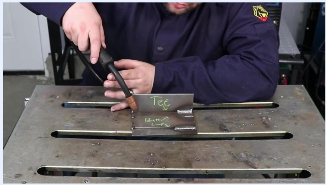
Person demonstrating MIG gun angle toward the "Tee" joint, emphasizing the importance of correct angles to avoid spatter
