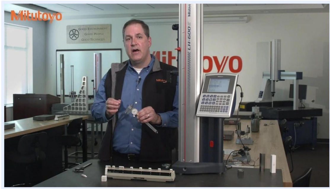
Measuring a 0.200-inch ring gauge with the inside jaws of a digital caliper; the calibration fixture is marked "INSIDE," with a 1-inch Mitutoyo gauge block and ring gauge visible
