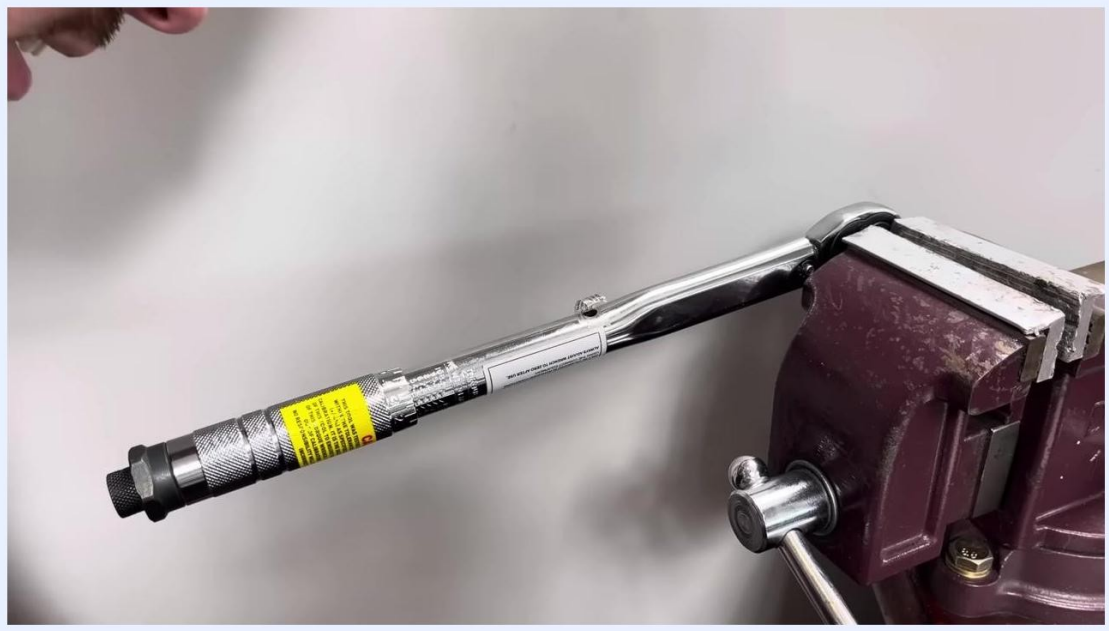
A torque wrench is clamped in a bench vise, with the handle and calibration label visible during inspection for further adjustment.
