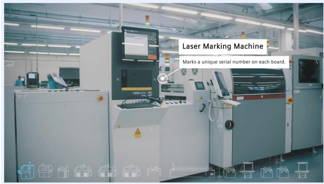
Laser marking machine labeled "NEOMARK easy," with a screen and control panel, and a callout indicating it marks a unique serial number on each board
