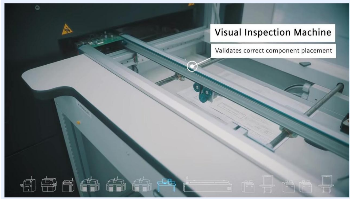
Visual inspection machine with callout "Validates correct component placement," showing PCB on conveyor
