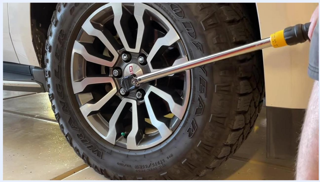
Torque wrench being used on a lug nut, with the user applying force to tighten it.
