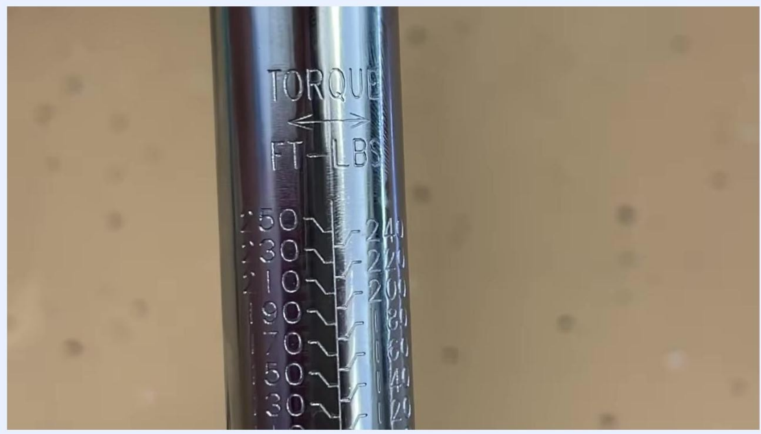
Close-up of the torque wrench shaft showing the FT-LBS scale, with values from 50 to 250 foot-pounds.
