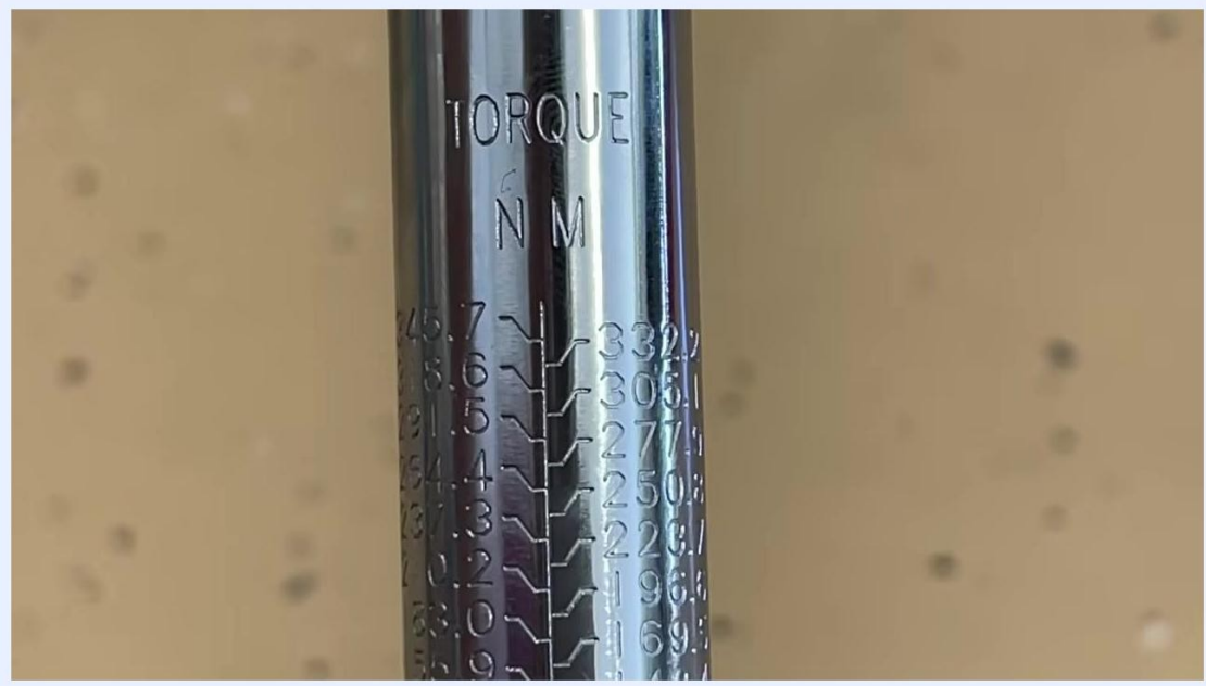
Close-up of the torque wrench shaft showing the Newton-meter (Nm) scale, with values from 74.6 to 345.7 Nm.
