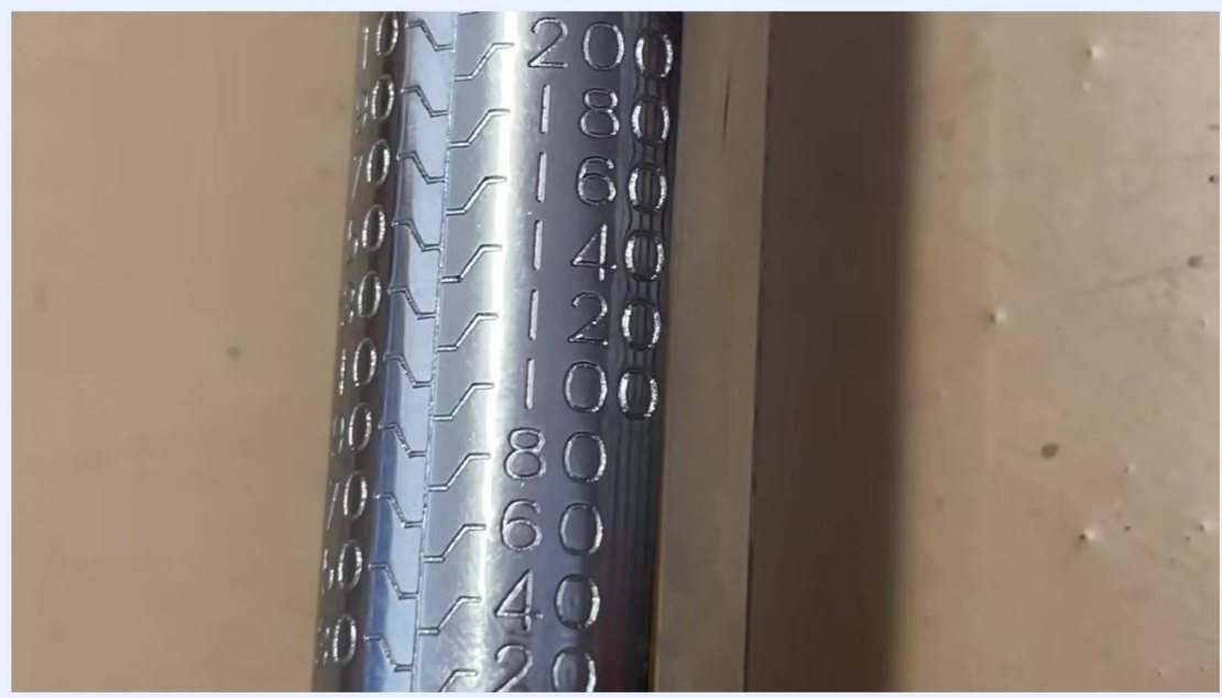
Close-up of the torque wrench shaft showing the 100 ft-lb mark and its drop-down reference line.
