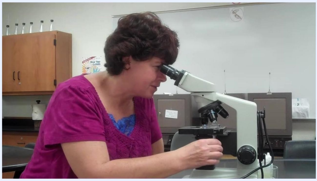
Instructor demonstrating troubleshooting by returning to the 10x objective and adjusting focus, emphasizing centering the specimen.
