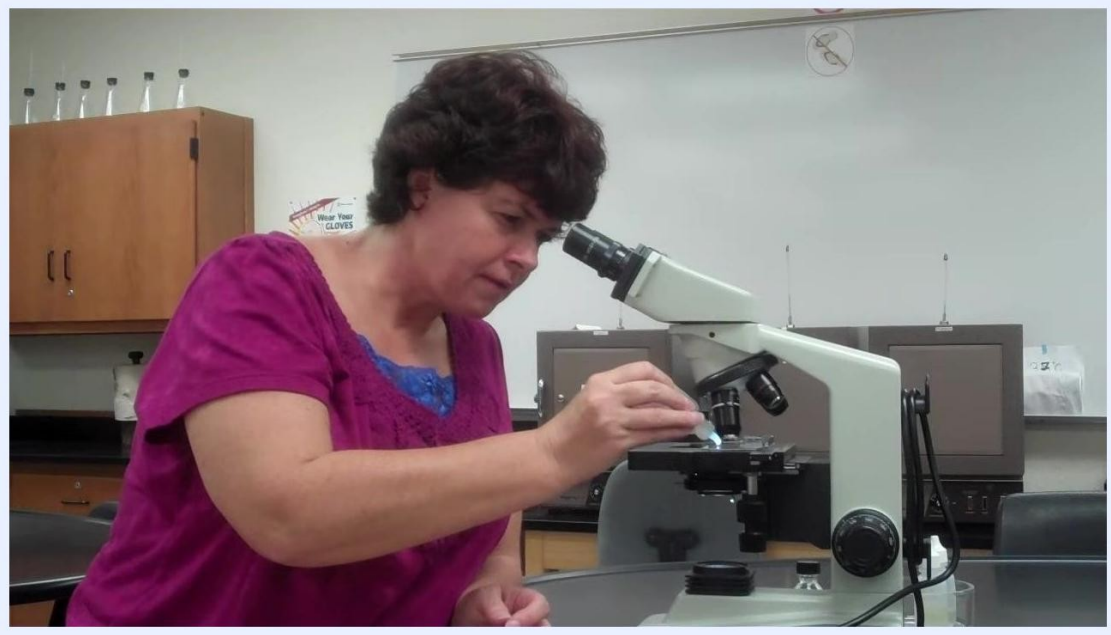
Instructor leaning in and carefully applying a drop of immersion oil to the slide, ensuring the dropper does not touch the slide.
