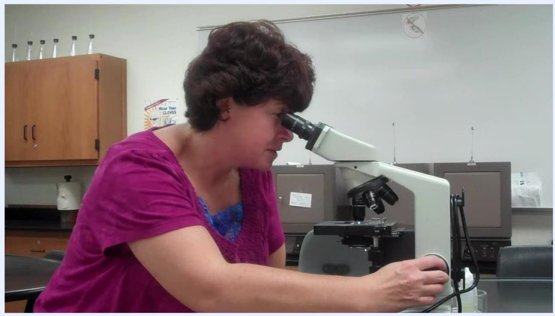
Instructor looking through the microscope and adjusting the fine focus knob to achieve a clear image under the 100x objective.
