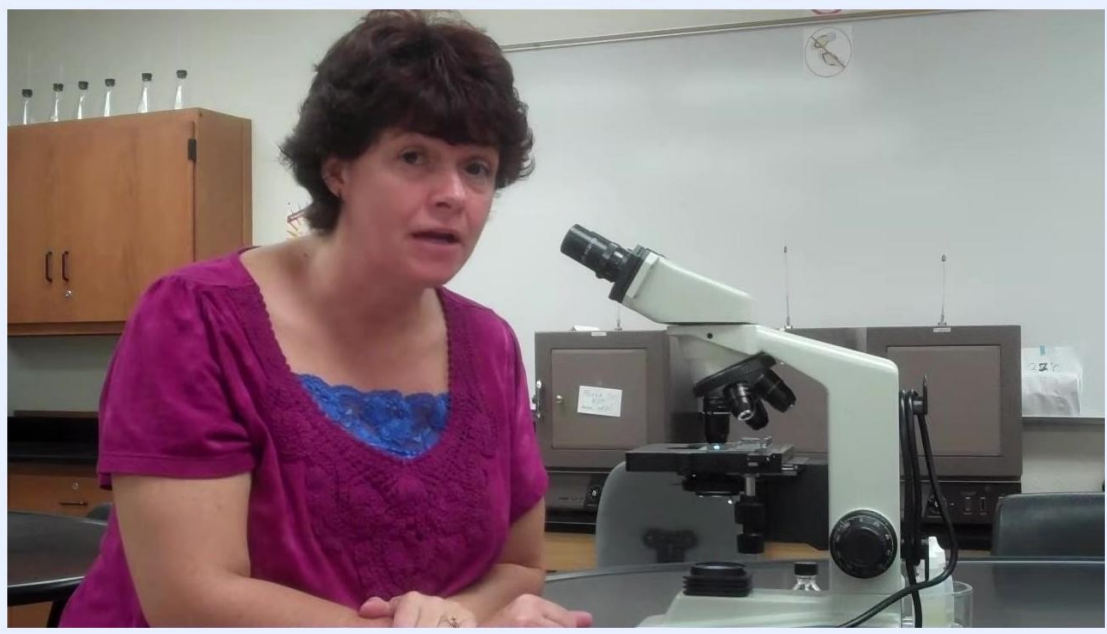
Instructor explaining the need to return to the 10x objective if the specimen cannot be found under 100x.
