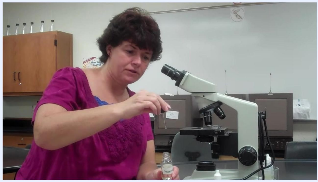
Instructor holding an immersion oil bottle and using a dropper to prepare a drop of oil above the slide, demonstrating proper technique.
