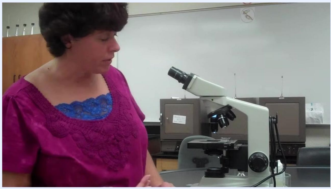
Instructor rotating the microscope nosepiece to the lowest power objective.
