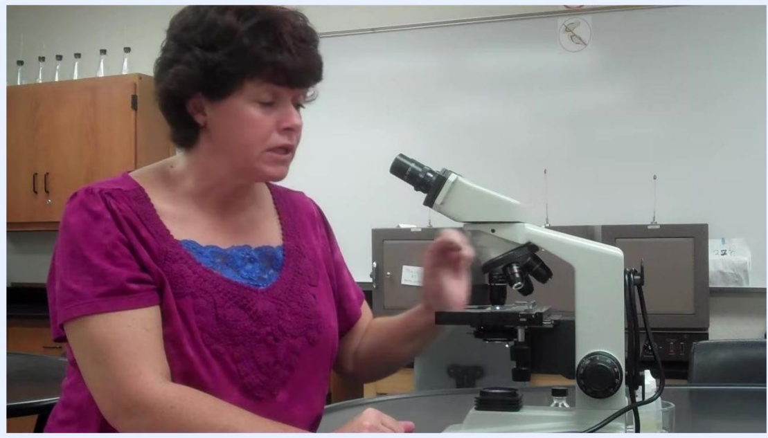
Instructor emphasizing the importance of not switching back to the 40x objective after oil application.
