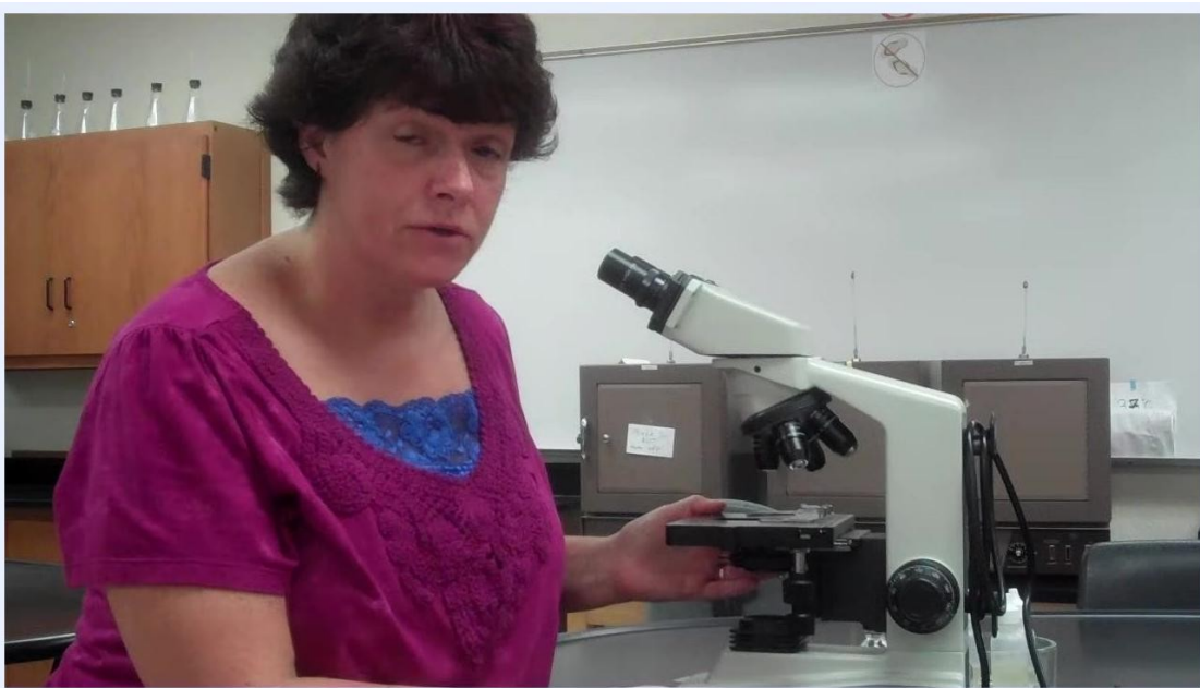
Instructor pointing to the microscope base, warning about heat from the light source.
