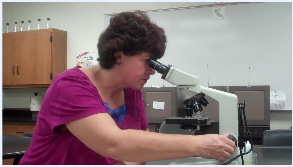
Instructor adjusting the focus knob, emphasizing not to go directly to the 100x objective.
