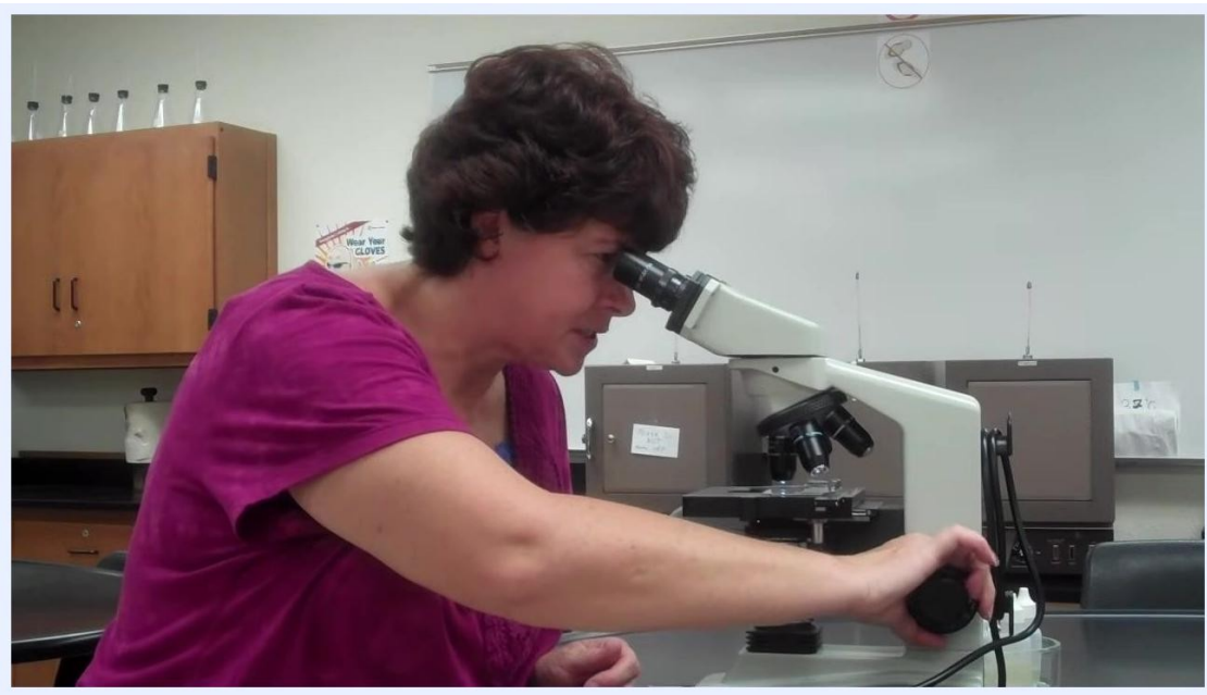
Instructor demonstrating microscope setup while adjusting the coarse focus knob and looking through the eyepiece; a slide is on the stage, with lab safety posters and cabinets in the background.
