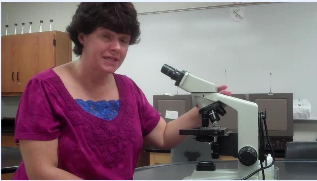
Instructor holding the objective turret between the 40x and 100x positions, preparing for oil application.
