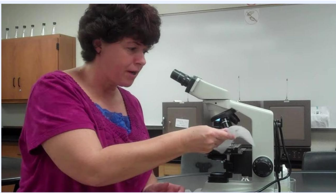
Instructor demonstrating gentle dabbing of the lens with lens paper.
