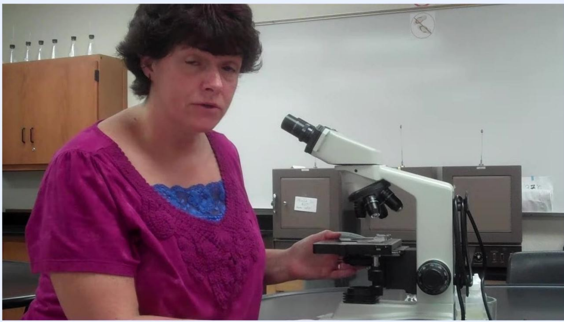
Instructor demonstrating the proper two-handed carrying technique for the microscope.
