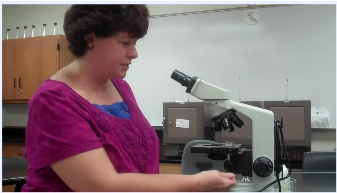
Instructor centering the mechanical stage arm on the microscope.
