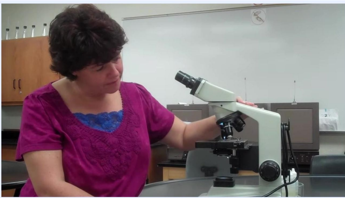
Instructor looking at the slide and turret, preparing to apply oil.
