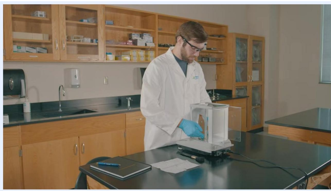
Lab technician removing the weigh pan and components from the analytical balance
