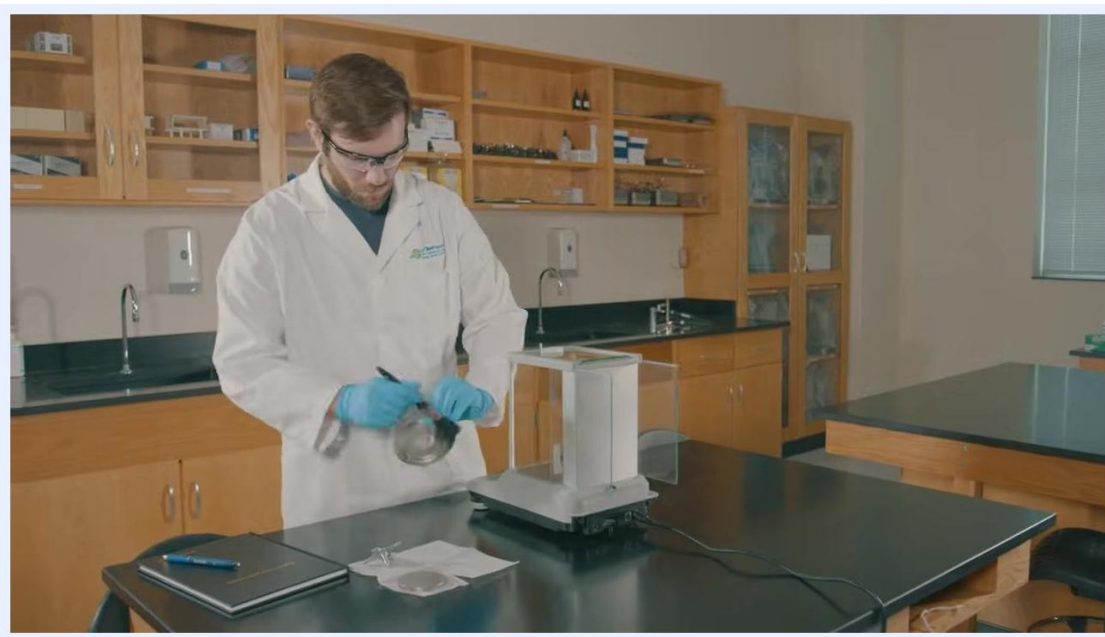
Lab technician replacing the drip ring and weigh pan after cleaning the analytical balance
