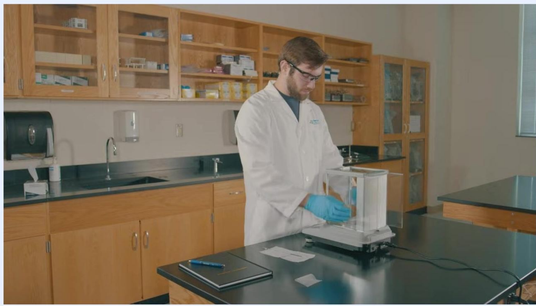
Lab technician in a lab coat and gloves closing the glass doors of the balance after adding sodium bicarbonate
