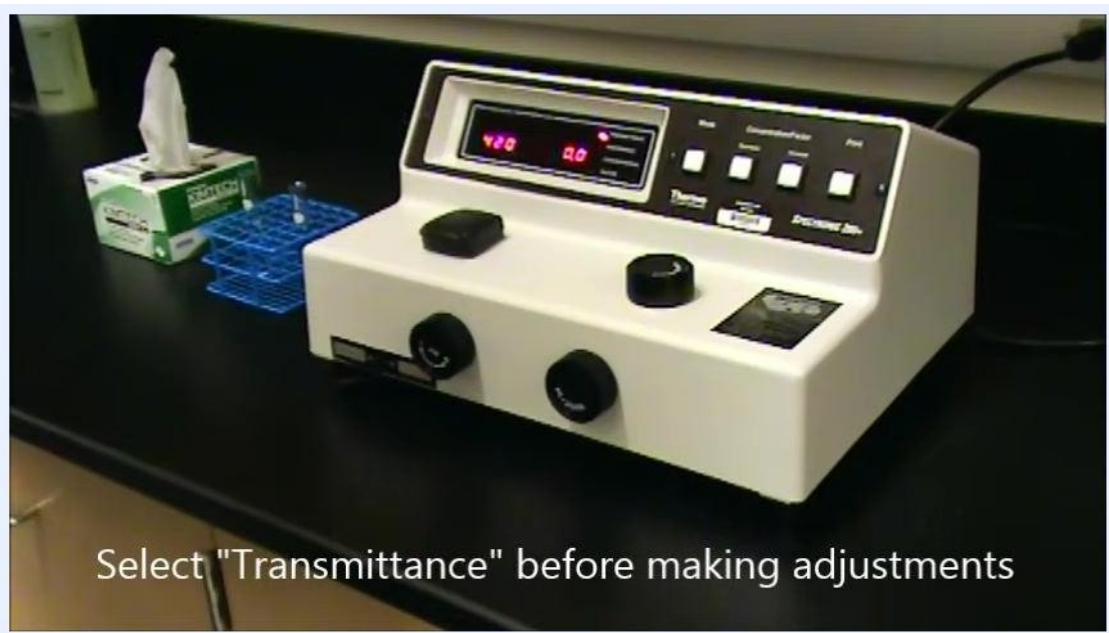
Spectrophotometer display instructing you to select Transmittance before making adjustments
