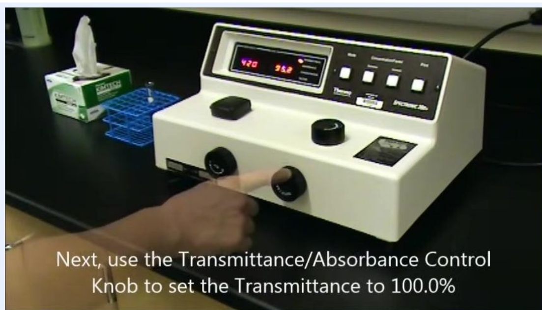
Hand turning the Transmittance/Absorbance Control Knob while the display shows 420 nm and 95.2
