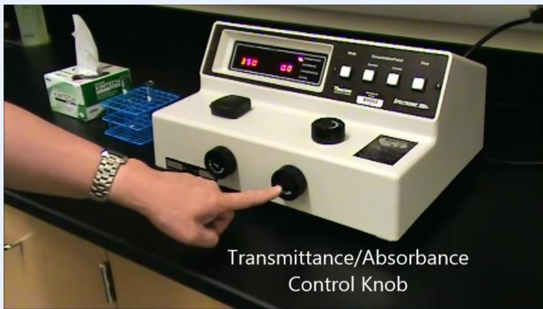
A hand points to the Transmittance/Absorbance Control Knob on the front panel
