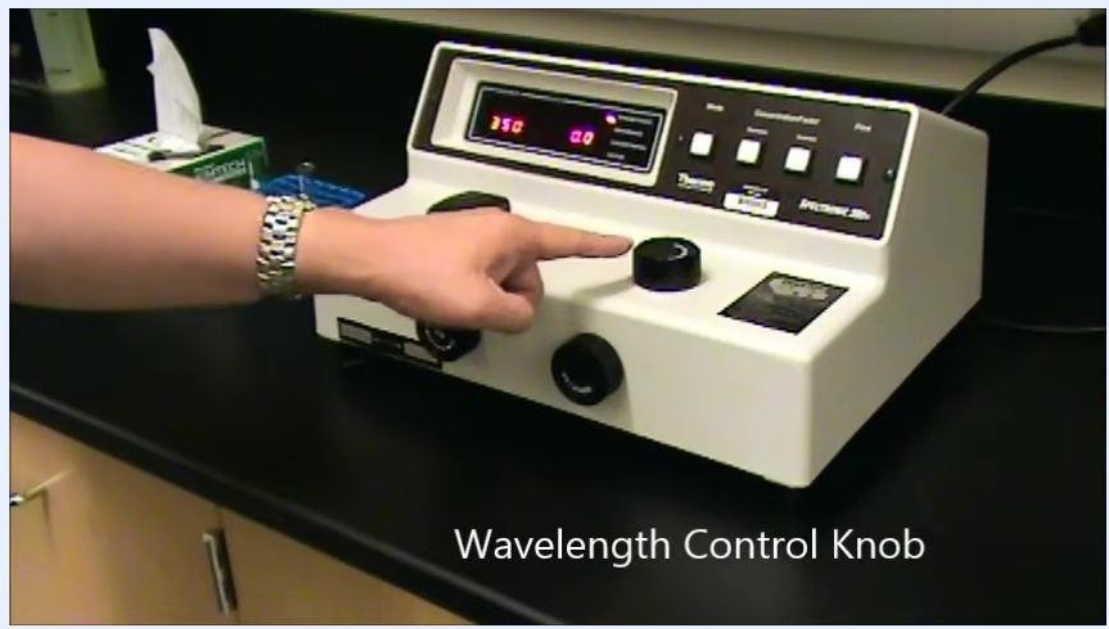
A hand points to the Wavelength Control Knob on the spectrophotometer
