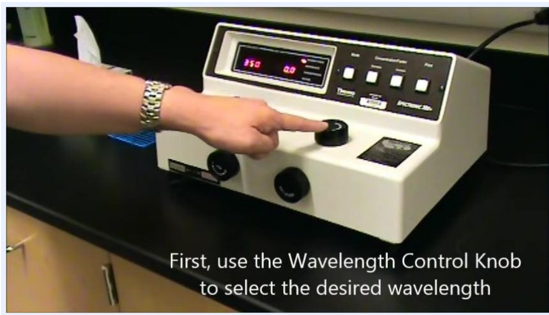
Hand adjusting the Wavelength Control Knob while the display shows 350 nm and 0.0
