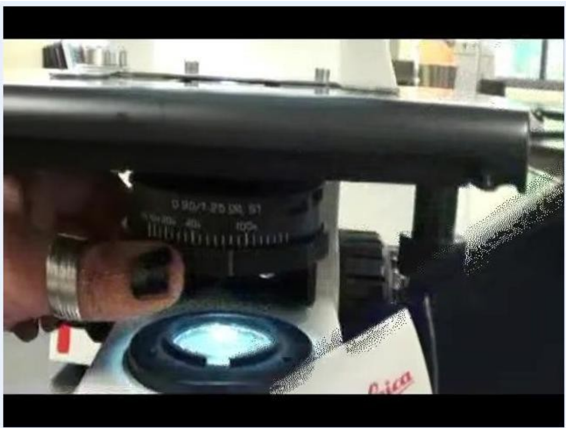
Close-up of the microscope base showing the illuminated light source labeled "Illuminator in base," with a hand near the power switch.
