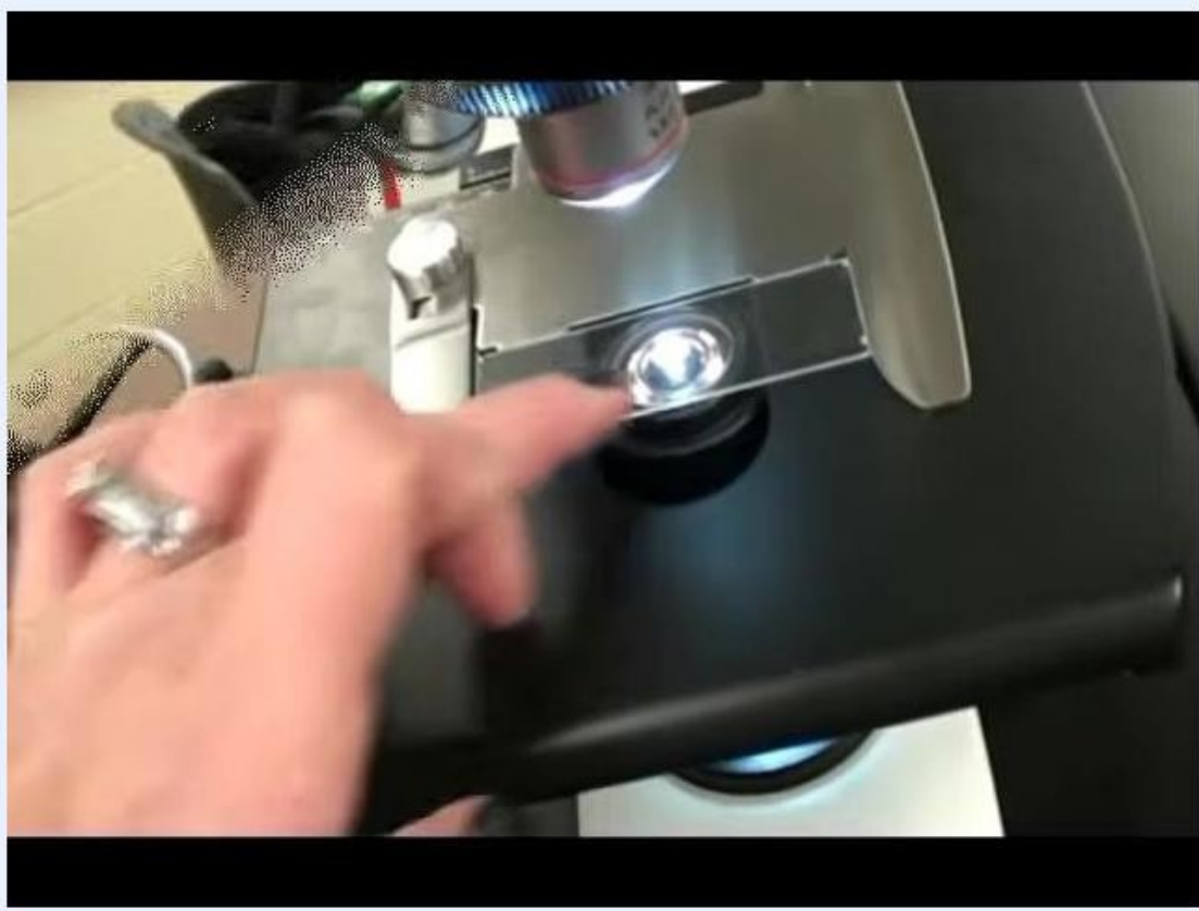
Hand operating the coaxial adjustment knobs on the side of the stage to move and center the slide.
