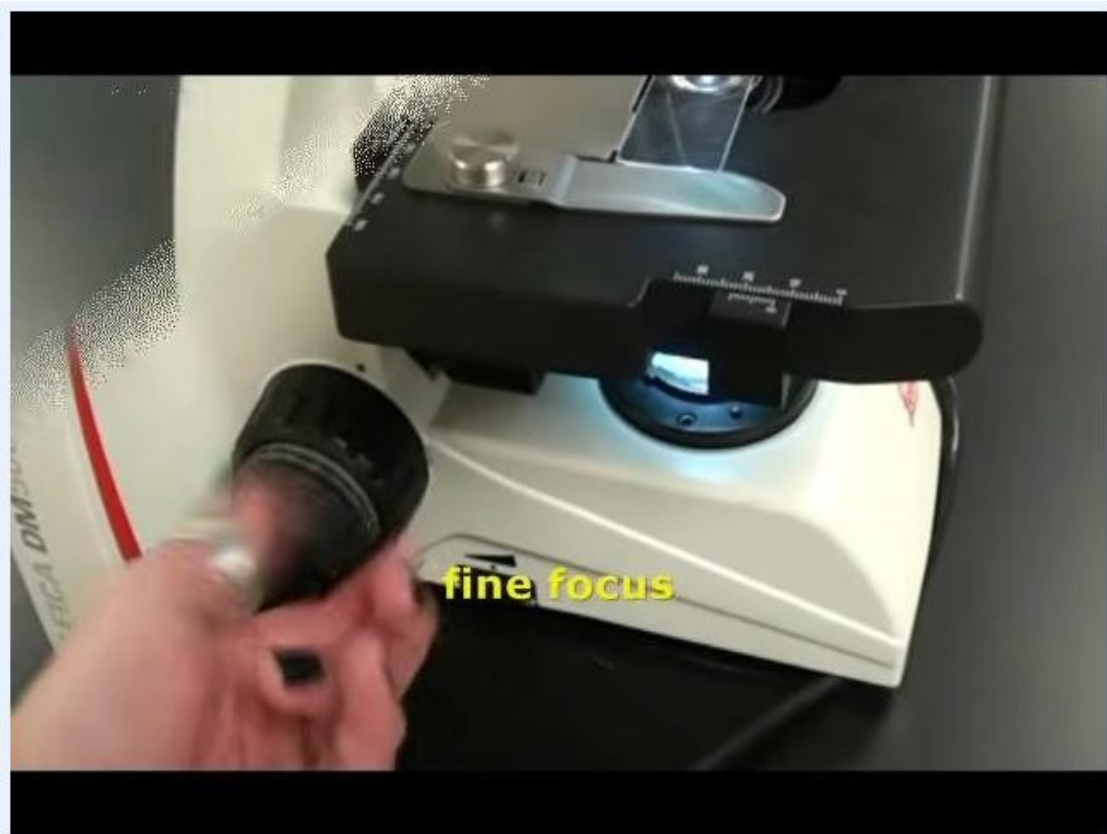
Hand adjusting the fine focus knob on the side of the microscope, with the label "fine focus" visible and the stage and slide illuminated.
