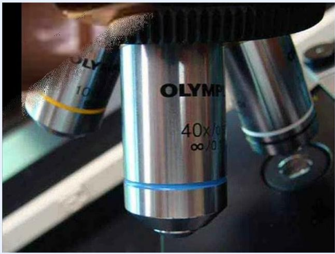
Close-up of microscope nosepiece with the 40x objective (blue band) centered, showing how close it is to the stage.
