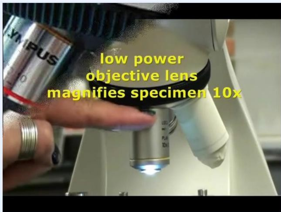
Hand pointing to the low power objective lens with a yellow band, labeled "low power objective lens magnifies specimen 10x".
