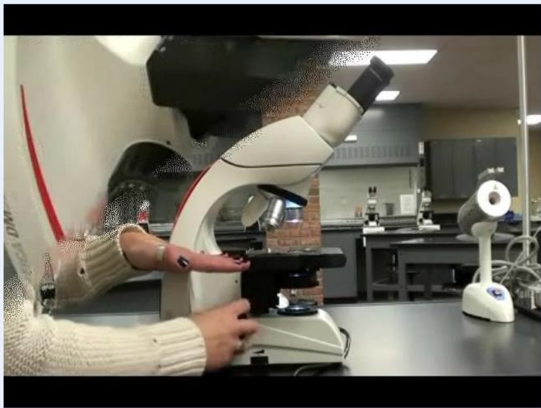
Person demonstrating the use of both coarse and fine focus knobs on the microscope, with hands positioned on the adjustment controls.
