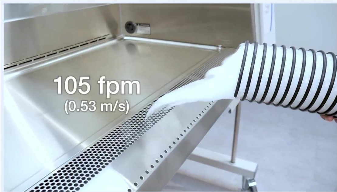
A gloved hand directs vapor across the work surface, demonstrating the smoke split airflow pattern.
