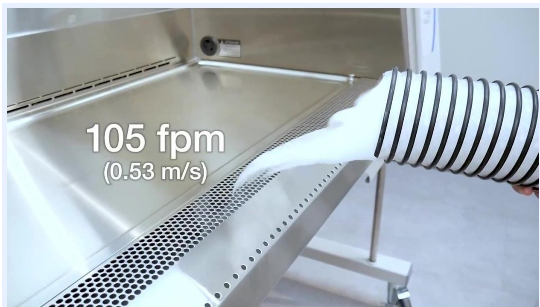
A gloved hand uses an airflow visualizer to release visible vapor, demonstrating airflow patterns above the front grille.
