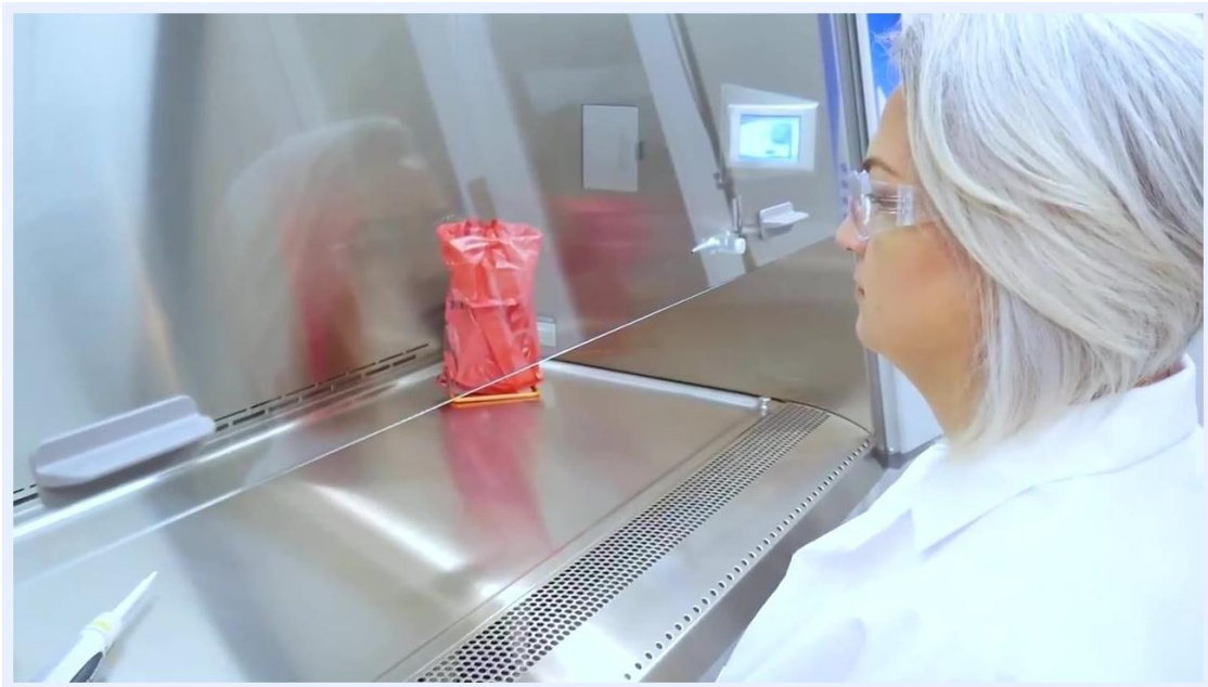
A worker sits in front of the cabinet, gloved and ready to begin entering the work area slowly.
