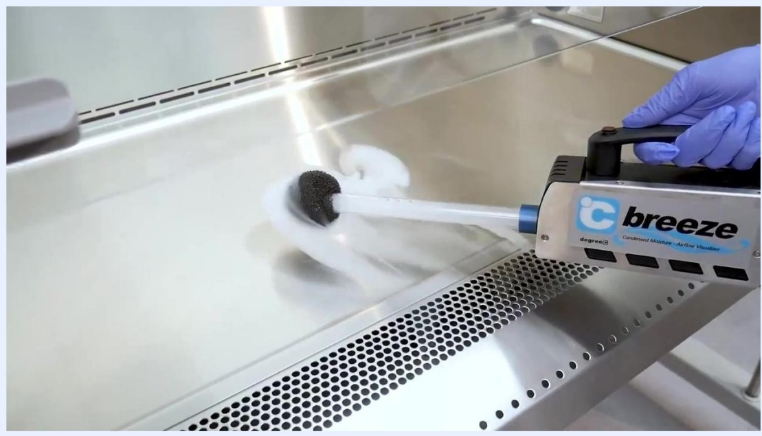
A gloved hand uses an airflow visualizer to release visible vapor, demonstrating airflow patterns above the front grille.
