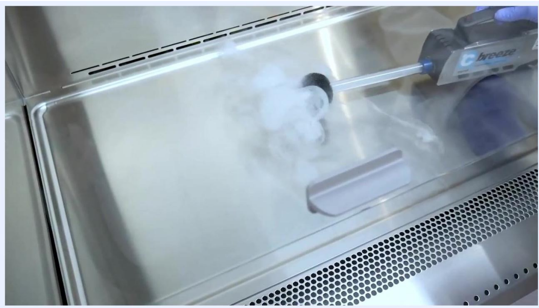
A gloved hand uses an airflow visualizer inside the cabinet to check for leaks and confirm proper airflow.
