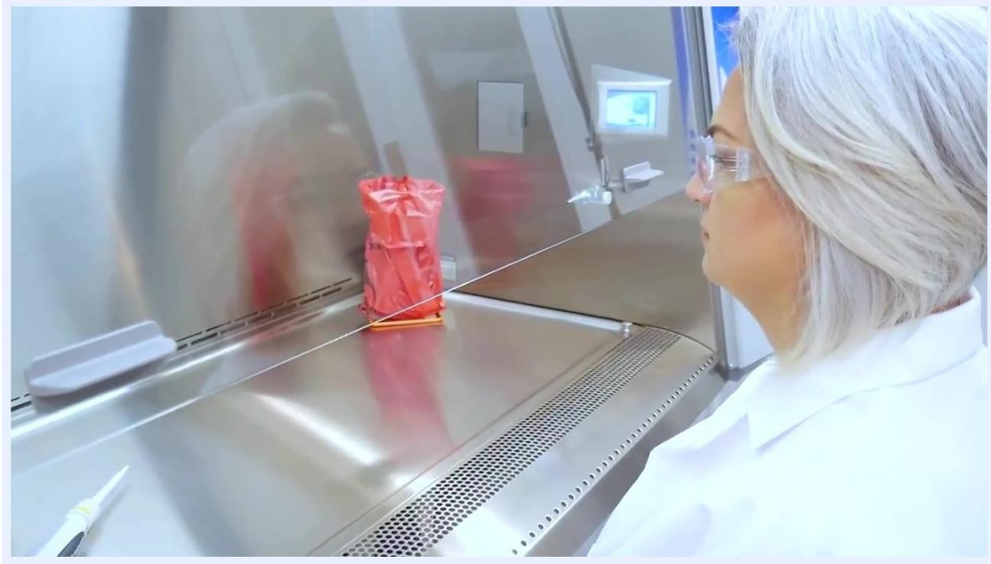
A worker sits at the cabinet with her nose and mouth positioned above the front grille.
