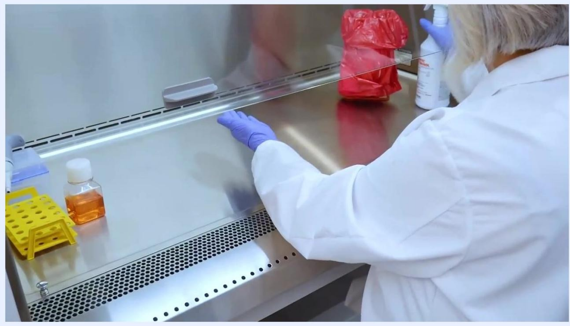
A worker uses a wipe and disinfectant spray to clean the exterior of lab materials before removing them from the cabinet.
