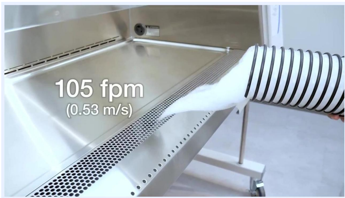
Vapor released at the front grille with an overlay reading "105 fpm (0.53 m/s)," indicating inflow air velocity.
