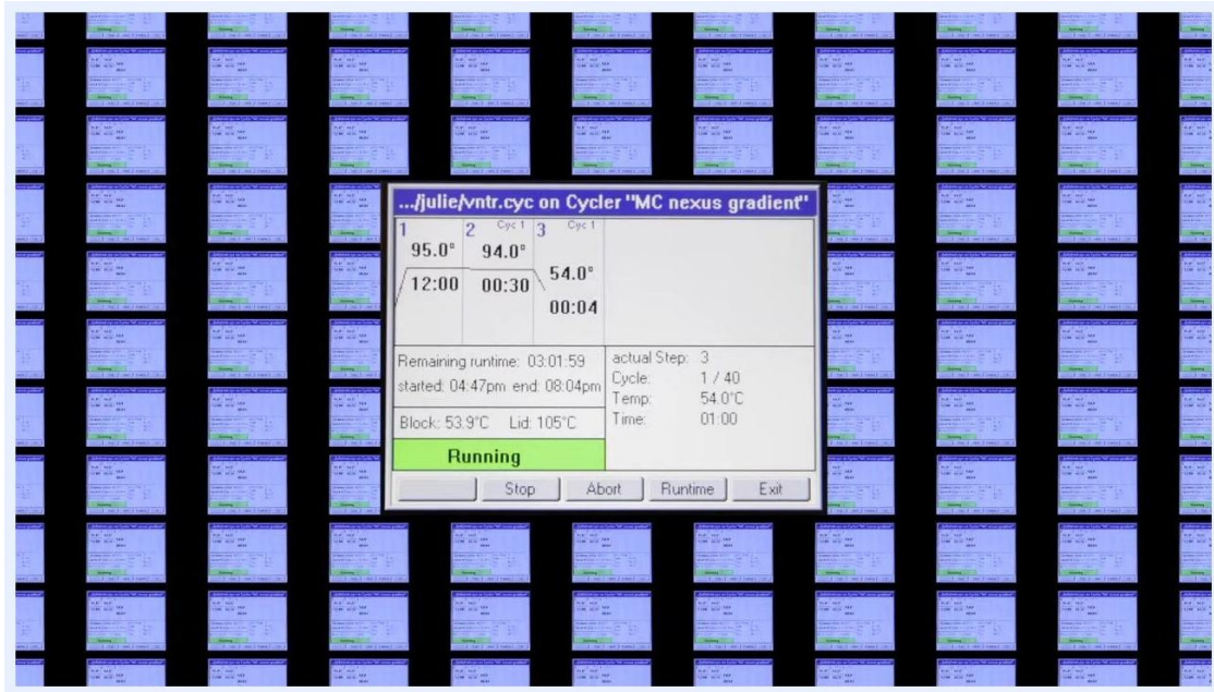
Thermal cycler display showing PCR program steps: 95.0°C for 12:00, 94.0°C for 0:30, 54.0°C for 1:00, 72.0°C for 2:00, with cycle count and status "Running".
