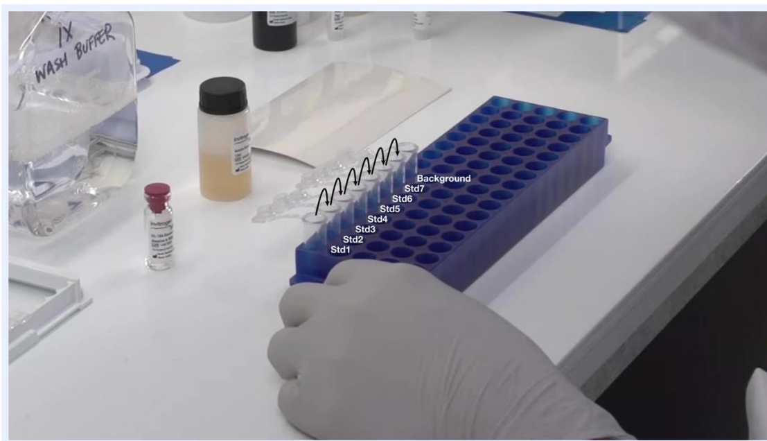
Gloved hand holding a blue rack of labeled tubes (Std1–Std7, Background) while pipetting into strip tubes, with the 1X Wash Buffer bottle and ELISA plate on the bench.
