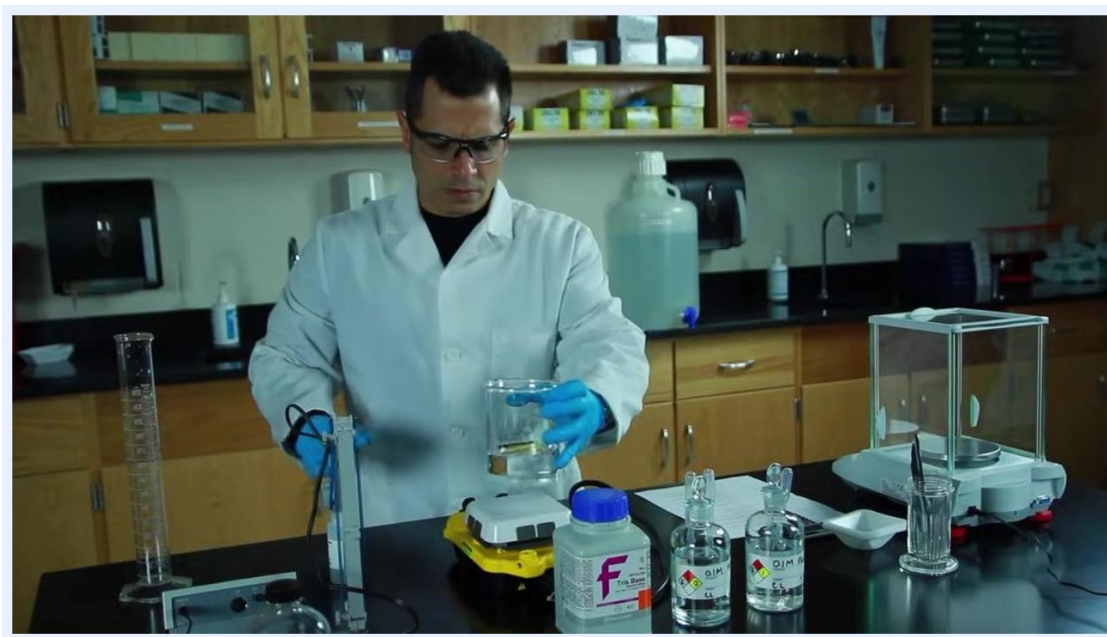
Placing a beaker containing water and a stir bar onto a yellow stir plate
