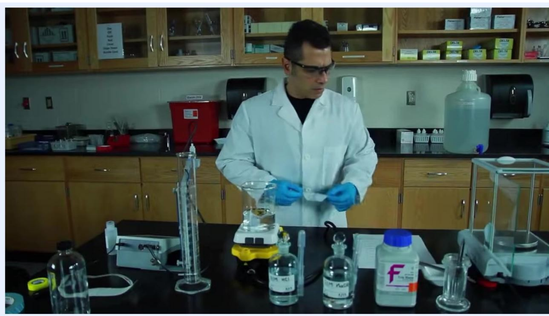
A lab-coated technician using a pH meter probe in the beaker on the stir plate, with acid and base bottles nearby
