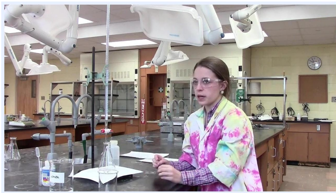
Person monitoring the titration process, with the flask on white paper and the burette dispensing solution.
