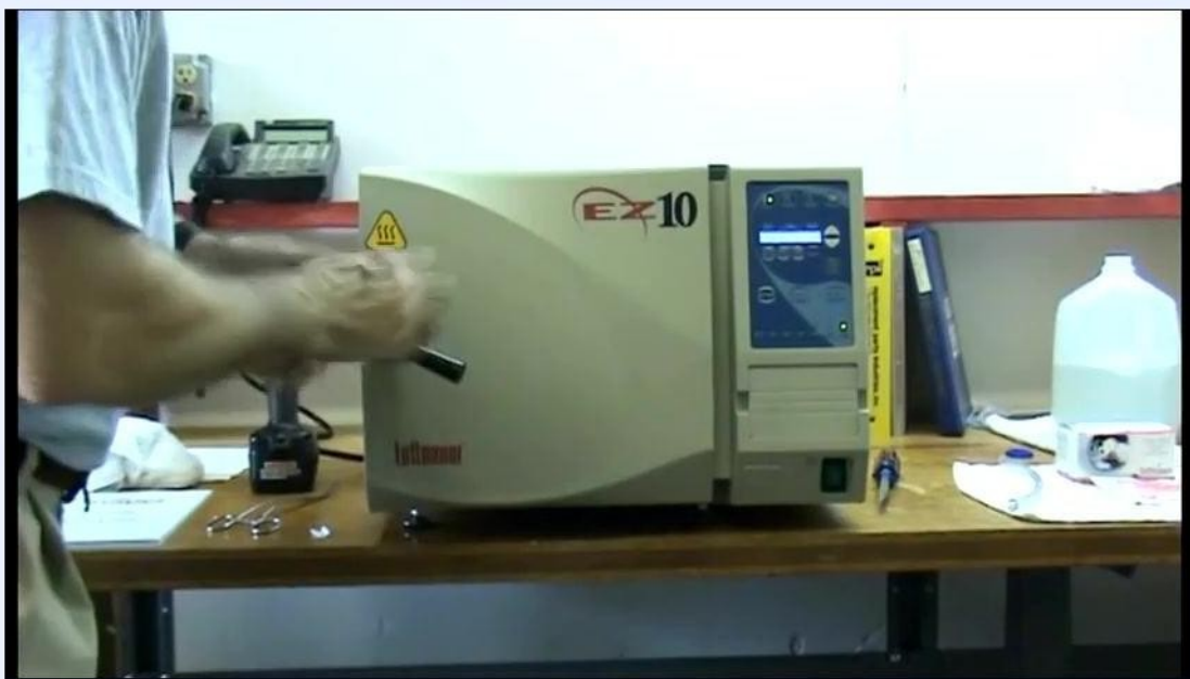
A person turning the handle to lock the autoclave door, with the control panel illuminated.
