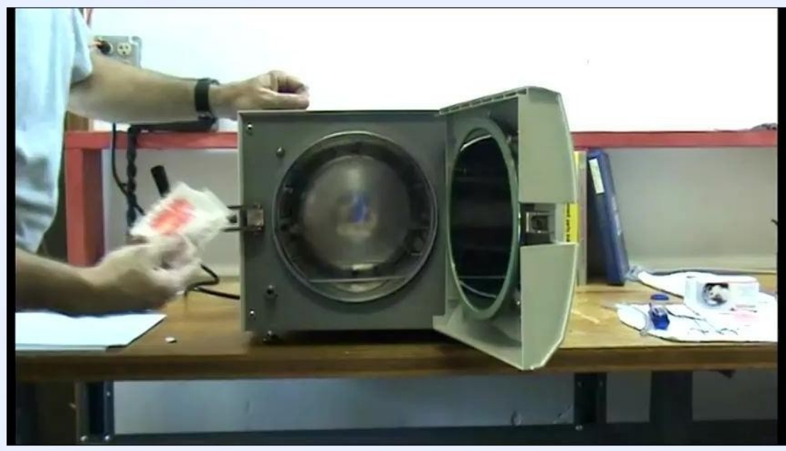
The chamber open with the operator holding a Chamber Brite packet, preparing to pour it in.
