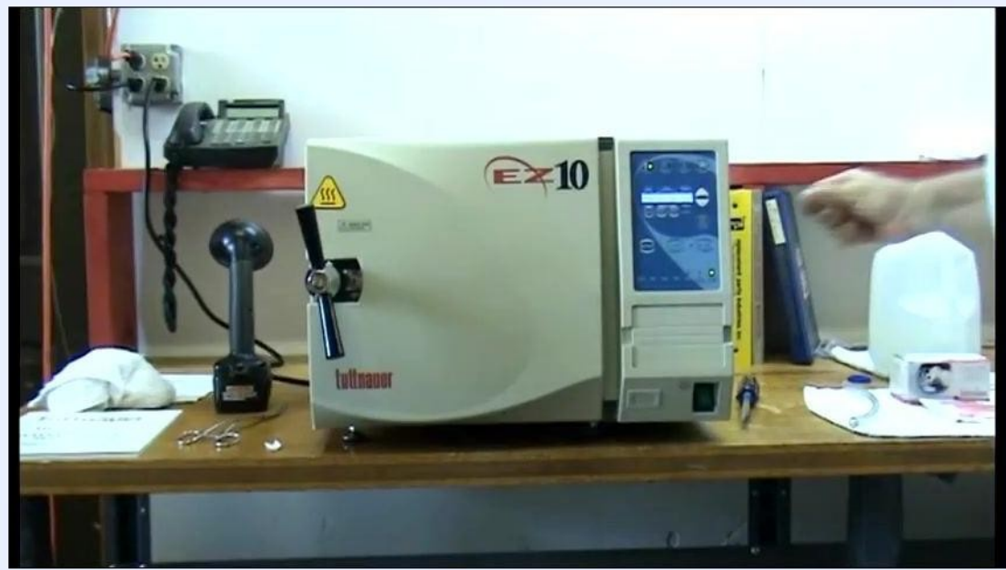
The autoclave door locked, control panel active, and a hand positioned near the panel.
