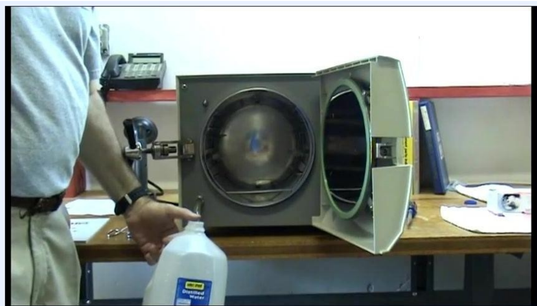
The operator holding the collection container as the solution drains from the reservoir.
