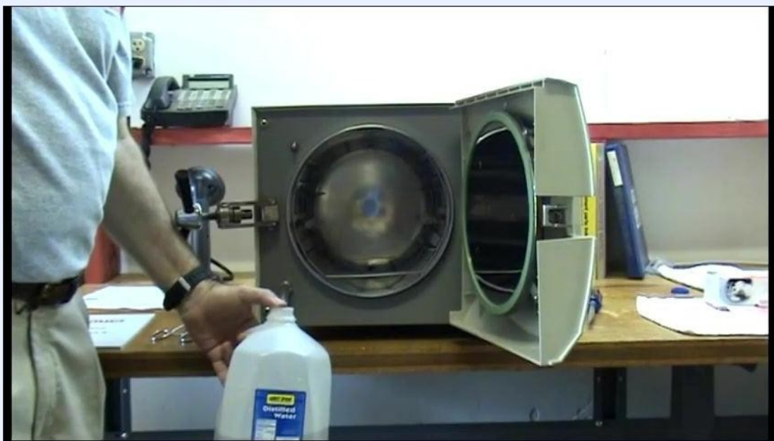
The operator holding a labeled distilled water jug near the open autoclave chamber, preparing to refill the reservoir, with tools and paperwork nearby on the workbench.
