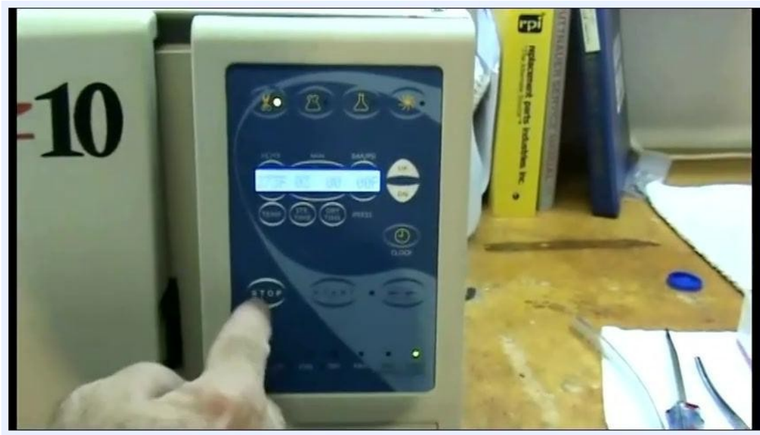
The operator's finger on the control panel selecting the appropriate cycle, with the display and buttons visible.
