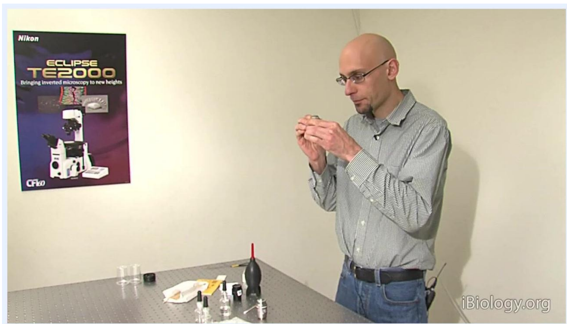
A person holds a blower, explaining its use for removing loose dust from microscope objectives, with cleaning supplies and objectives visible on the table.
