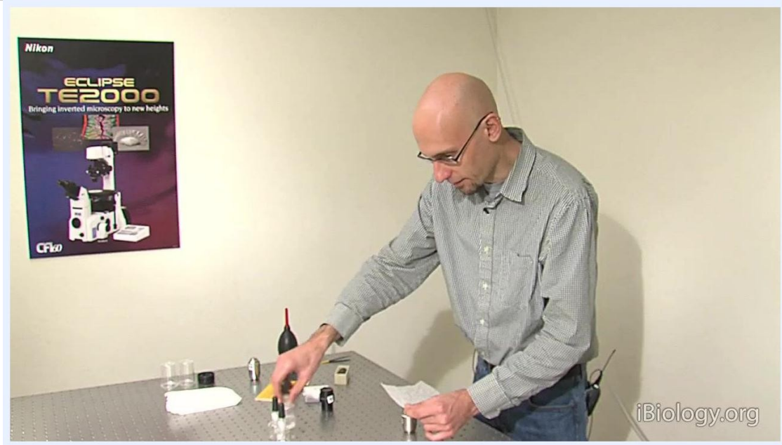
A person applies a drop of solvent to a microscope objective on a laboratory table, with cleaning supplies and lens paper visible.
