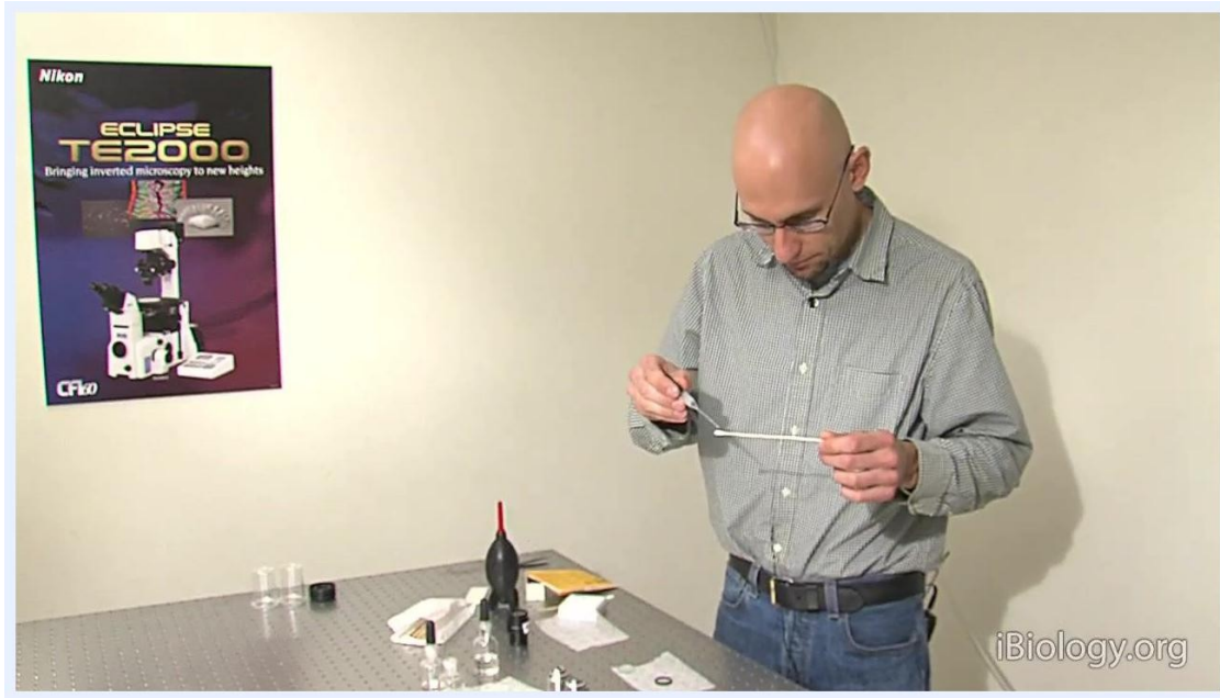
A person stands at the workstation, holding a cotton swab and preparing to moisten it with solvent, with cleaning supplies, lens paper, filters, and a Nikon ECLIPSE TE2000 poster visible.
