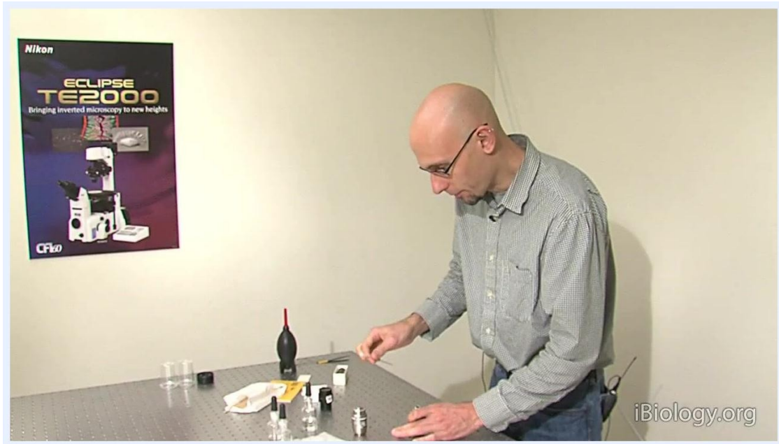
A person uses a cotton swab to clean a microscope objective, preparing to repeat the process with methanol, with cleaning supplies and objectives visible on the table.
