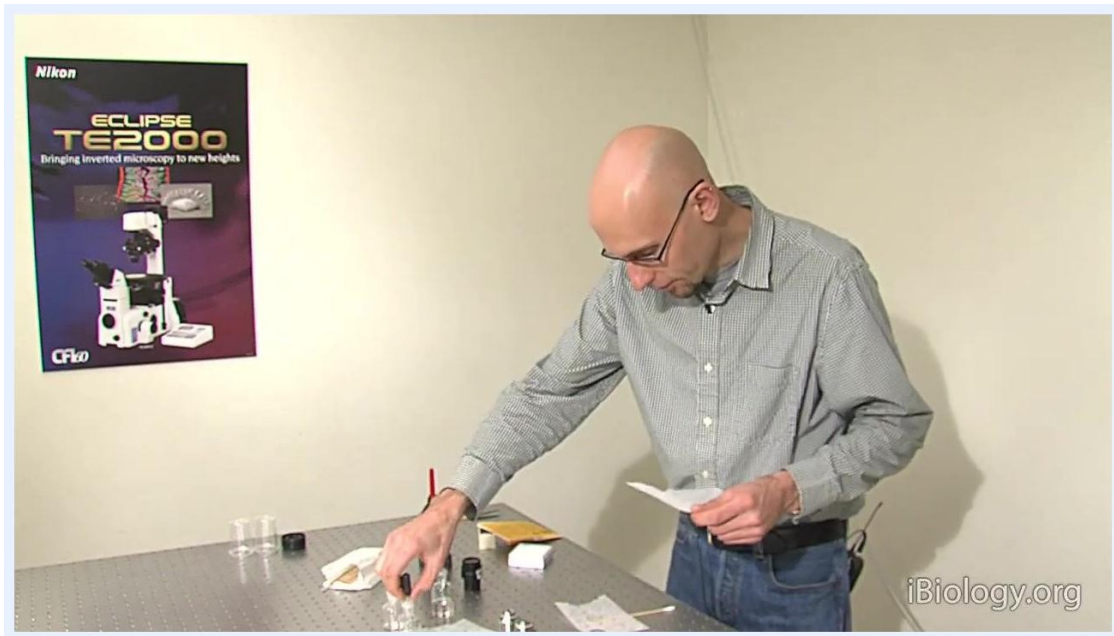
A person applies solvent to an unmounted filter and prepares to use the drag mopping technique with lens paper.
