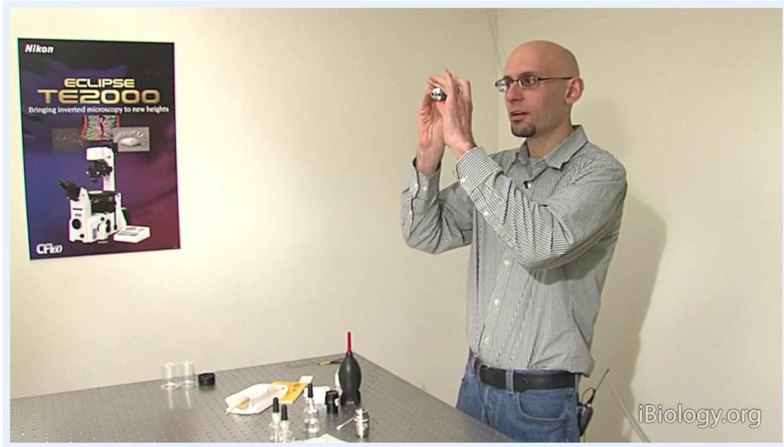
A person uses a blower to clean a microscope objective on the table, with cleaning supplies and objectives visible.
