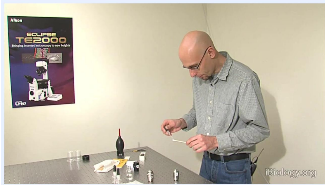
A person wets a cotton swab with solvent, preparing to clean a microscope objective, with cleaning supplies and a Nikon ECLIPSE TE2000 poster visible.
