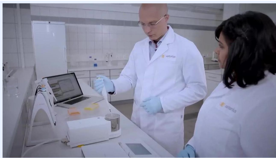
A technician dispensing liquid with a pipette into a vessel on a balance, focusing on precision and repeatability
