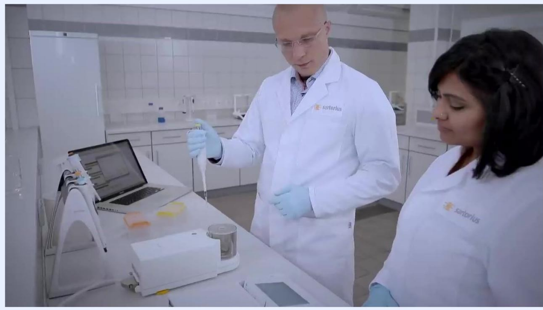
A technician holding a pipette vertically and at a 45-degree angle, demonstrating correct pipetting technique during calibration
