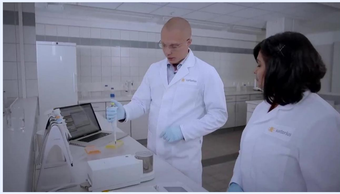
A laboratory technician in a white lab coat and blue gloves dispensing liquid from a pipette into a vessel on a balance, with another technician observing.
