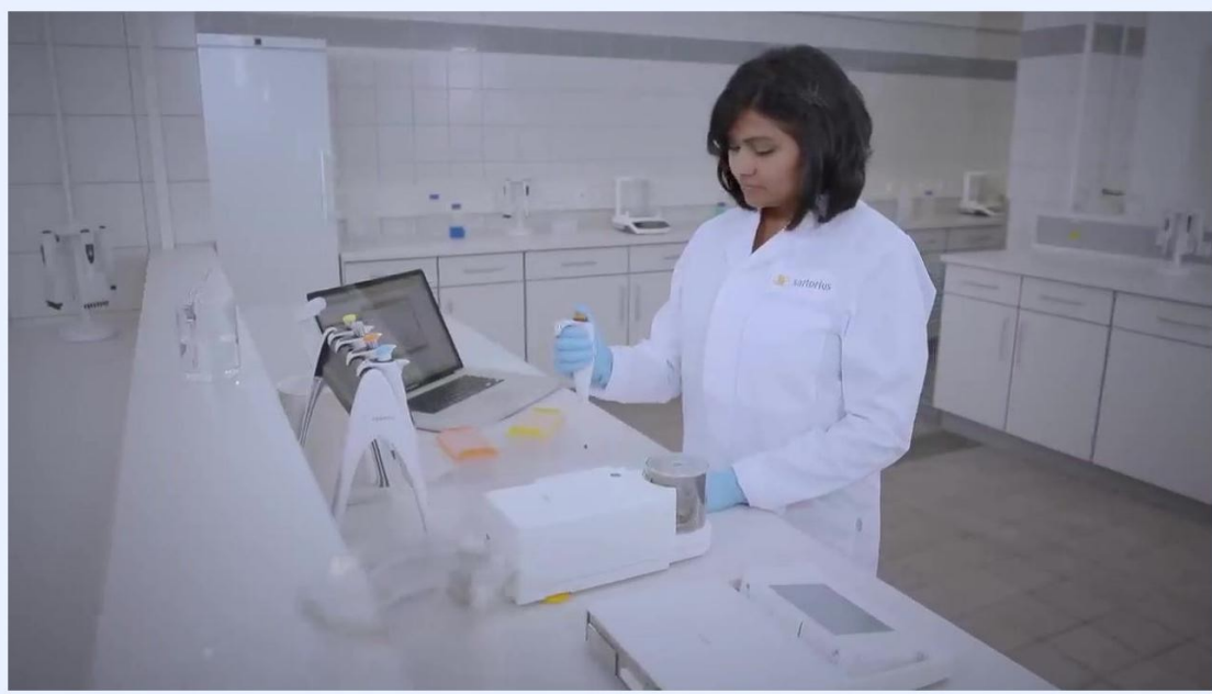
A laboratory technician in a white lab coat and blue gloves pre-wetting a pipette tip at a calibration station. The workspace includes a balance, pipette stand, disposable tip boxes, and a laptop.
