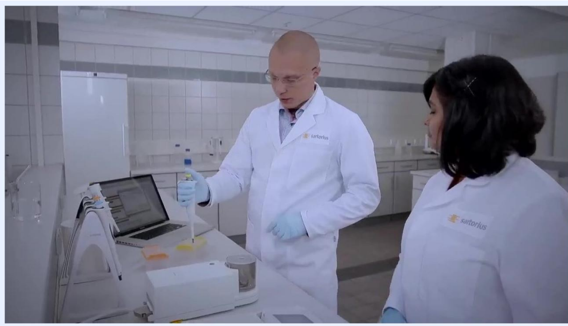
Close-up of a gloved hand dispensing liquid from a pipette into a small vessel inside a balance enclosure. The balance and other calibration equipment are visible.
