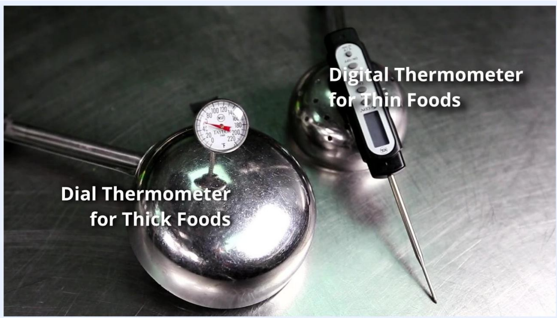
Dial thermometer and digital thermometer laid out on metal surfaces, showing which tool to use for thick foods and which for thin foods.
