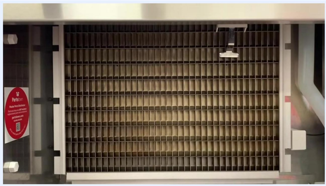
View of the evaporator grid inside the ice machine, shown empty and ready for inspection
