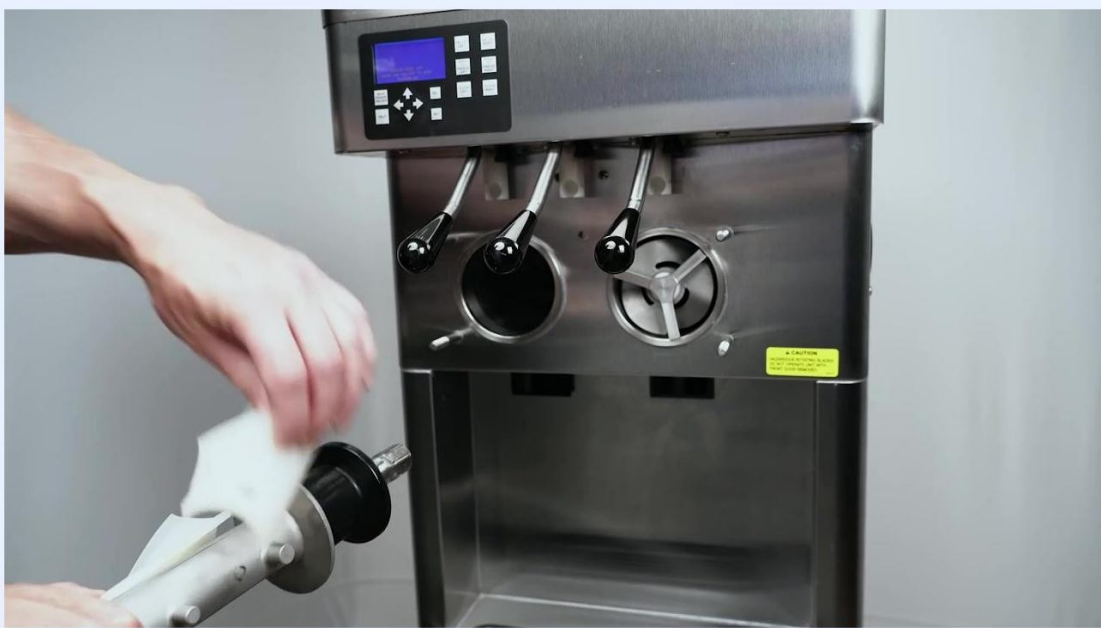
A close-up of the hex drive end of an auger shaft, partially inserted into a black rear seal. The hex end is coated with a small amount of clear lubricant. A hand is visible in the foreground.
