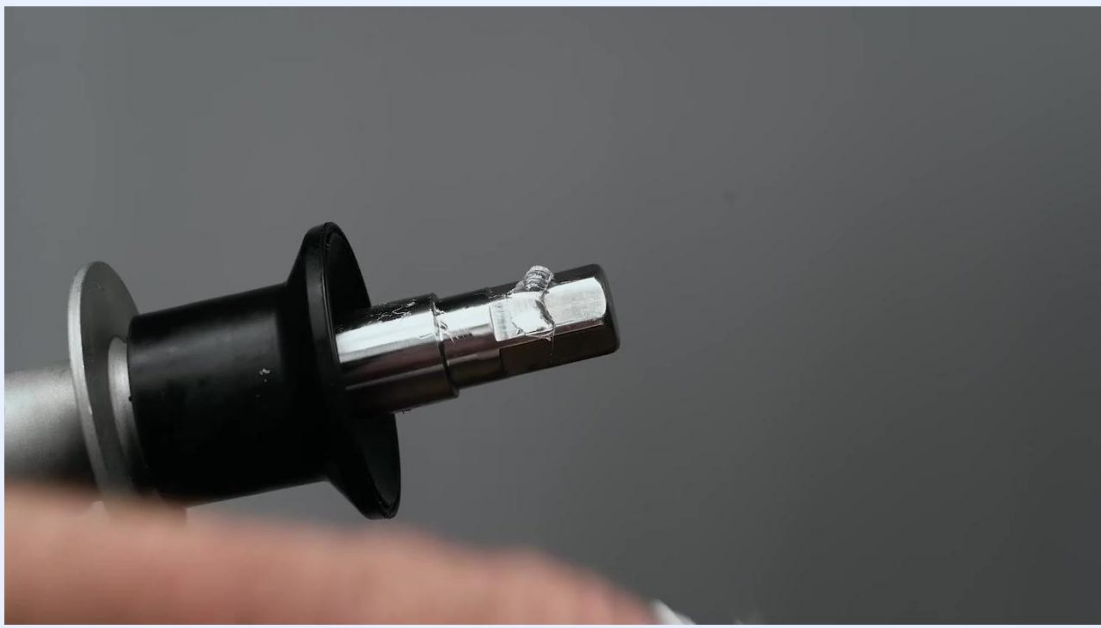
A close-up of a stainless steel auger shaft with a black rear seal installed. The seal and the shaft are coated with a visible layer of clear lubricant. The background is neutral gray, and a hand is partially visible holding the shaft.
