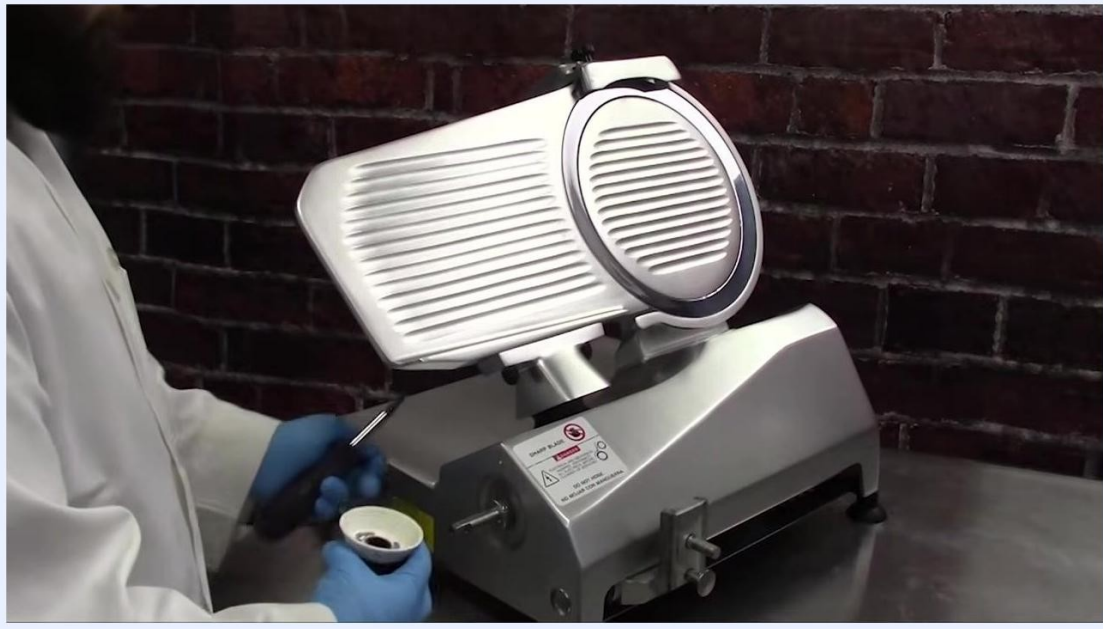
Close-up of a gloved hand loosening and removing the black thickness control dial, marked with numbers 0–9.
