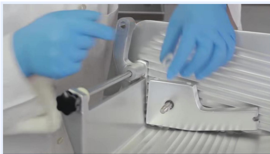
Operator positioning the thin plastic spacing washer onto the feed grip rod, ensuring proper placement.
