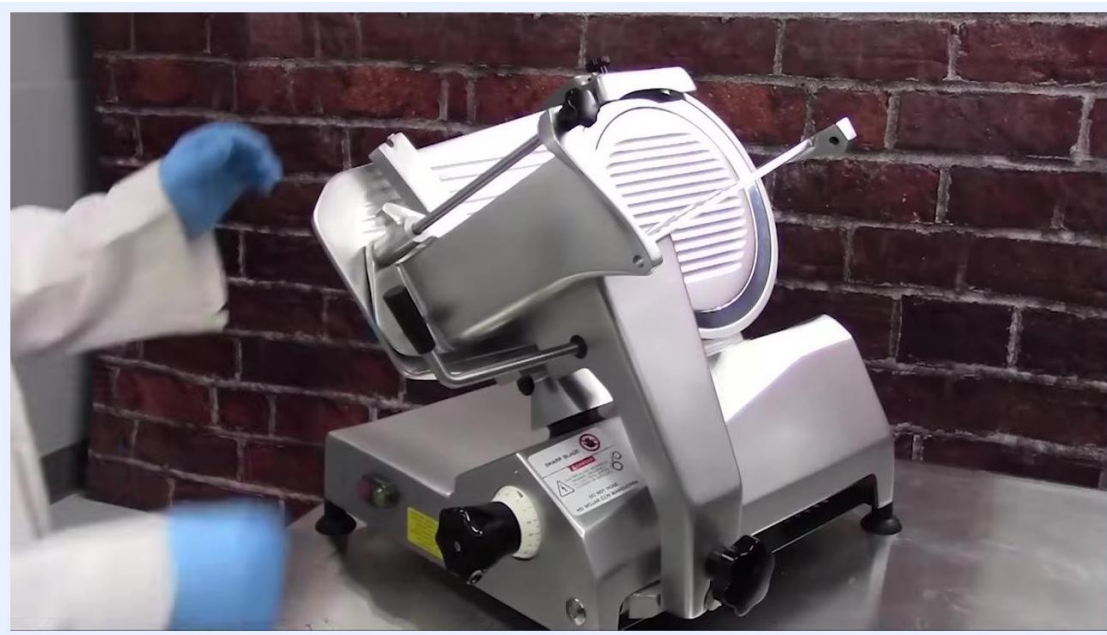
Slicer with the feed grip being removed; operator's gloved hands visible.
