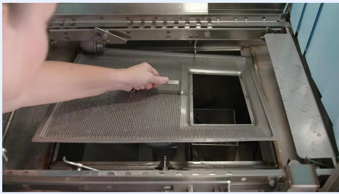
Hand lifting the strainer pan out of the wash tank
