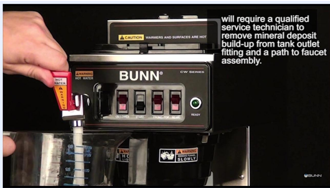
A front view of the BUNN CW Series coffee brewer shows the red faucet handle attached, ready for the handle and bonnet nut assembly to be removed.
