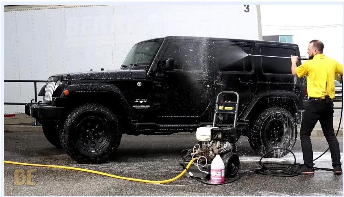
Person in a yellow shirt moving the soap injector hose from the soap solution bucket to a clean bucket of water, both buckets visible next to the BE Power Washer
