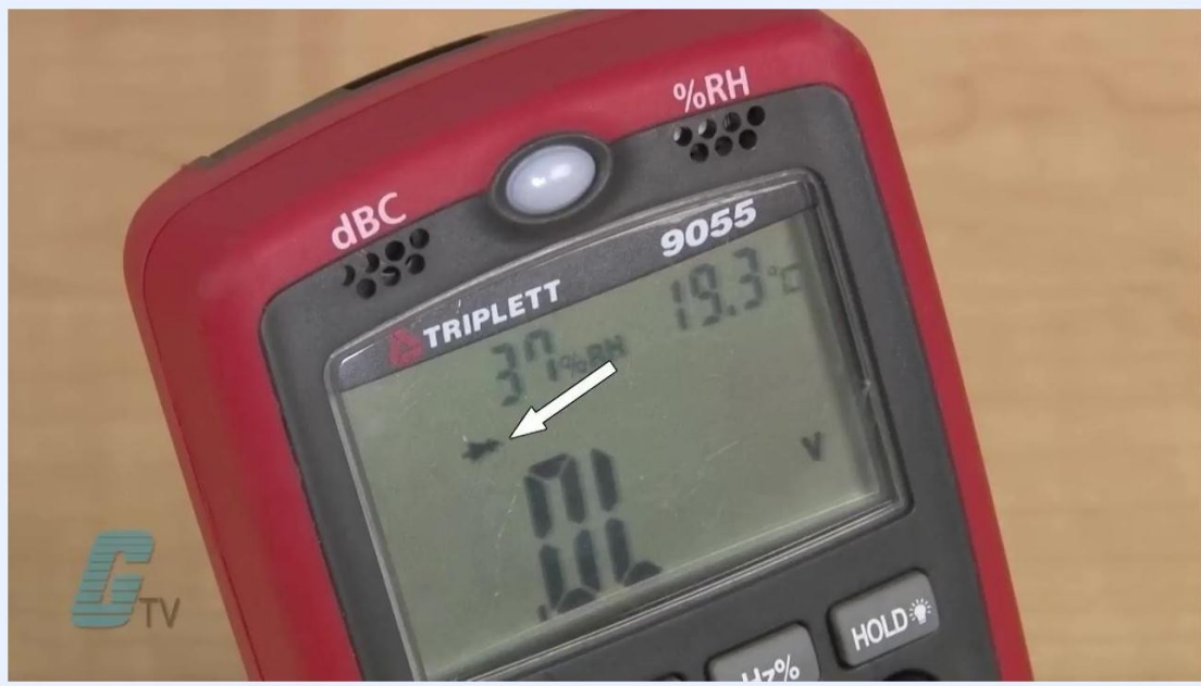
Close-up of a TRIPLETT 9055 digital multimeter display showing the "OL" reading, the radio wave symbol, and an arrow pointing to a specific icon.
