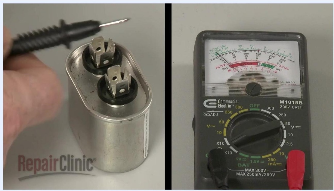
Split image: a hand holding a probe near the capacitor terminals on the left, and the ohm meter showing needle deflection on the right
