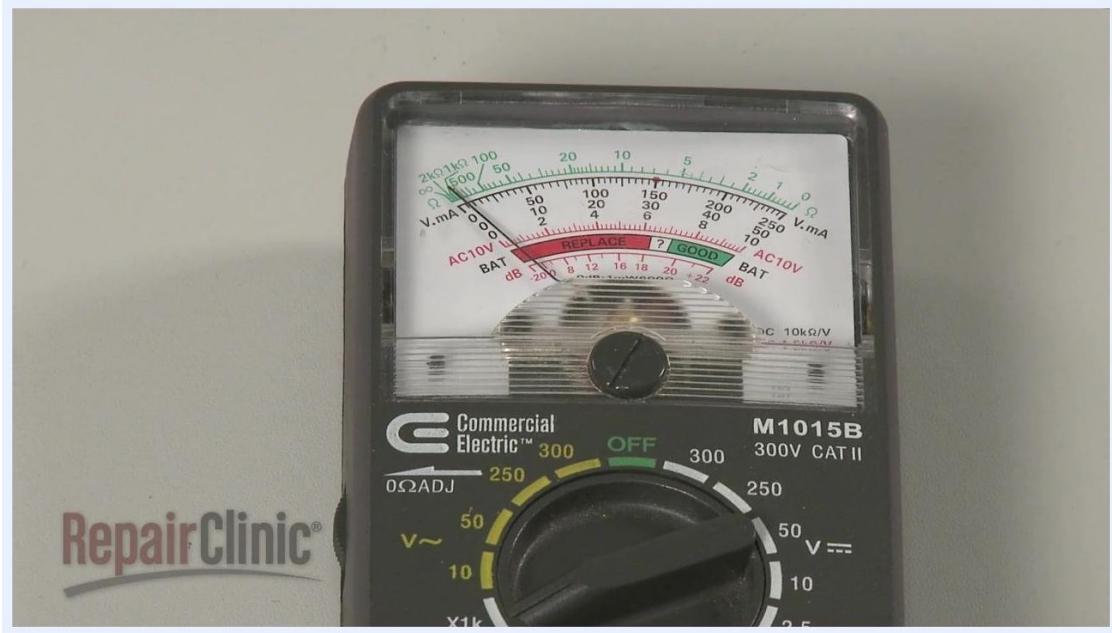
Analog ohm meter showing needle movement during a dual capacitor test
