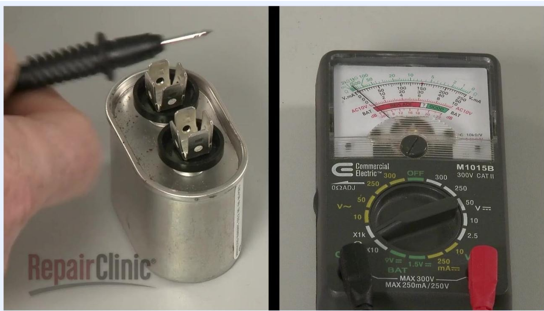
Close-up of dual capacitor terminals, clearly labeled "C" and "FAN"
