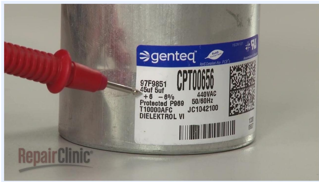
Close-up of a dual capacitor label showing "45uf 5uf" ratings, with a probe pointing at the values
