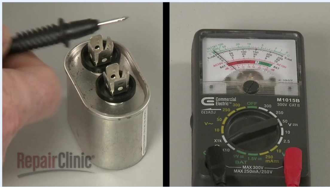
Analog ohm meter with the needle at zero, indicating a failed capacitor
