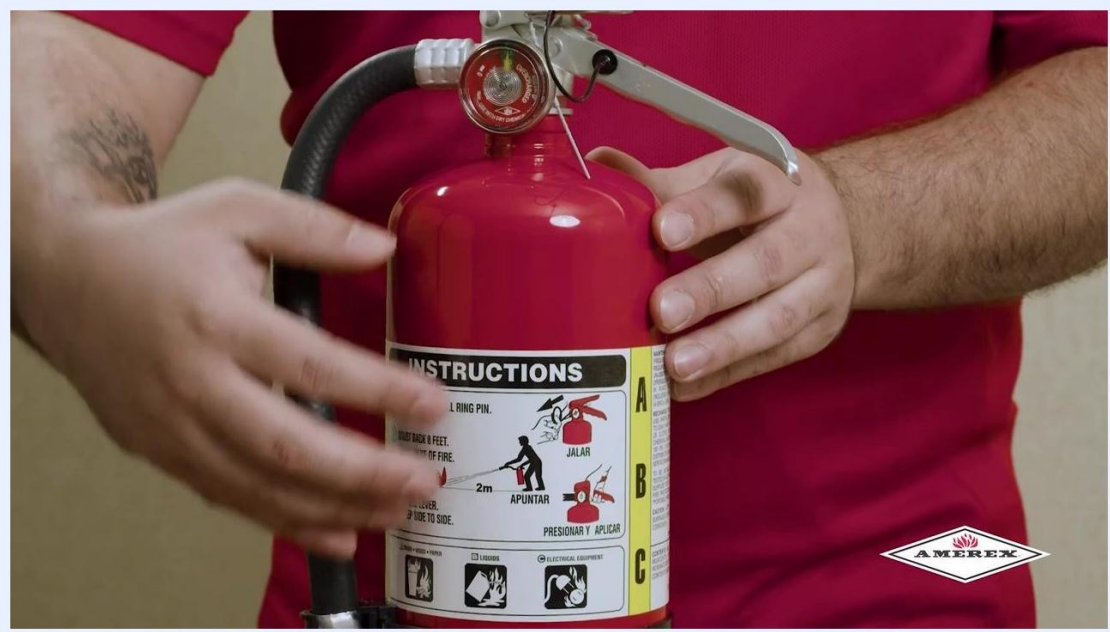
Close-up of hands squeezing the extinguisher's handle and lever to check for freedom of movement.
